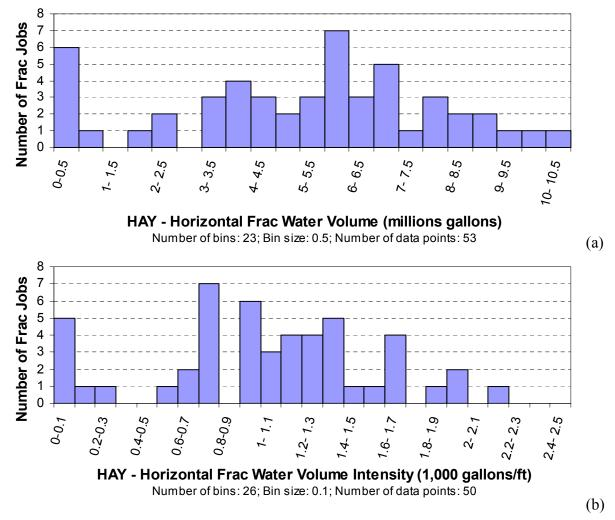
Figure 37. Haynesville—horizontal well frac water use: (a) total volume; (b) intensity in 1,000 gal/ft (2008 and beyond)
