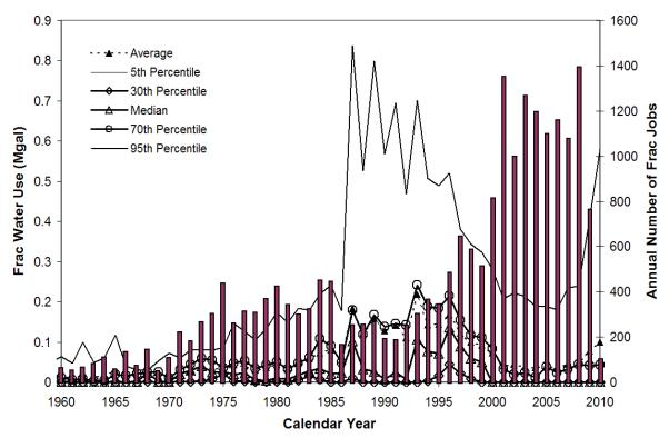
Note: curves and columns represent water use (LHS y-axis) and number of jobs (RHS y-axis), respectively
