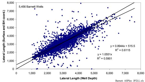
Note: equation for best fit and fit through the origin are shown. Only those points for which both values are available are shown. Plot also provides estimate of typical and maximum lateral length.
