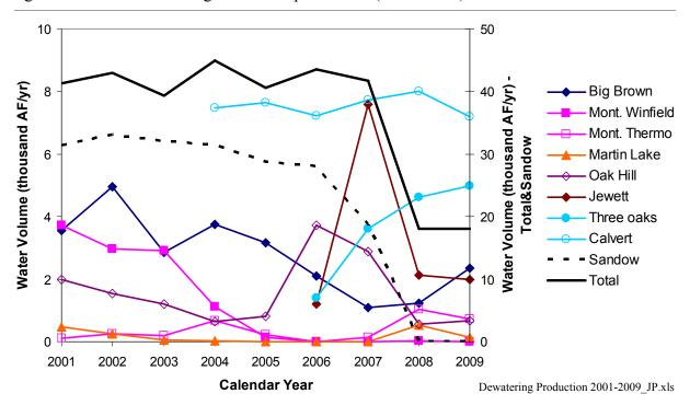
Note: all mines described by LHS y-axis except Sandow and Total represented by RHS y-axis Figure 99. Lignite mine groundwater production 2001–2009
