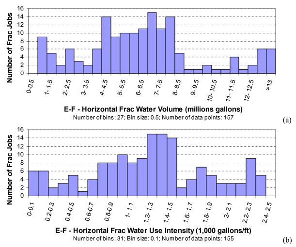
Figure 44. Eagle Ford—horizontal well frac water use: (a) total volume; (b) intensity in 1,000 gal/ft (2008 and beyond)
