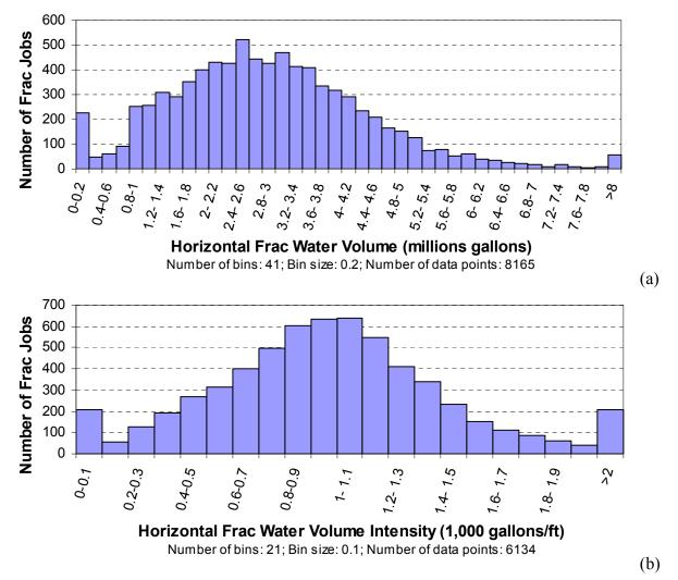
Figure 31. Barnett Shale-frac water use: (a) total volume, (b) intensity in 1,000 gal/ft
