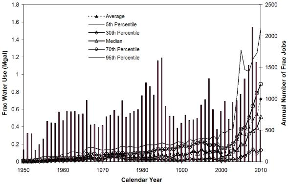
Note: curves and columns represent water use (LHS y-axis) and number of jobs (RHS y-axis), respectively Figure 68. Permian Basin—annual number of frac jobs superimposed on annual average, median, and other percentiles of individual well frac water use (all 50,000+ wells).
