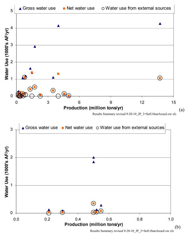
Figure 105. Water use from BEG survey for (a) crushed stone facilities; (b) sand and gravel facilities
