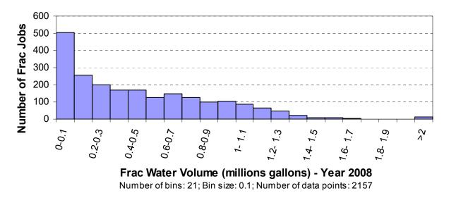
Figure 71. Permian Basin-frac water use in vertical wells
