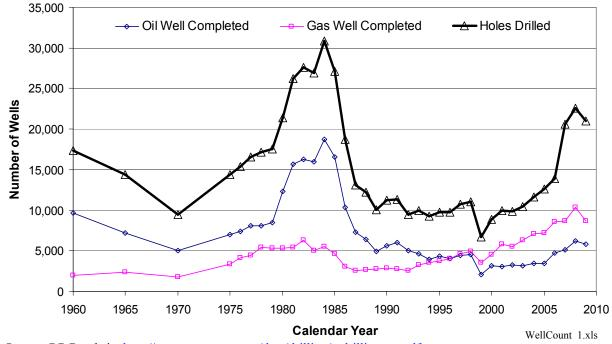
Source: RRC website <u>http://www.rrc.state.tx.us/data/drilling/txdrillingstat.pdf</u> Note: completions include mostly new drills but also re-entered and recompleted wells (10-15% of total) Figure 95. Number of holes drilled and of oil and gas wells completed in Texas between 1960 and 2009
