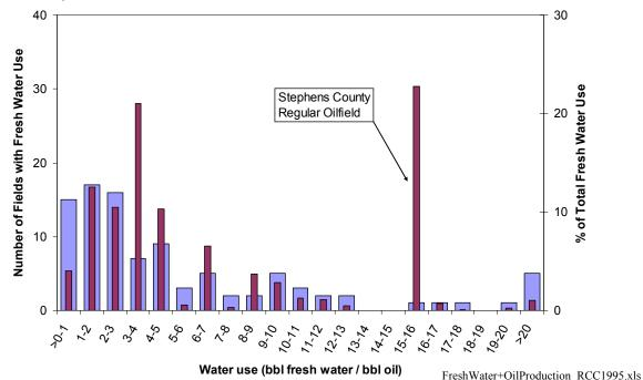
Note: broad and narrow columns represent # of fields (LHS y-axis) and % water use (RHS y-axis), respectively Figure 85. Histogram (year 1995) of water-use coefficient in waterflooded oil fields (wide columns) and fraction of total fresh-water use for each bin
