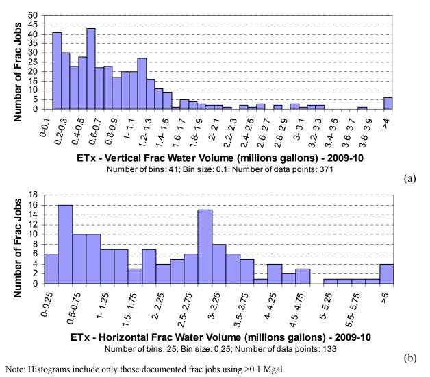
Figure 62. East Texas Basin—frac water use in vertical wells (a) and horizontal wells (b)
