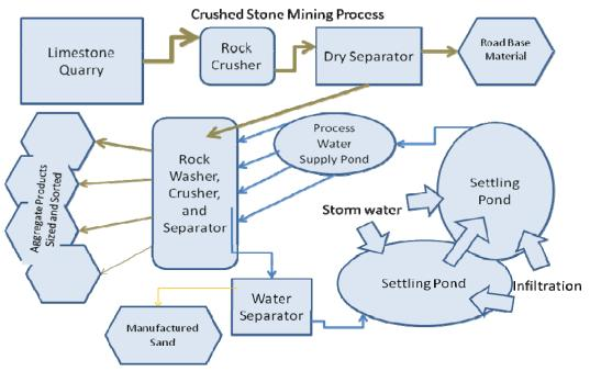
Figure 102. Flow diagram of typical crushed-stone process
