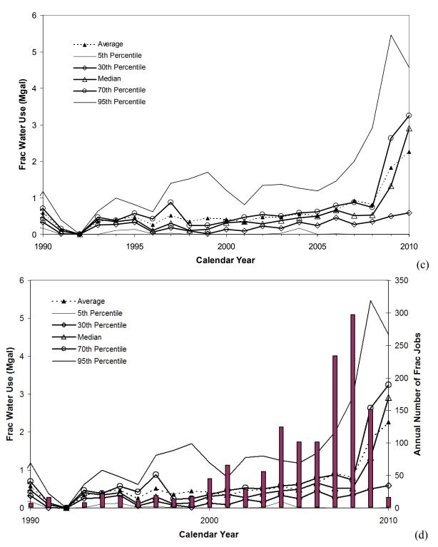
Figure 61. East Texas Basin—annual number of frac jobs (b and d) superimposed on annual average, median, and other percentiles of individual well frac water use (a and c) for 1950– ~2008 (a and b) and 1990–~2008 (c and d) periods (continued).
