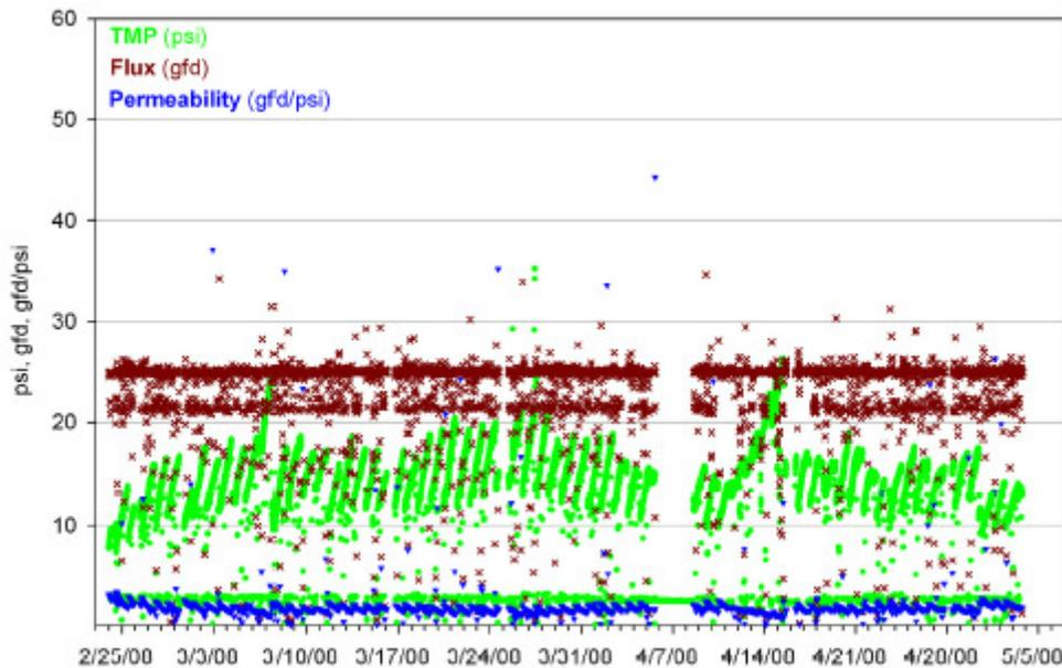
**Figure 9:** Operation at 25 gfd (TCEQ Stage 2), Pall MF membrane performance
