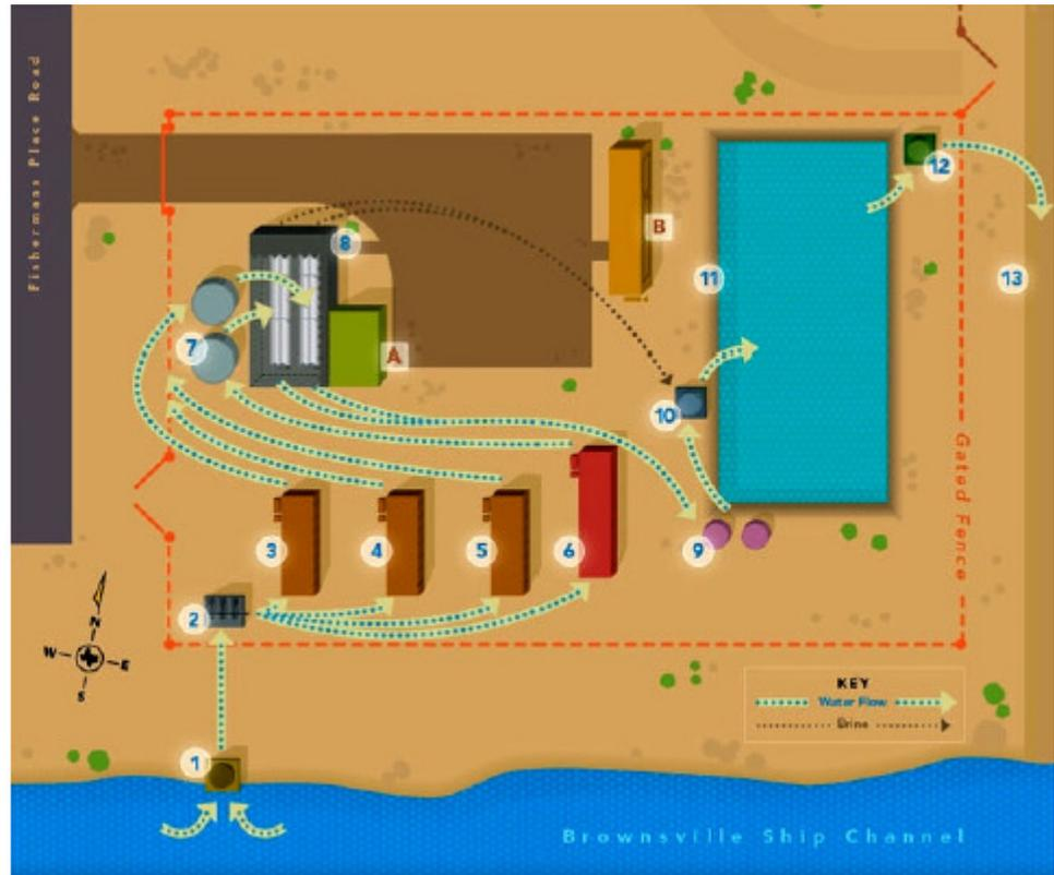
**Figure 7:** Layout of the Brownsville Seawater Desalination Pilot Project
