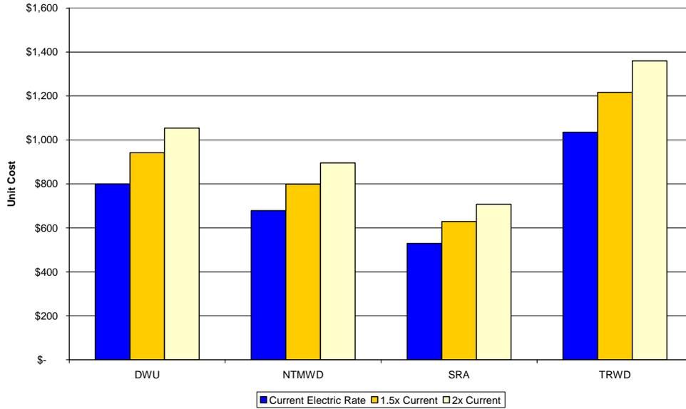
**Figure 2.12** Impacts of Electric Rates on Unit Cost by User During Amortization
