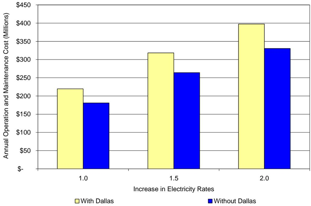
**Figure 2.10** Comparison of Annual Cost for Different Electric Rates
