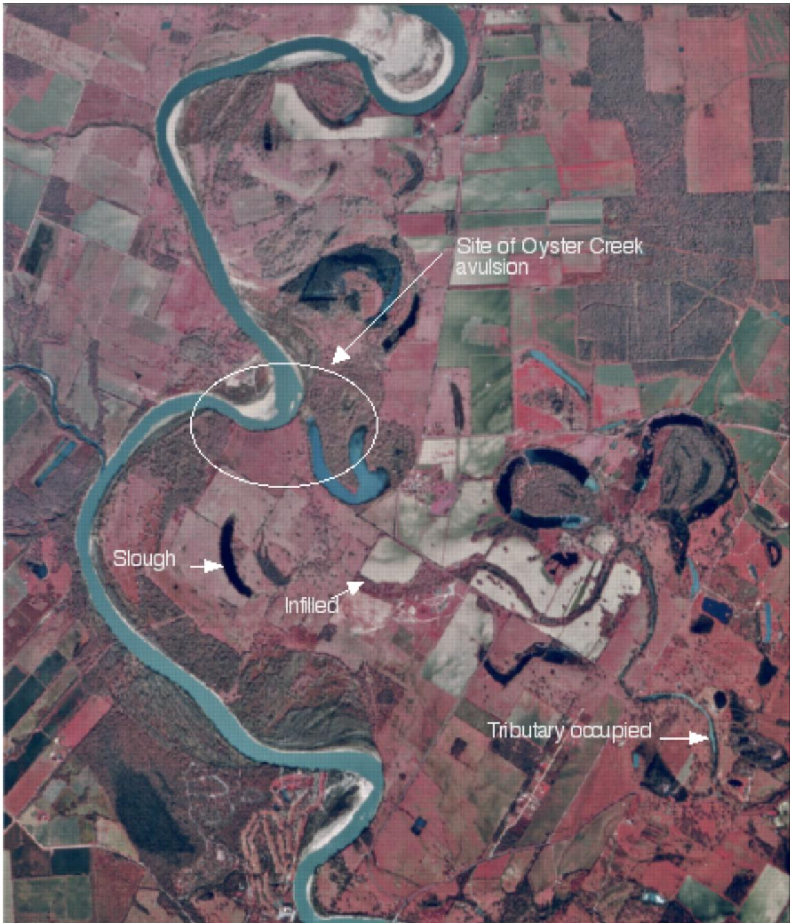
Figure 4. Site of the Oyster Creek avulsion of the Brazos River near San Felipe, TX. Portions of the Brazos paleochannel in various stages of development are shown. A Number of cutoffs are also visible in this false-color DOQQ image.
