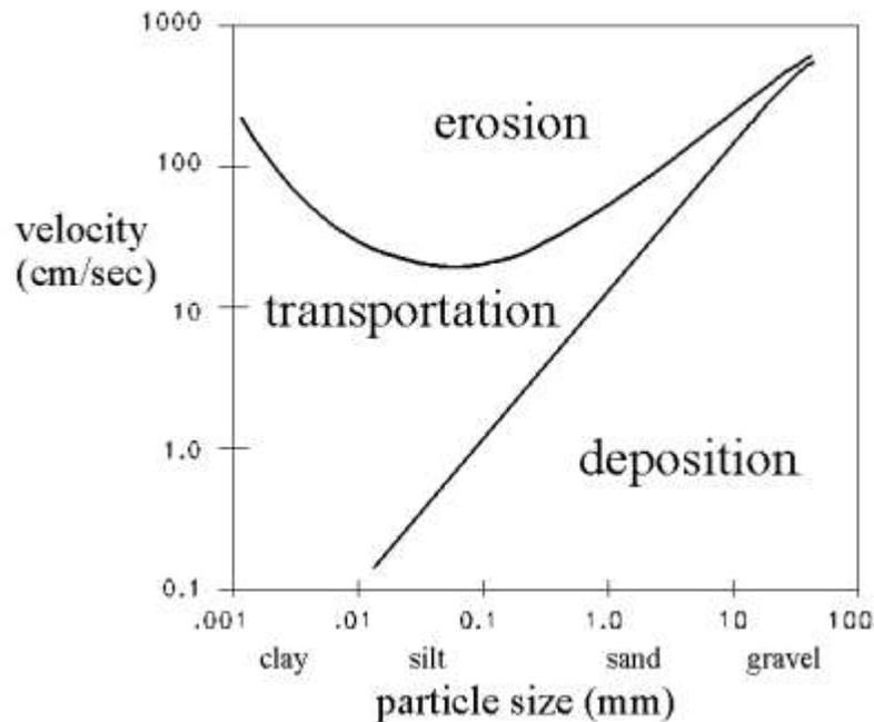
Figure 10. Hjulstrom's diagram, mean flow velocity required to initiate movement on a flat, uniform bed, for flow depth of 1 meter. The diagram shows the velocity a stream needs to pick up (erode), carry (transport), or drop (deposit) a clast or grain in flowing water.
