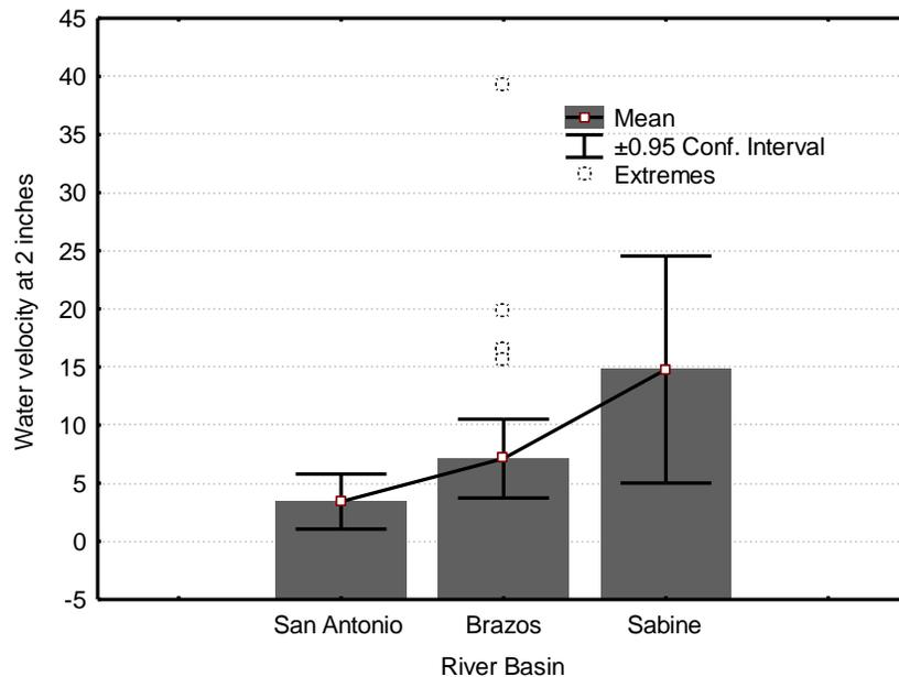
Figure 7. Average water velocity measurements (at 2 inches) recorded in the sampled river basins; the difference in velocity among river basins was significant ( $P = 0.011$ , Kruskal-Wallis test).
