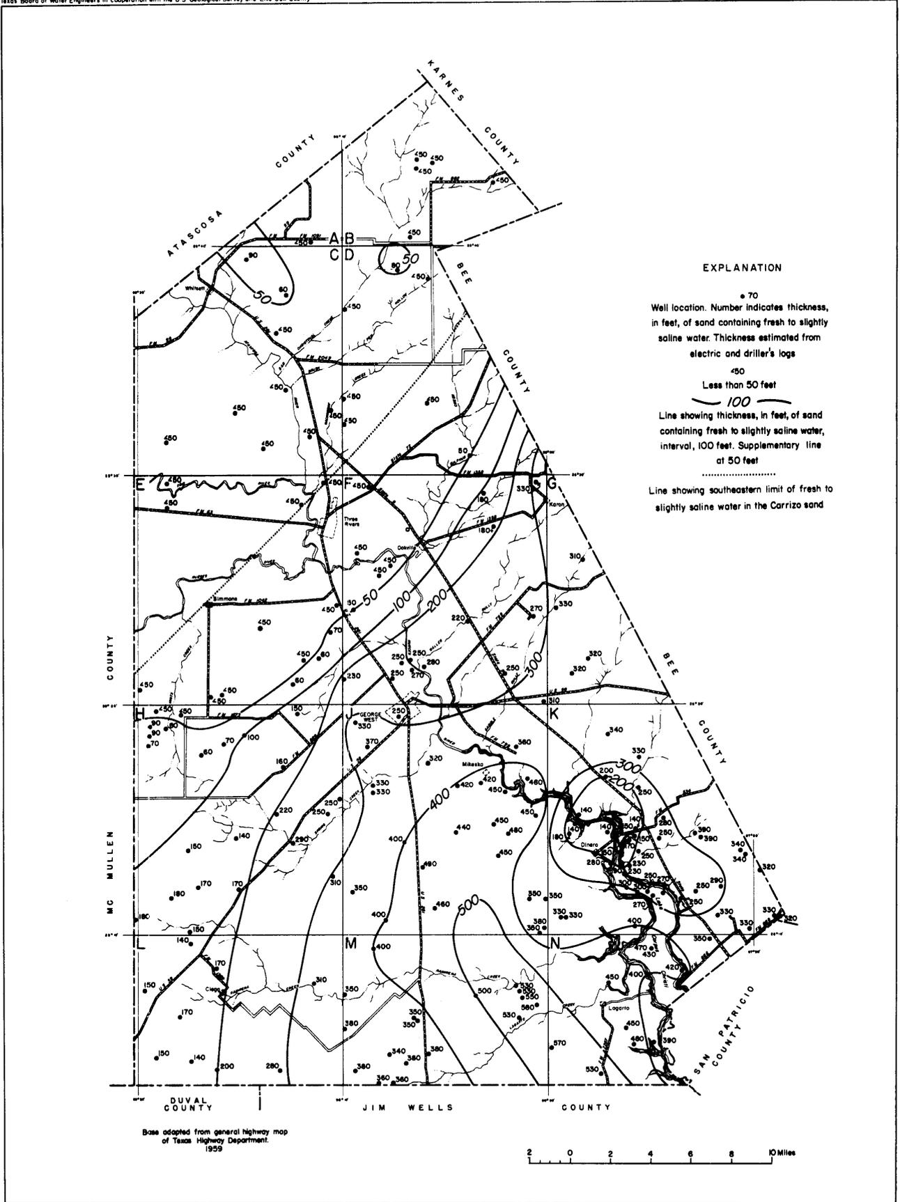
FIGURE 4.- Approximate thickness of sand containing fresh to slightly saline ground water, exclusive of the Carrizo sand, Live Oak County
