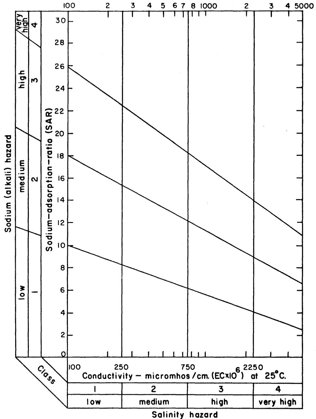
FIGURE 7.—Diagram for the classification of irrigation waters
