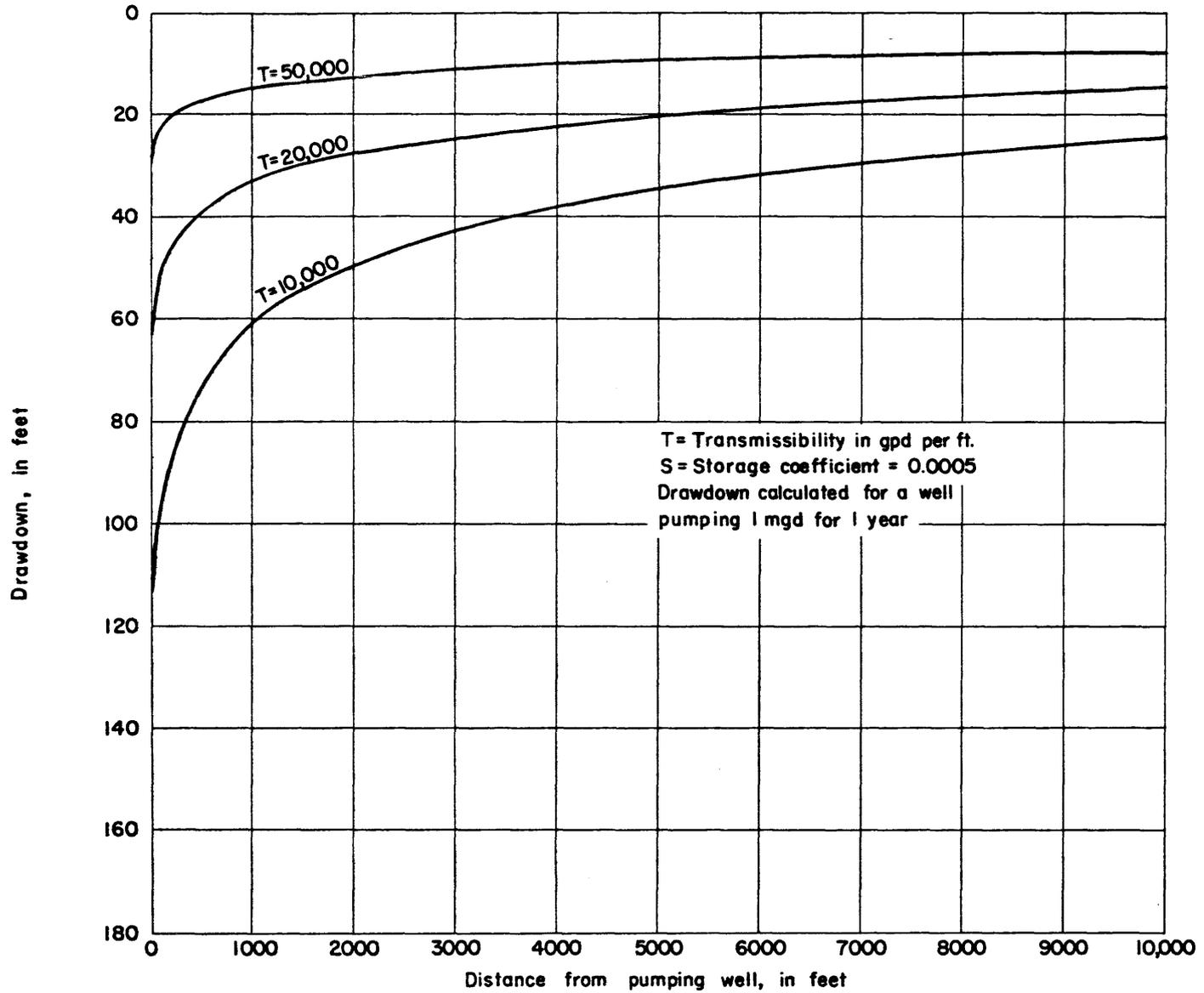
FIGURE 5.— Relation between drawdown and transmissibility in an infinite aquifer
