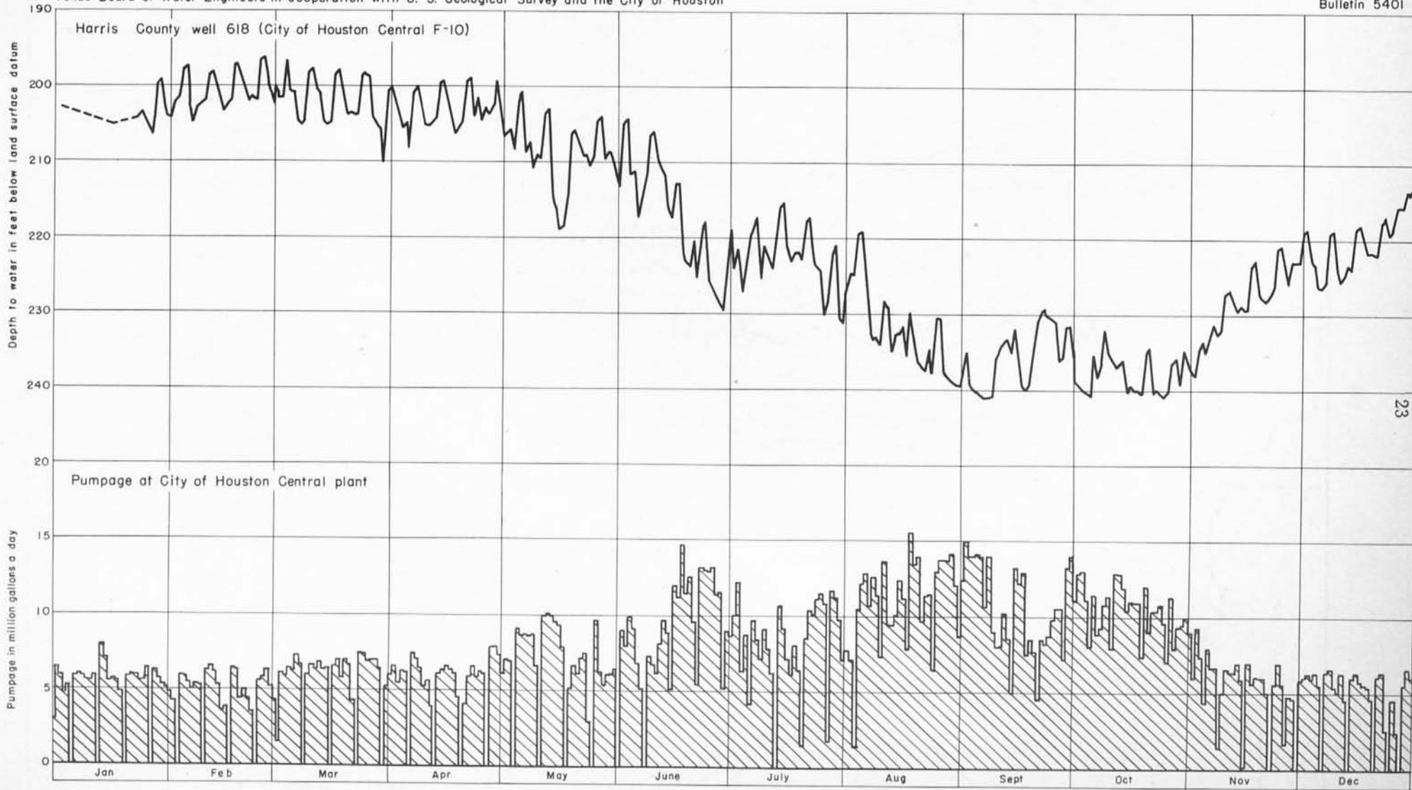
FIGURE 16:- Effect of pumping in City of Houston Central well field on water level in Central well F-10, 1952.
