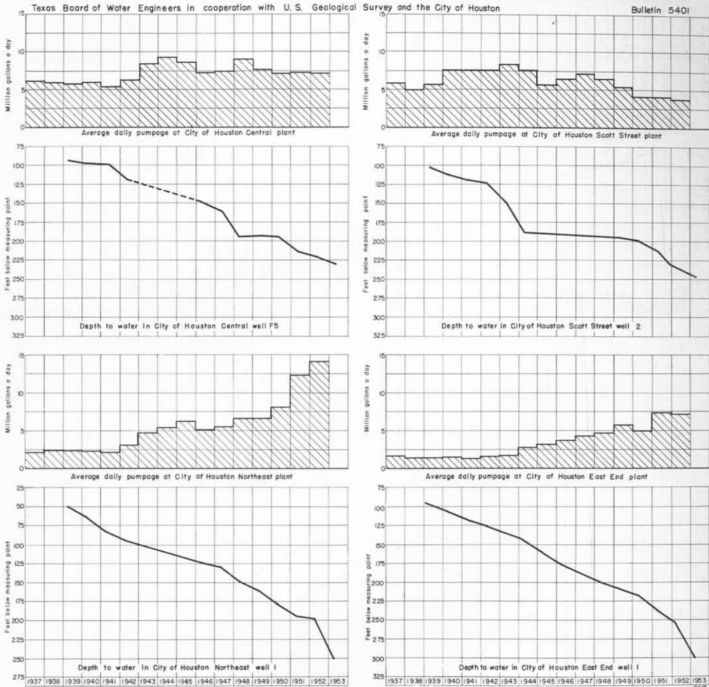
FIGURE 5.—Relation of pumpage to artesian pressure in Houston Central, Scott Street, Northeast, and East End well fields.
