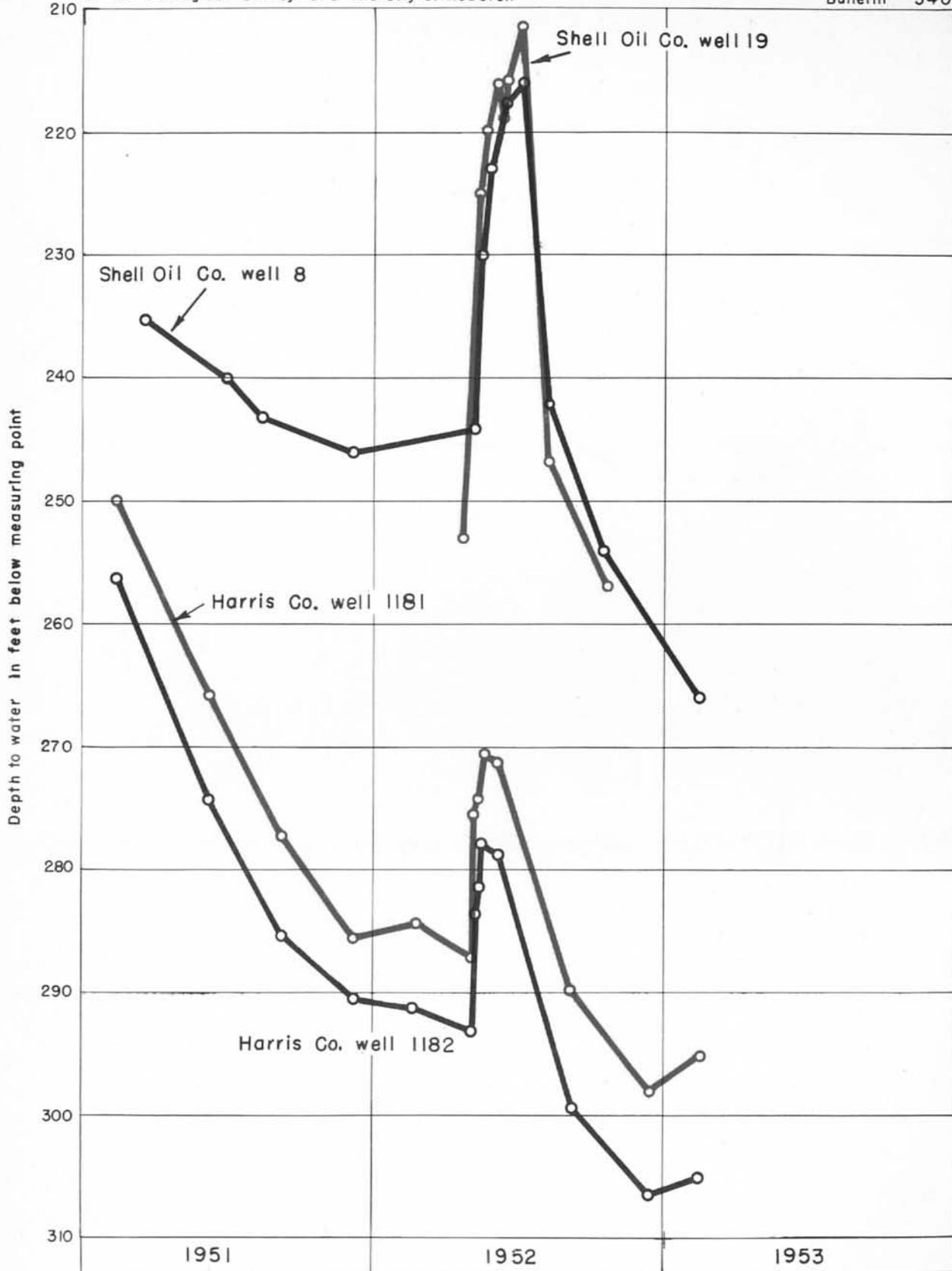
FIGURE II.- Recovery of water levels during shutdown of wells at Shell Oil Co., Sinclair Oil and Refining Co., and Crown-Central Petroleum Co. refineries, summer 1952
