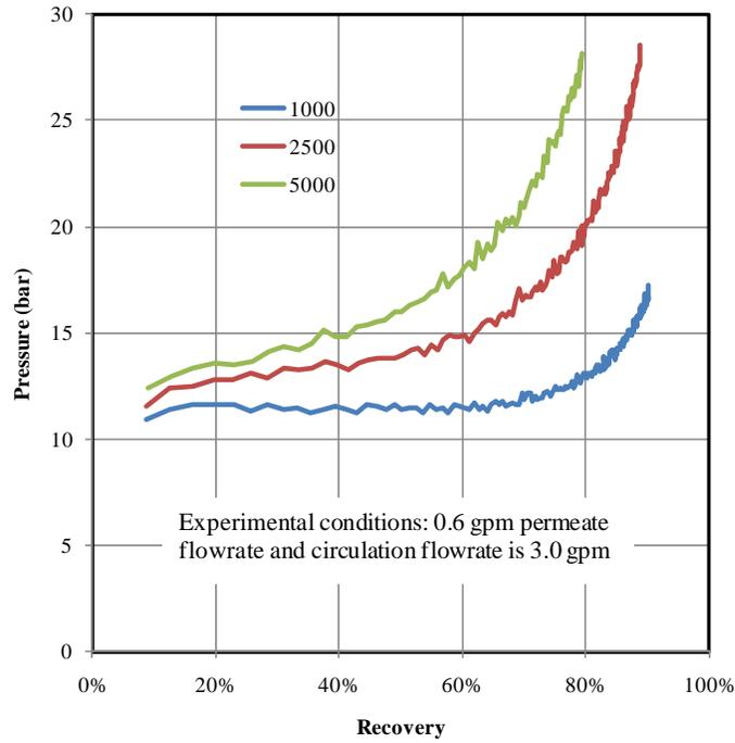
Figure 1. Pressure profiles during membrane filtration in the parallel RO system
