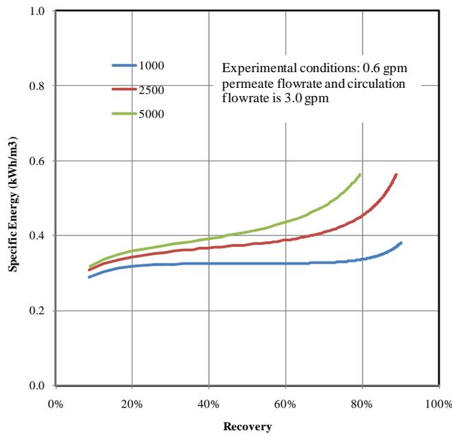
Figure 2. Specific energies as functions of recovery in the parallel RO system
