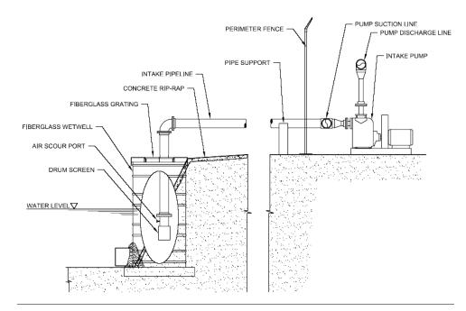
Figure 2-3: Schematic drawing of the intake for the Brownsville Seawater Desalination Pilot Project.
