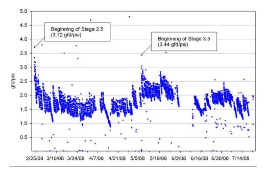
Figure 3-41: Permeability at 20°C, 25 gfd (TCEQ Stages 2 and 3), Pall MF membrane performance.
