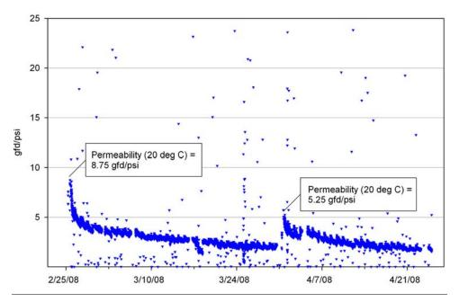
Figure 3-17: Operation at 15 gfd (TCEQ Stage 2), GE Zenon UF membrane performance.
