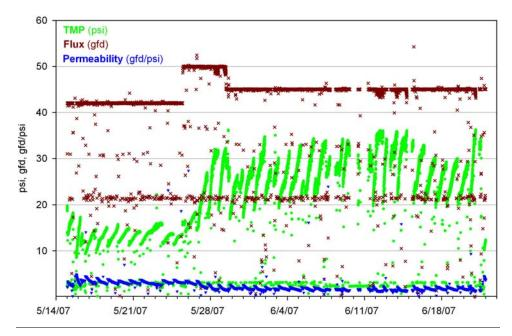
Figure 3-30: Optimization Run No. 1 (TCEQ Stage 1), Pall MF membrane performance.
