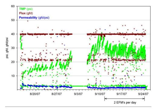
Figure 3-33: Operation at 40 gfd (TCEQ Stage 3), Pall MF membrane performance.
