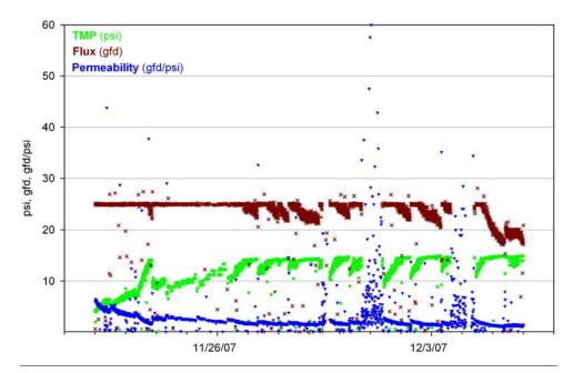
Figure 3-14: Operation at 25 gfd (TCEQ Stage 2), GE Zenon UF membrane performance.
