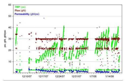
Figure 3-37: Operation at 30 gfd (TCEQ Stage 2), Pall MF membrane performance.
