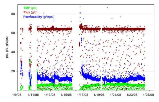
Figure 3-24: Operation at 65 gfd (TCEQ Stage 3), Norit UF membrane performance.
