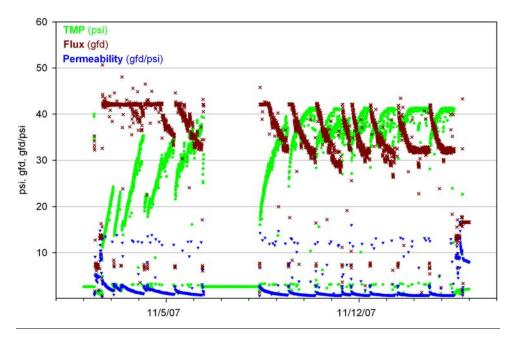
Figure 3-35: Optimization Run No. 2b (TCEQ Stage 1), Pall MF membrane performance.
