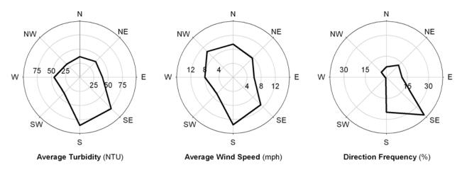
Figure 3-6: Relationship between wind direction and turbidity in the Brownsville Ship Channel during the Pilot Study.
