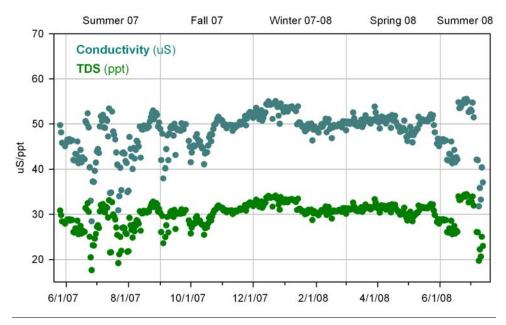
Figure 3-8: Raw water conductivity and TDS during the Pilot Study.
