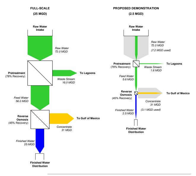
Figure 5-1: Comparison schematic between the full-scale (25 mgd) and recommended demonstration-scale (2.5 mgd) seawater desalination projects.
