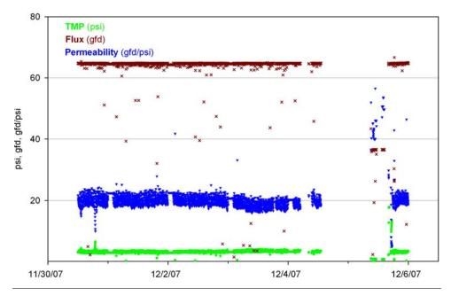
Figure 3-22: Optimization Run No. 2 (TCEQ Stage 1), Norit UF membrane performance.
