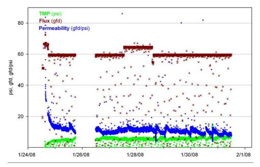
Figure 3-25: Operation at 60 gfd (TCEQ Stage 2), Norit UF membrane performance.
