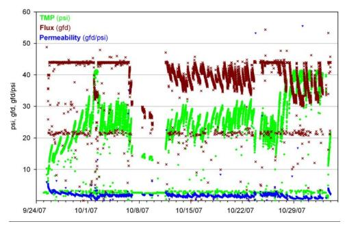
Figure 3-34: Optimization Run No. 2a (TCEQ Stage 1), Pall MF membrane performance.
