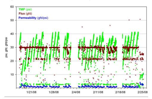
Figure 3-39: Operation at 30 gfd (TCEQ Stage 3), Pall MF membrane performance.
