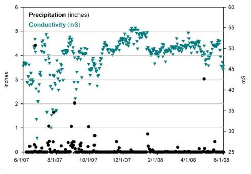
Figure 3-9: The relationship between precipitation and raw water conductivity in the Brownsville Ship Channel during the Pilot Study.
