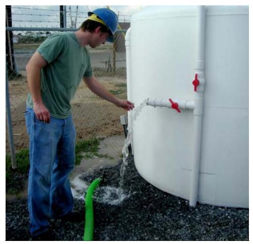
Figure 2-11: Photograph showing the collection of a sample for testing chlorine residual in RO feed stream.
