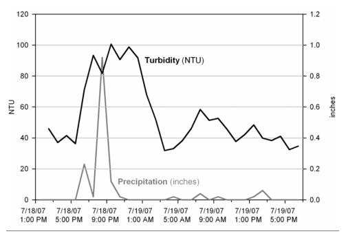
Figure 3-5: An example of the temporal impact rainfall had on raw water turbidity in the Brownsville Ship Channel during the Pilot Study.
