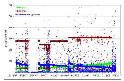
Figure 3-12: Optimization run No. 1 (TCEQ Stage 1), GE Zenon UF membrane performance.
