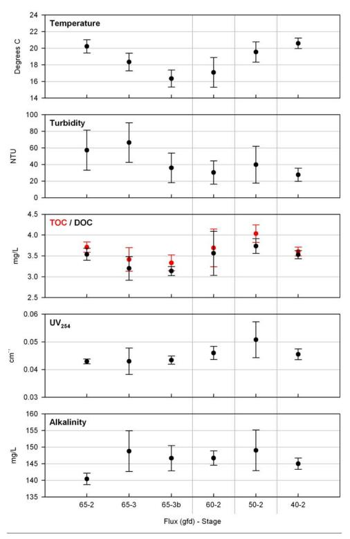
Figure 3-29: Raw water quality for selected parameters during the Norit UF runs.
