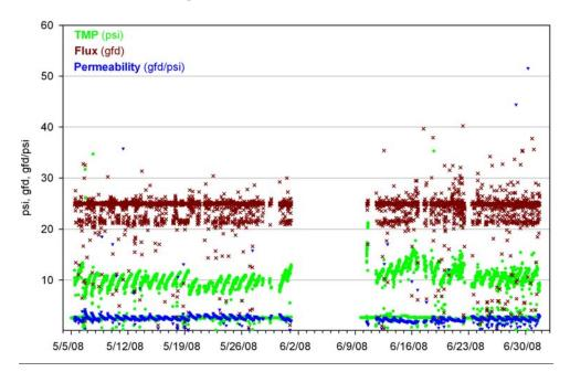
Figure 3-42: Operation at 25 gfd (TCEQ Stage 3), Pall MF membrane performance.
