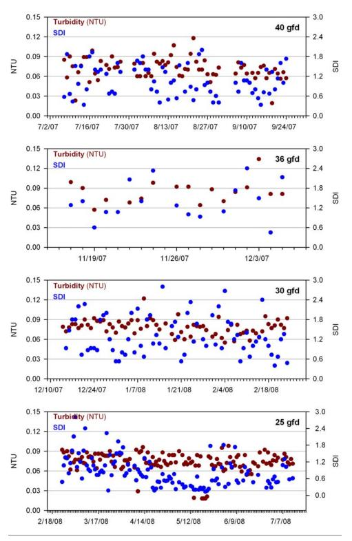
Figure 3-43: Summary of filtrate water quality results for Pall UF.
