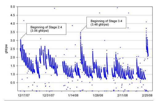
Figure 3-38: Permeability at 20°C, 30 gfd (TCEQ Stages 2 and 3), Pall MF membrane performance.
