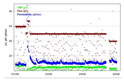
Figure 3-26: Operation at 50 gfd (TCEQ Stage 2), Norit UF membrane performance.
