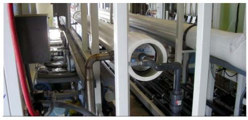
Figure 3-45: Photograph of seawater RO pressure vessels used during the Pilot Study.
