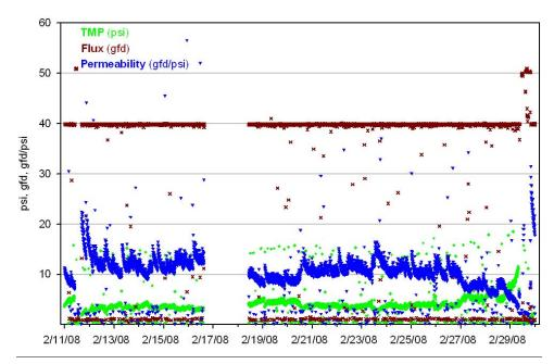
Figure 3-27: Operation at 40 gfd (TCEQ Stage 2), Norit UF membrane performance.
