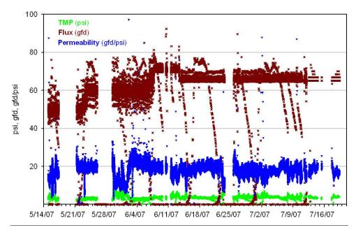
Figure 3-21: Optimization Run No. 1 (TCEQ Stage 1), Norit UF membrane performance.
