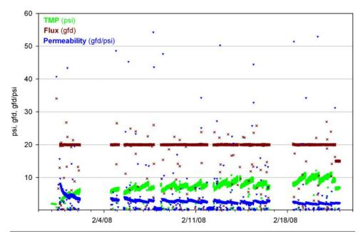
Figure 3-15: Operation at 20 gfd (TCEQ Stage 2), GE Zenon UF membrane performance.
