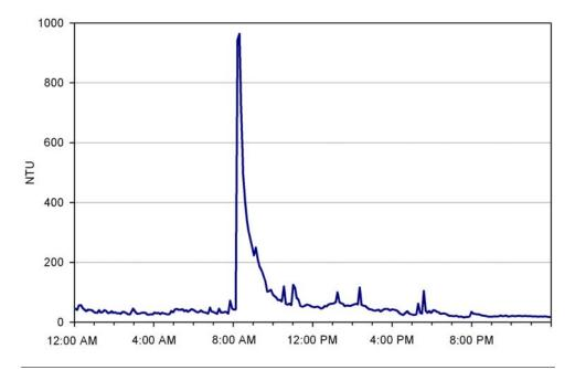
Figure 3-3: Snapshot of raw water turbidity spike caused by a passing cargo ship, 12/26/07.
