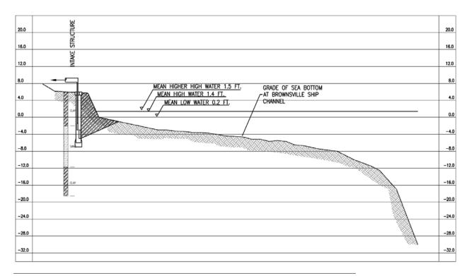
Figure 2-4: Cross sectional view of the intake structure in relation to the Brownsville Ship Channel.
