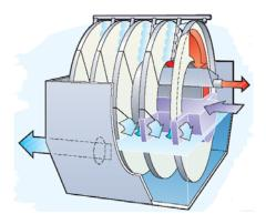
Figure 2-8: Schematic drawing of the Hydrotech Discfilter<sup>9</sup>.
