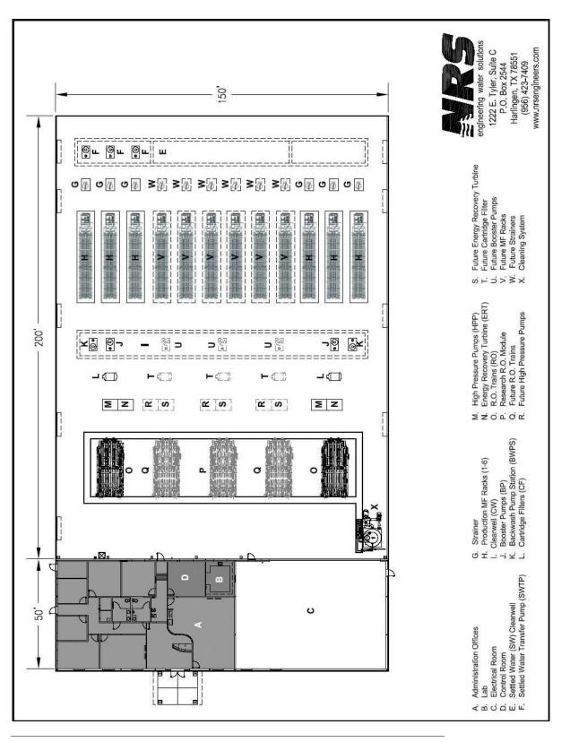
Figure 5-6: Layout of the treatment systems and building for the proposed 2.5 mgd Demonstration Project.
