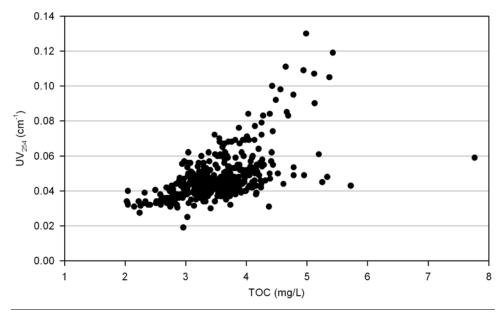
Figure 3-11: Correlation between raw water TOC and UV<sub>254</sub> during the Pilot Study.
