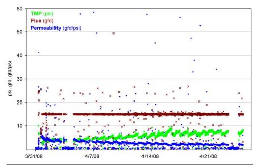
Figure 3-18: Operation at 15 gfd (TCEQ Stage 3), GE Zenon UF membrane performance.
