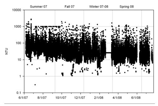
Figure 3-2: Raw water turbidity in the Brownsville Ship Channel.
