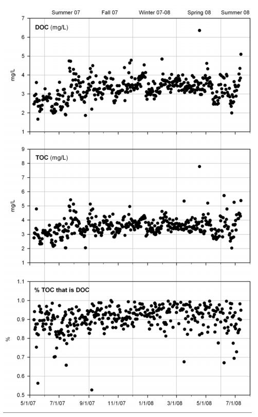
Figure 3-10: Raw water DOC, TOC, and percent of TOC that is DOC during the Pilot Study.
