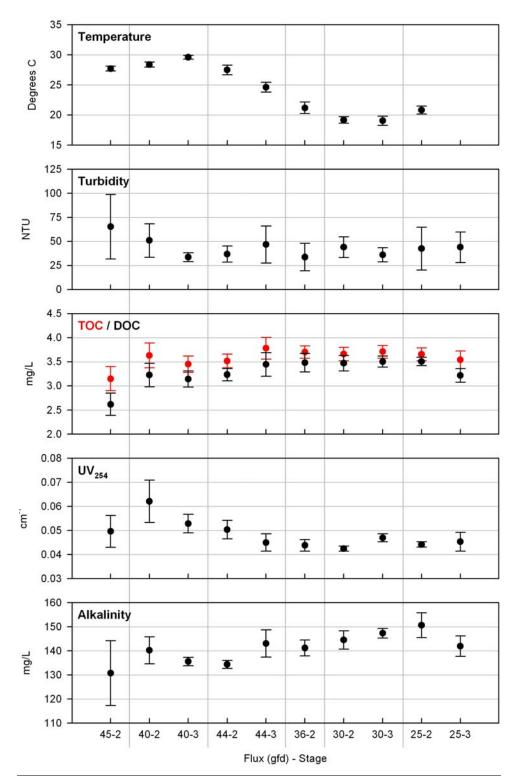
Figure 3-44: Raw water quality for selected parameters during the Pall MF runs.
