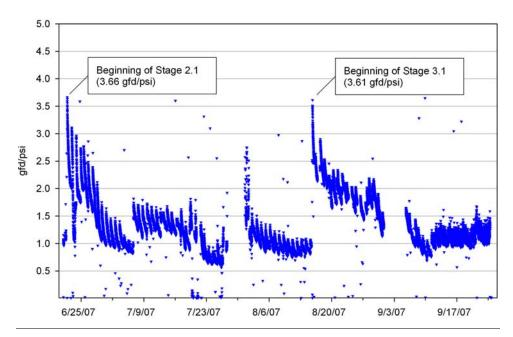
Figure 3-32: Permeability at 20°C, 40 gfd (TCEQ Stages 2 and 3), Pall MF membrane performance.
