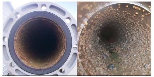
Figure 3-55: Photograph of biogrowth and barnacles attached to the inner wall of the raw water manifold. The intake had been operational for approximately 12 months prior to this photograph.
