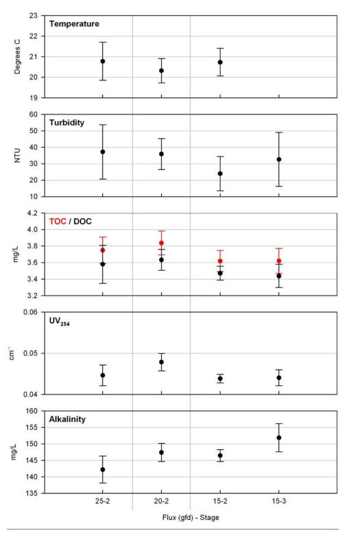
Figure 3-20: Raw water quality for selected parameters during the GE Zenon UF runs.
