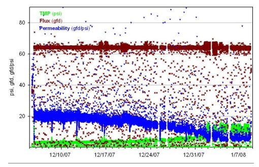
Figure 3-23: Operation at 65 gfd (TCEQ Stage 2), Norit UF membrane performance.
