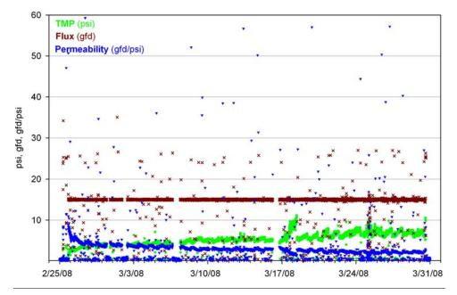
Figure 3-16: Operation at 15 gfd (TCEQ Stage 2), GE Zenon UF membrane performance.
