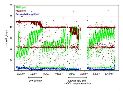
Figure 3-31: Operation at 40 gfd run (TCEQ Stage 2), Pall MF membrane performance.
