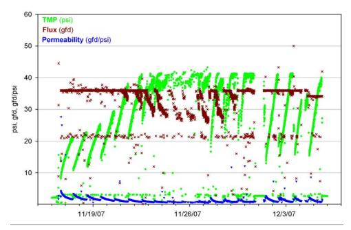
Figure 3-36: Operation at 36 gfd (TCEQ Stage 2), Pall MF membrane performance.
