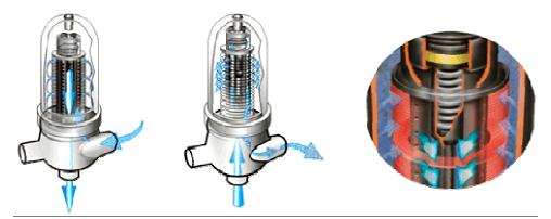
Figure 2-7: Schematic drawing of the Arkal Disc Filter<sup>7</sup>.
