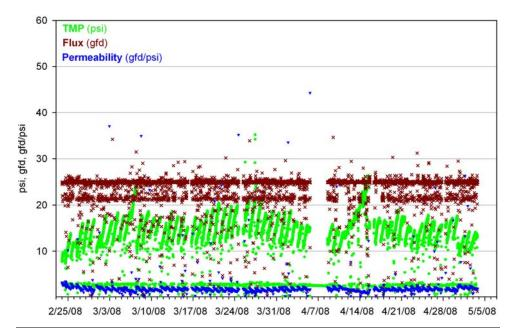
Figure 3-40: Operation at 25 gfd (TCEQ Stage 2), Pall MF membrane performance.
