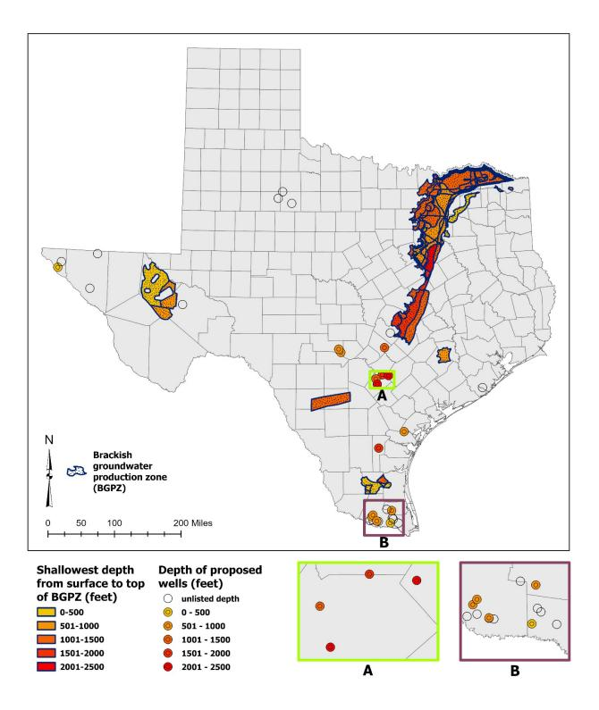
Figure 3: Depth of wells of recommended brackish groundwater desalination projects (if listed) compared to shallowest depth to the top of a brackish groundwater production zones (BGPZs).
