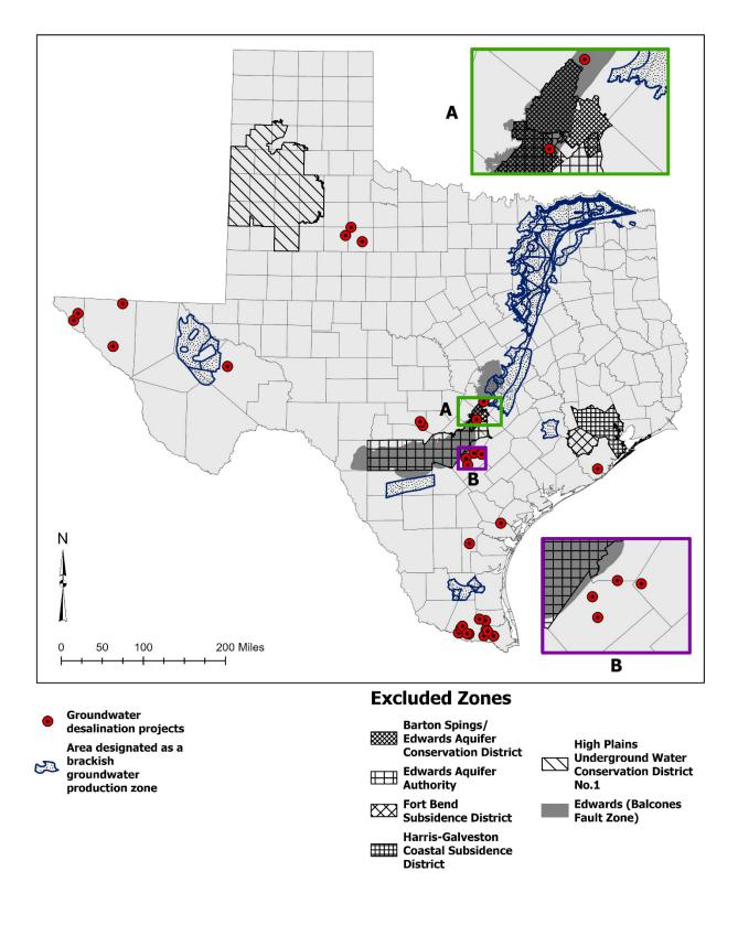
Figure 2: Location of recommended brackish groundwater desalination projects relative to brackish groundwater production zones (BGPZs).
