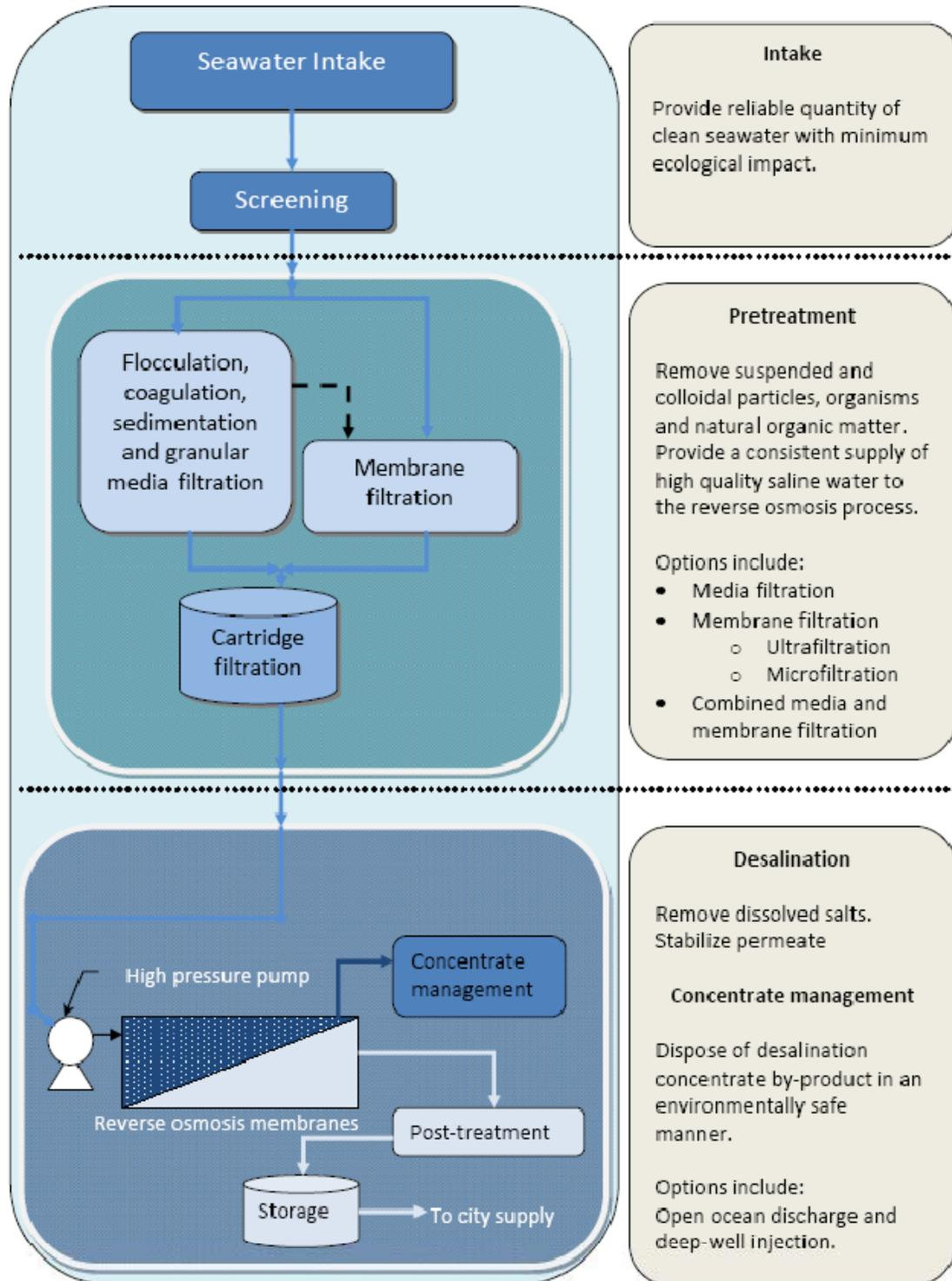
**Figure 2 - Components of the seawater desalination by reverse-osmosis process**
