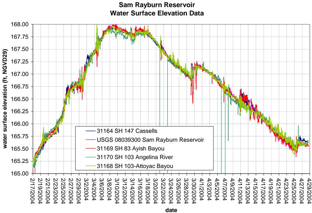
**Figure 4** – Water surface elevation at each water level installation.
