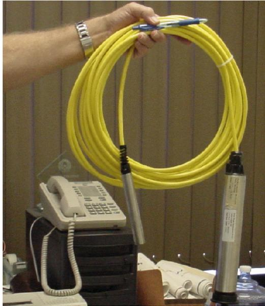
**Figure 1** – Photo of water level loggers used for this study.
