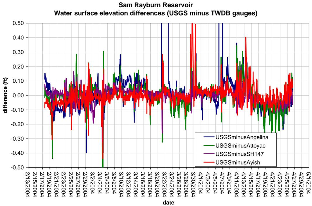
**Figure 5** – Difference of water surface elevation at each TWDB installation compared to the USGS Sam Rayburn Reservoir gauge.
