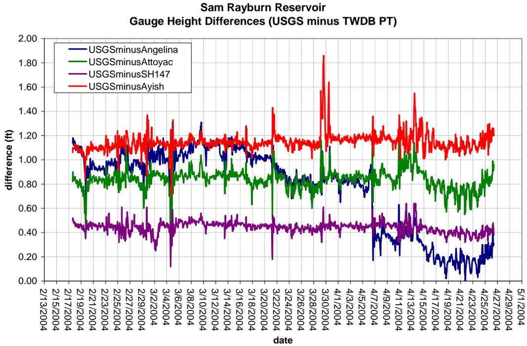
**Figure 3** – Difference of water height above each TWDB pressure transducer from water height above USGS Sam Rayburn Reservoir gauge datum.
