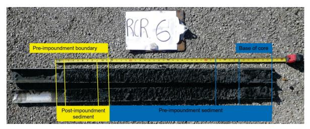
Figure 7. Sediment core RCR-6 from Richland-Chambers Reservoir. Post-impoundment sediment layers occur in the top 11.0 inches of this sediment core (identified by the yellow box). Pre-impoundment sediment layers were identified and are defined by the blue box.
