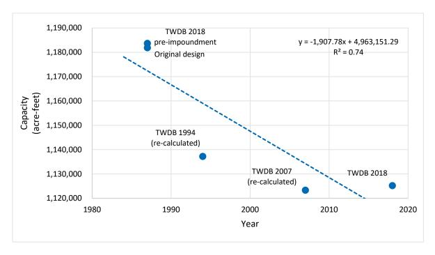
Figure 11. Plot of current and previous capacity estimates (acre-feet) for Richland-Chambers Reservoir. Capacity estimates for each survey plotted as blue dots. The blue trend line illustrates the average loss of capacity through 2018 based on all available survey data.
