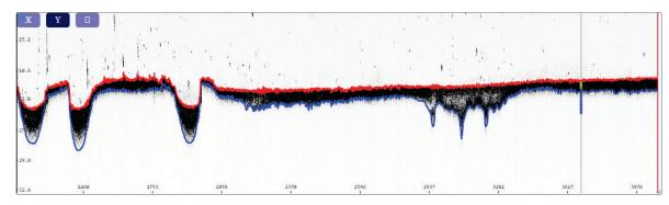
Figure 9. Cross-section of data collected during survey, displayed in Hydropick (208 kHz frequency), correlated with sediment core sample RCR-6 and showing the current surface in red and pre-impoundment surface in blue.
