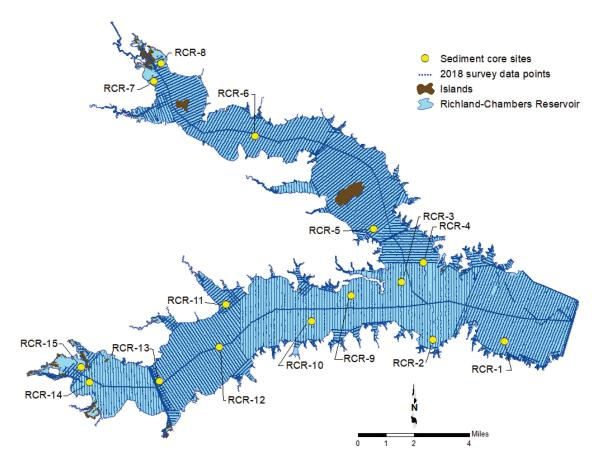
Figure 2. 2018 TWDB Richland-Chambers Reservoir survey data (*blue dots*) and sediment coring locations (*yellow circles*)
