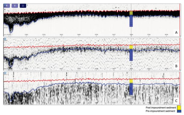
Figure 8. Comparison of sediment core RCR-6 with acoustic signal returns. A) 208 kHz frequency, B) 50 kHz frequency, and C) 12 kHz frequency. The current surface in red and preimpoundment surface in blue.
