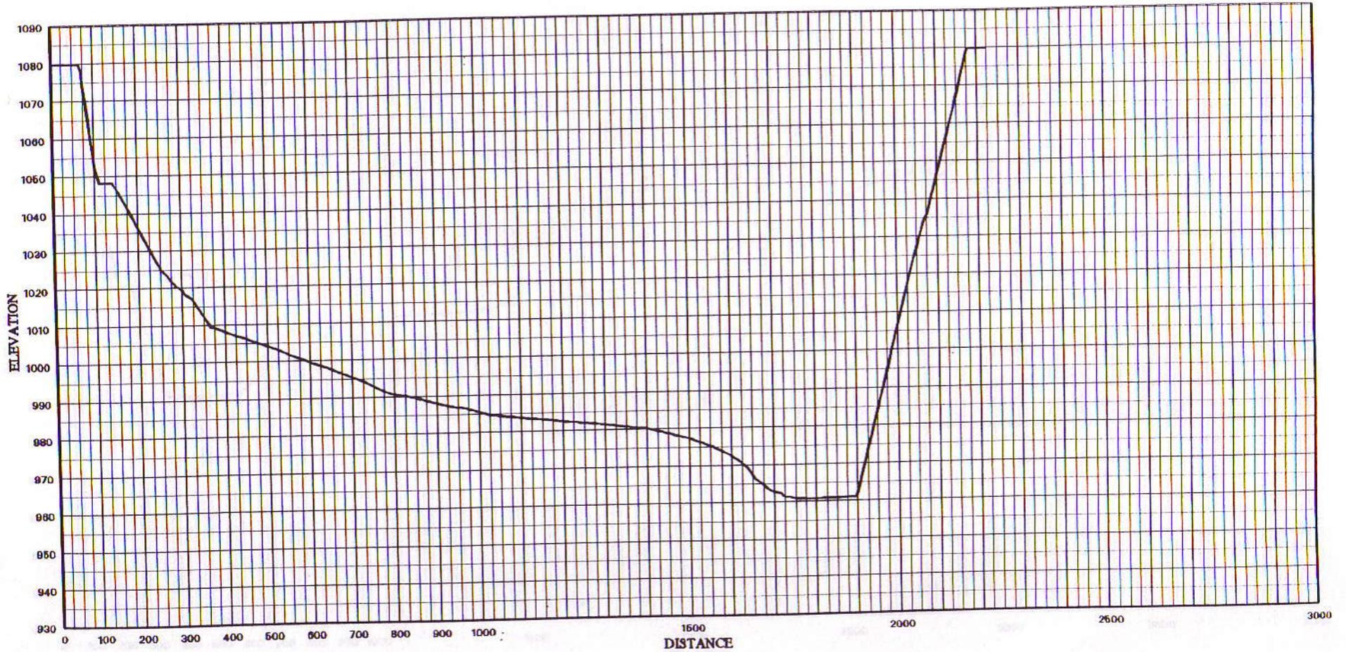
— Range Line Generated Using ARC/INFO's TIN Module
