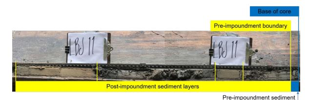
Figure 7. Sediment core LBJ-11 from Lake LBJ. Post-impoundment sediment layers occur in the top 50.0 inches of this sediment core (identified by the yellow box). Pre-impoundment sediment layers were identified and are defined by the blue box.
