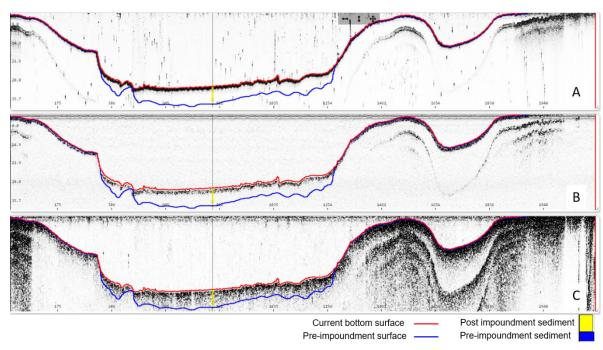
Figure 8. Comparison of sediment core LBJ-11 with acoustic signal returns. A) 208 kHz frequency, B) 50 kHz frequency, and C) 12 kHz frequency. The current surface in red and preimpoundment surface in blue.
