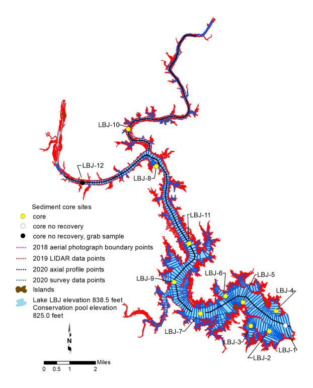
Figure 2. 2020 TWDB Lake LBJ survey data (*blue dots*), sediment coring locations (*circles*), and 2019 LIDAR data (*red dots*).
