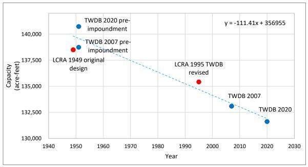
Figure 10. Plot of current and previous capacity estimates (acre-feet) at elevation 825.0 feet for Lake LBJ. Capacity estimates for each TWDB survey plotted as blue dots and other surveys as red dots. The blue trend line illustrates the total average loss of capacity through 2020. The 2007 TWDB pre-impoundment estimate is not included in the trendline calculation and is for informational purposes only.
