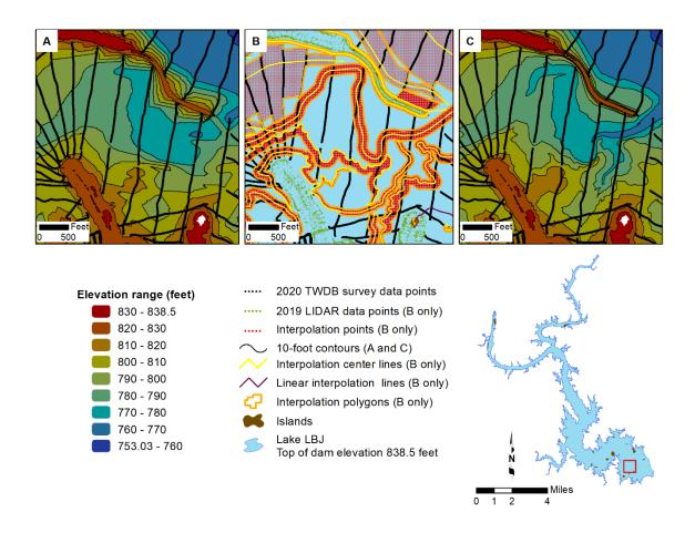
Figure 3. Anisotropic spatial interpolation as applied to Lake LBJ sounding data; A) bathymetric contours without interpolated points, B) sounding points (*black*) and interpolated points (*red*), C) bathymetric contours with interpolated points.
