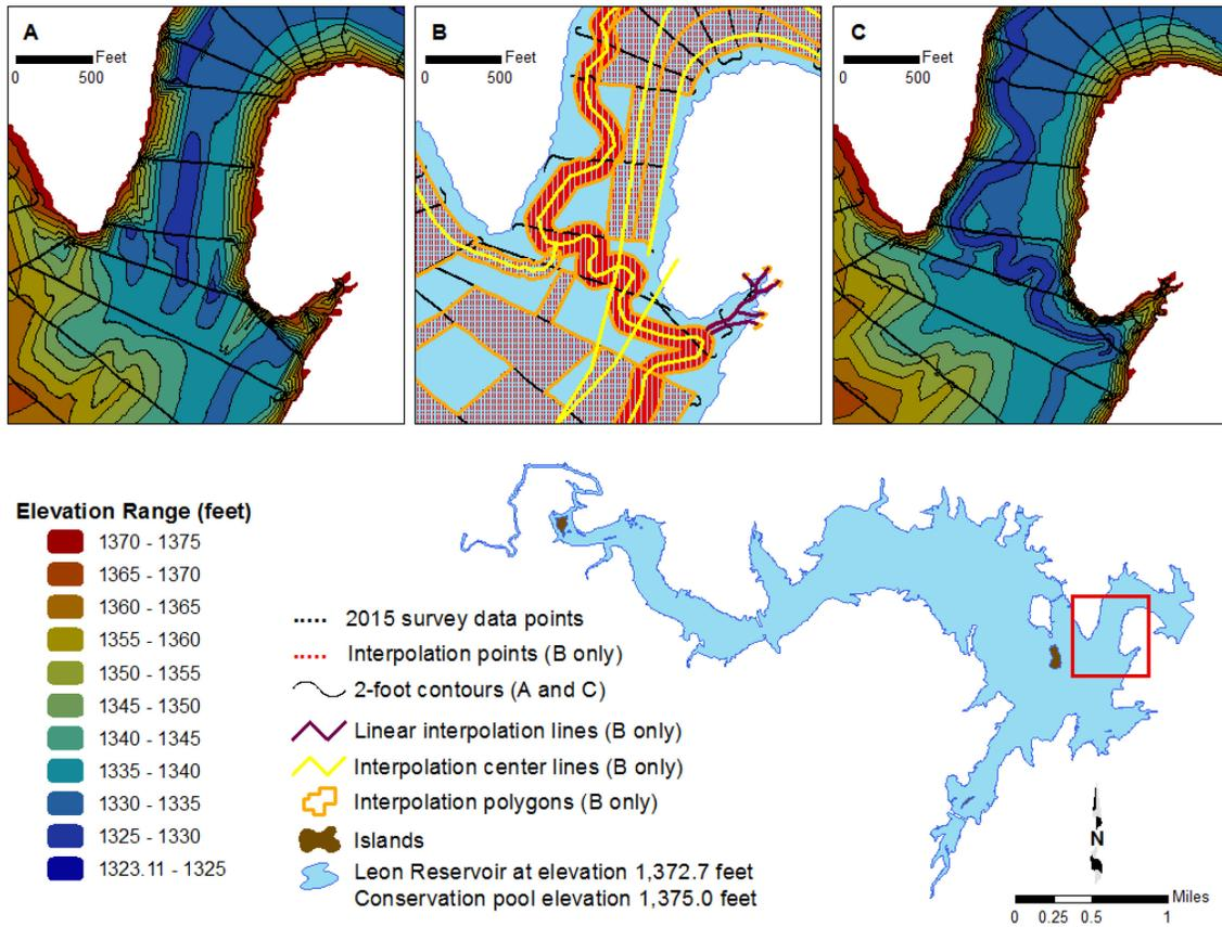
**Figure 3. Anisotropic spatial interpolation and linear interpolation of Leon Reservoir sounding data - A) bathymetric contours without interpolated points, B) sounding points (black) and interpolated points (red), C) bathymetric contours with the interpolated points**
