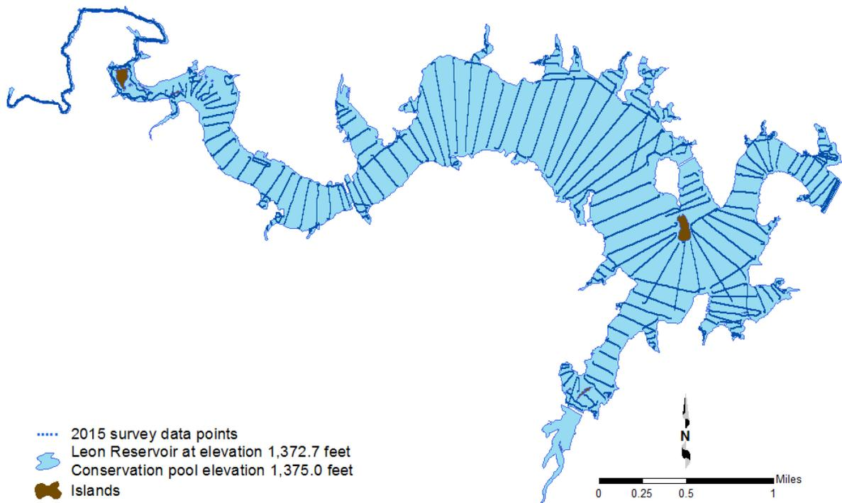
**Figure 2. Data collected during 2015 TWDB Leon Reservoir survey**
