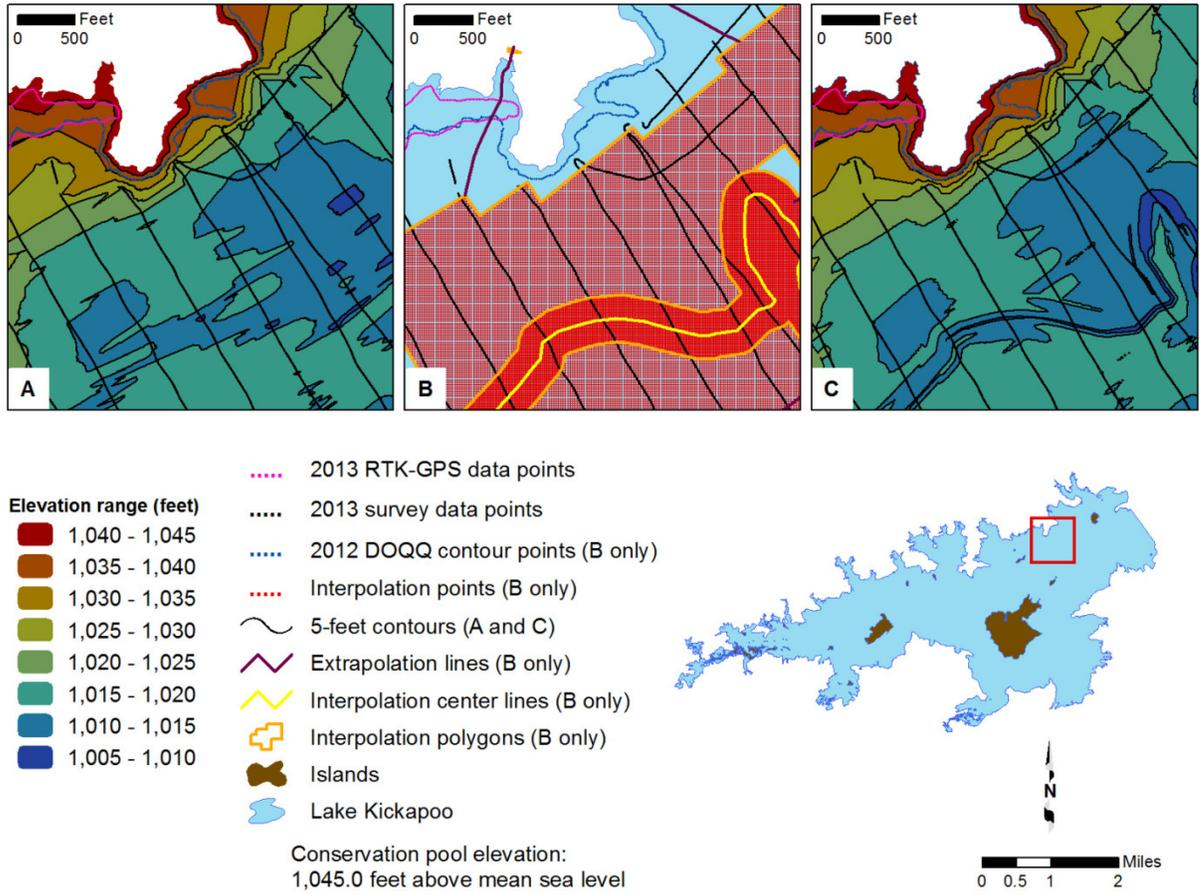
**Figure 3. Anisotropic spatial interpolation and linear extrapolation of Lake Kickapoo sounding data - A) bathymetric contours without interpolated points, B) sounding points (black) and interpolated points (red), C) bathymetric contours with the interpolated points**
