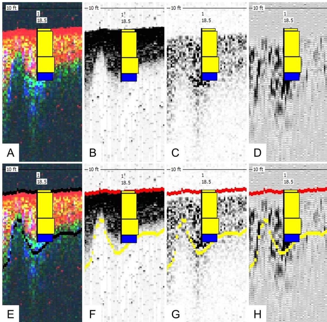
**Figure 8. Comparison of sediment core BA-1 with acoustic signal returns: A,E) combined acoustic signal returns, B,F) 208 kHz frequency, C,G) 50 kHz frequency, D,H) 24 kHz frequency**
