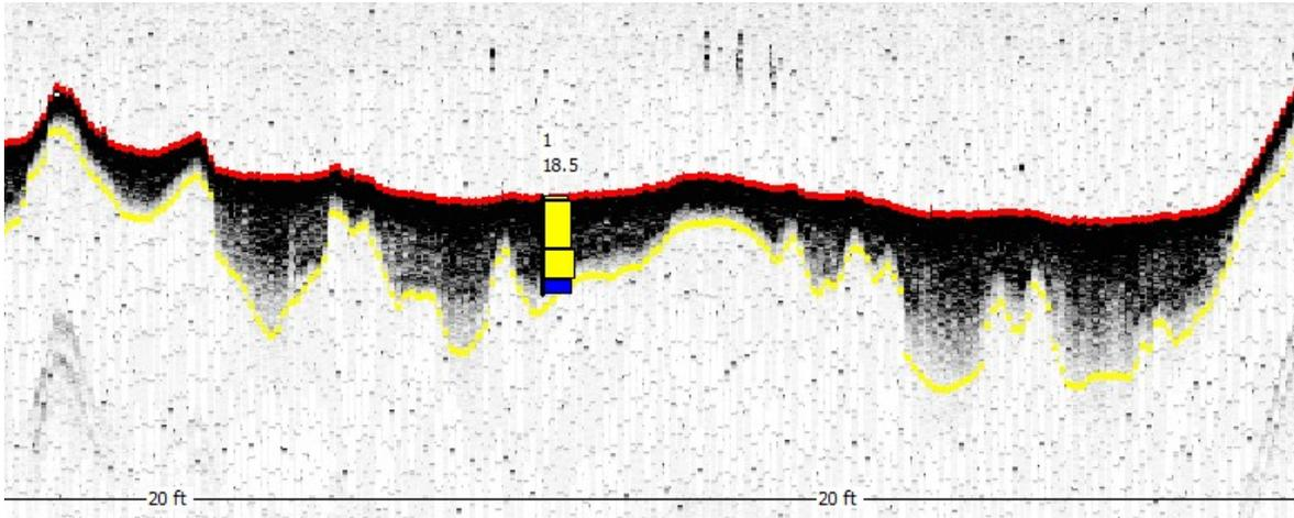
**Figure 9. Cross-section of data collected during survey, displayed in DepthPic© (208 kHz frequency), correlated with sediment core sample BA-1 and showing the current surface in red and pre-impoundment surface in yellow**
