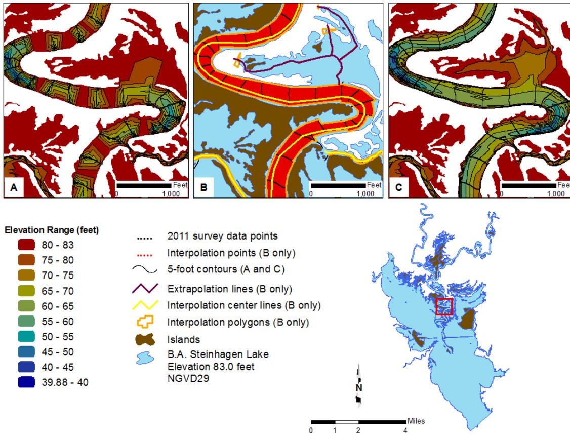
**Figure 3. Anisotropic spatial interpolation and linear extrapolation of B.A. Steinhagen Lake sounding data - A) bathymetric contours without interpolated points, B) sounding points (black) and interpolated points (red), C) bathymetric contours with the interpolated points**
