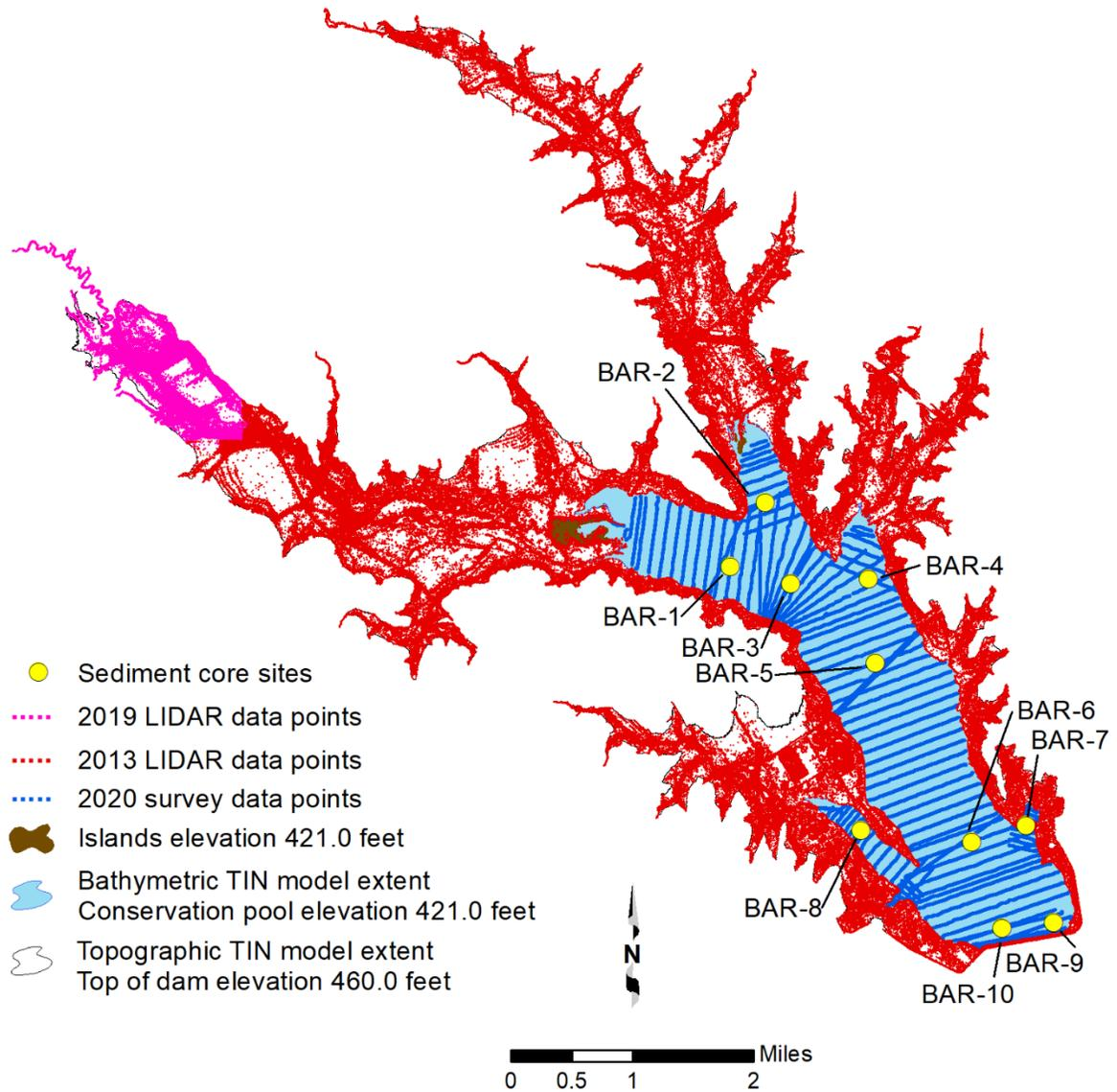
**Figure 2.** 2020 TWDB sounding data (*blue dots*), 2019 LIDAR data (*pink dots*), 2013 LIDAR data (*red dots*), and sediment coring locations (*yellow circles*).
