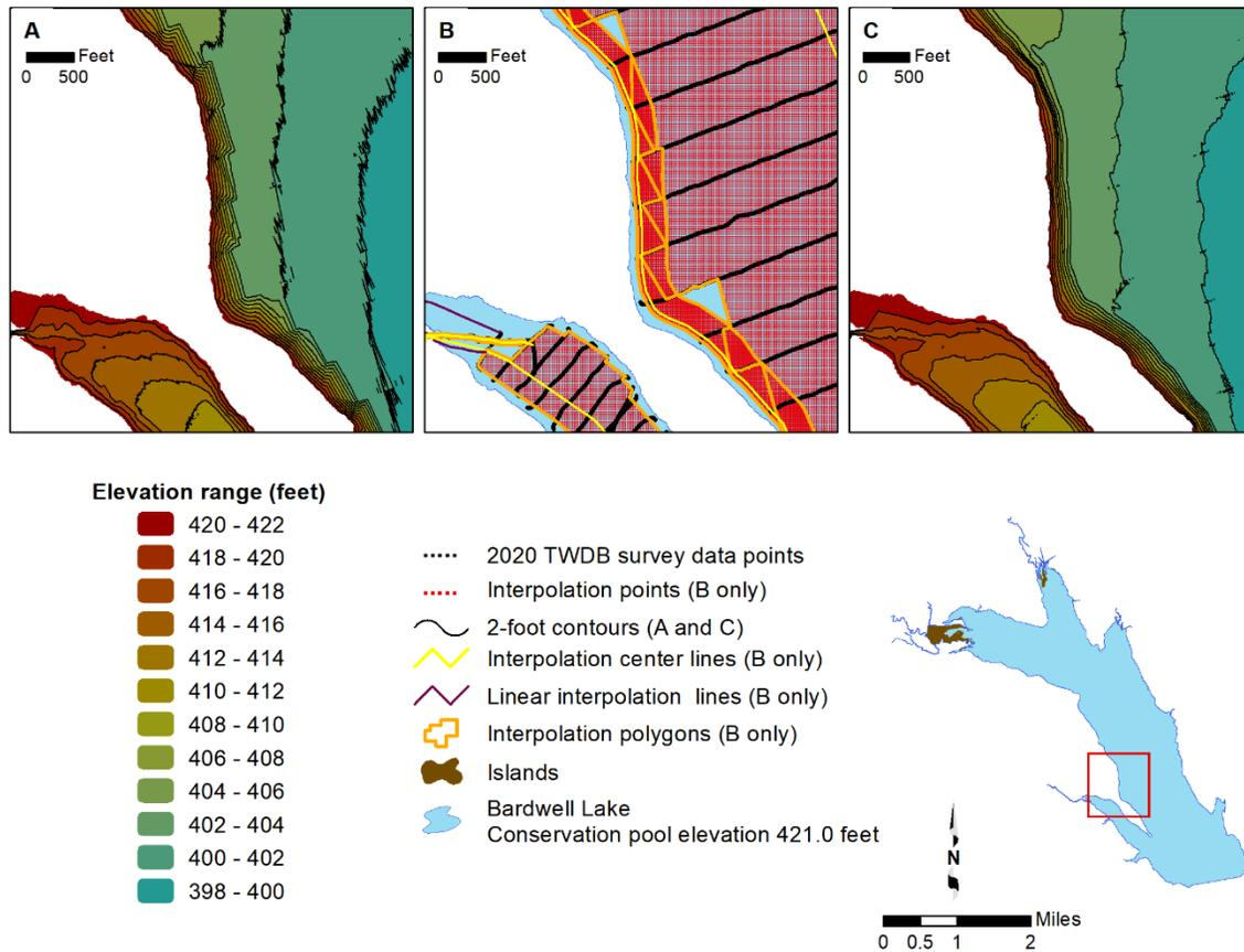
**Figure 3. Anisotropic spatial interpolation and linear interpolation as applied to Bardwell Lake sounding data; A) bathymetric contours without interpolated points, B) sounding points (black) and interpolated points (red), C) bathymetric contours with interpolated points.**
