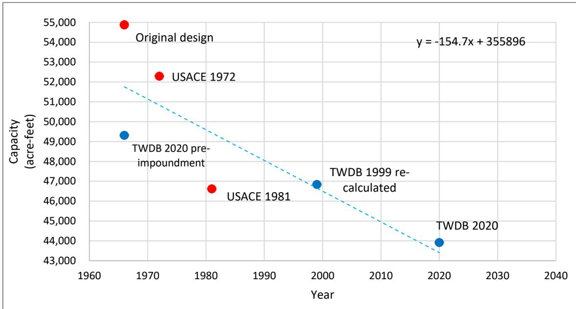
**Figure 10. Plot of current and previous capacity estimates (acre-feet) at elevation 421.00 feet. Capacity estimates for each TWDB survey plotted as blue dots and other surveys as red dots. The blue trend line illustrates the total average loss of capacity through 2020.**
