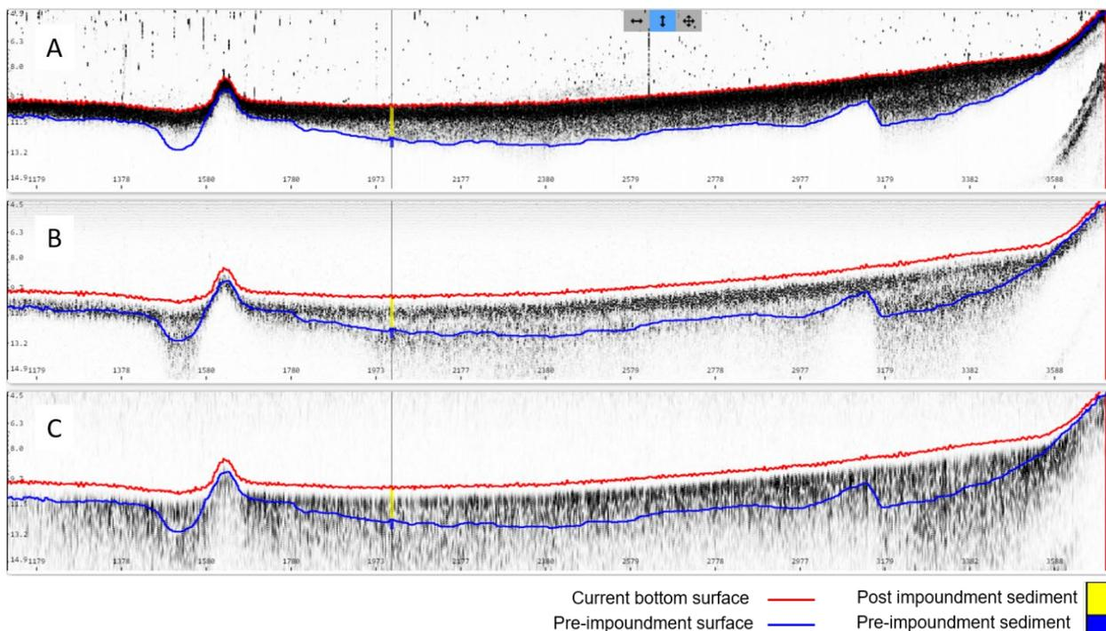
**Figure 8. Sediment core sample BAR-3 compared with acoustic signal returns. A) 208 kHz frequency, B) 50 kHz frequency, and C) 12 kHz frequency.**
