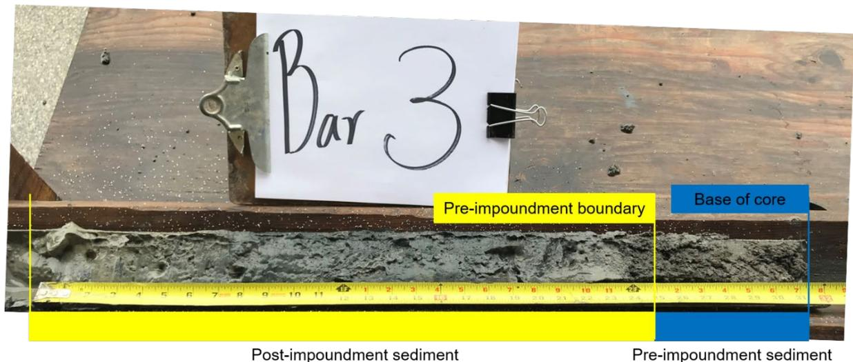
**Figure 7. Sediment cores BAR-3. Post-impoundment sediment layers are identified by yellow boxes. Pre-impoundment sediment layers are identified by blue boxes.**
