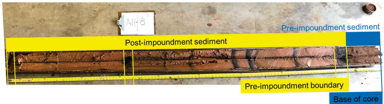
Figure 7. Sediment core AH-8 from Alan Henry Reservoir. Post-impoundment sediment layers occur in the top 104.5 inches of this sediment core (identified by the yellow box). Pre-impoundment sediment layers were identified and are defined by the blue box.
