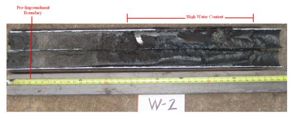
Figure D2 – Sediment Core W-2 from Lake Weatherford, showing the pre-impoundment boundary 4 inches above the base of the core (left). The pre-impoundment boundary is marked by the change in soil structure below and above the area 4" up from the core base. Above 20" from the core base, the sediment moisture content is extremely high.
