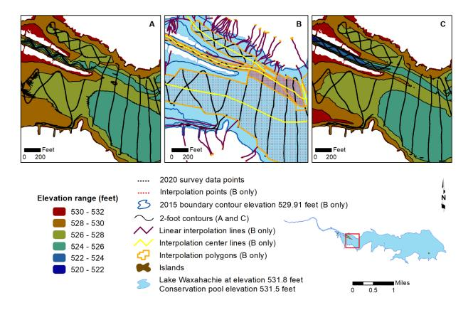
Figure 3. Anisotropic spatial interpolation and linear interpolation as applied to Lake Waxahachie sounding data; A) bathymetric contours without interpolated points, B) sounding points (*black*) and interpolated points (*red*), C) bathymetric contours with interpolated points.
