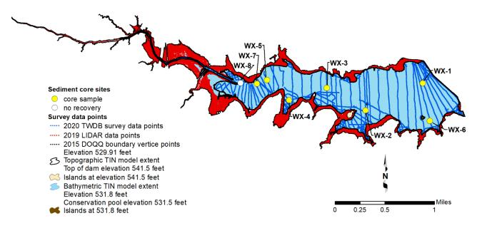
Figure 2. 2020 TWDB sounding data (*blue dots*), 2019 LIDAR data (*red dots*), and sediment coring locations (*yellow circles*).
