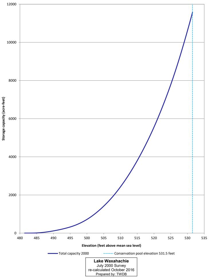
Appendix C: 2000 re-calculated capacity curve
