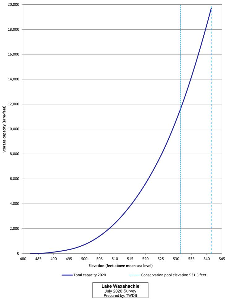
Appendix K: Bathymetric and topographic capacity curve
