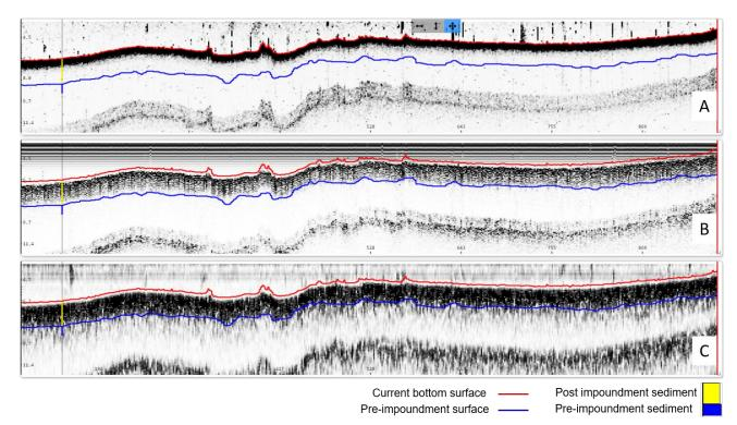
Figure 8. Sediment core sample WX-7 compared with acoustic signal returns. A) 208 kHz frequency, B) 50 kHz frequency, and C) 12 kHz frequency.
