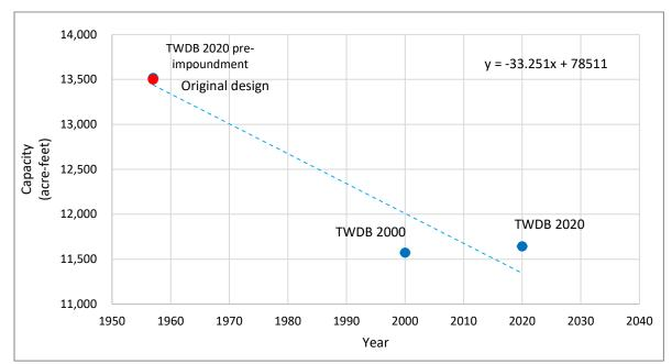
Figure 10. Plot of current and previous capacity estimates (acre-feet) at elevation 531.50 feet. Capacity estimates for TWDB surveys plotted with blue dots and other surveys with a red dot. The blue trend line illustrates the total average loss of capacity through 2020.
