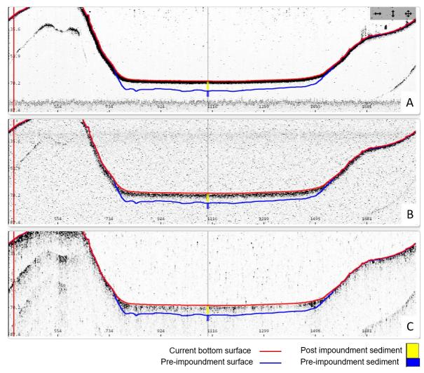
Figure 8. Sediment core sample LT-6 compared with acoustic signal returns. A) 208 kHz frequency, B) 50 kHz frequency, and C) 12 kHz frequency.
