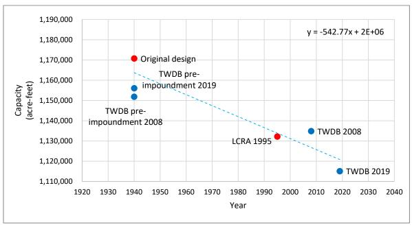
Figure 10. Plot of current and previous capacity estimates (acre-feet) at elevation 681.0 feet. Capacity estimates for each TWDB survey plotted as blue dots and other surveys as red dots. The blue trend line illustrates the total average loss of capacity through 2019. The TWDB pre-impoundment estimate from 2008 is plotted for informational purposes and was not considered in the trend line calculation.
