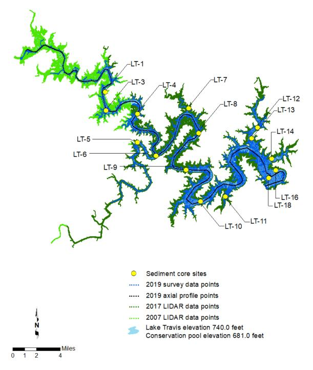
Figure 2. 2019 TWDB sounding data (*blue dots*), sediment coring locations (*yellow circles*), 2007 LIDAR data (*light green dots*), and 2017 LIDAR data (dark *green dots*).
