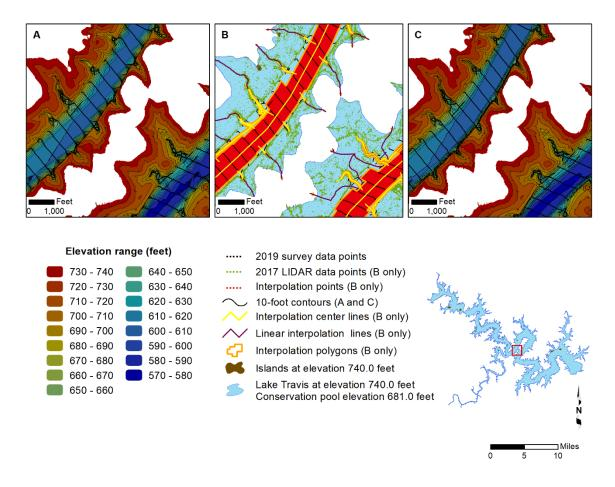
Figure 3. Anisotropic spatial interpolation as applied to Lake Travis sounding data; A) bathymetric contours without interpolated points, B) sounding points (*black*) and interpolated points (*red*), C) bathymetric contours with interpolated points.
