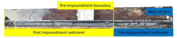
Figure 7. Sediment core LT-6. Post-impoundment sediment layers occur in the top 80.0 inches of this sediment core (identified by the yellow box). Pre-impoundment sediment layers were identified and are defined by the blue box.
