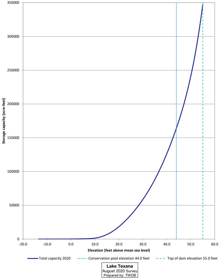
Appendix O: 2020 Bathymetric and topographic capacity curve
