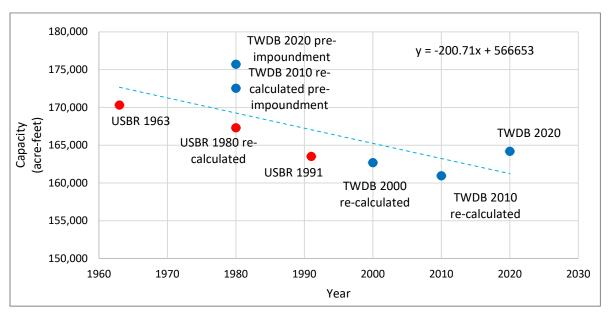
Figure 10. Plot of current and previous capacity estimates (acre-feet). Capacity estimates for each TWDB survey plotted as blue dots and other surveys as red dots. The blue trend line illustrates the total average loss of capacity through 2020.
