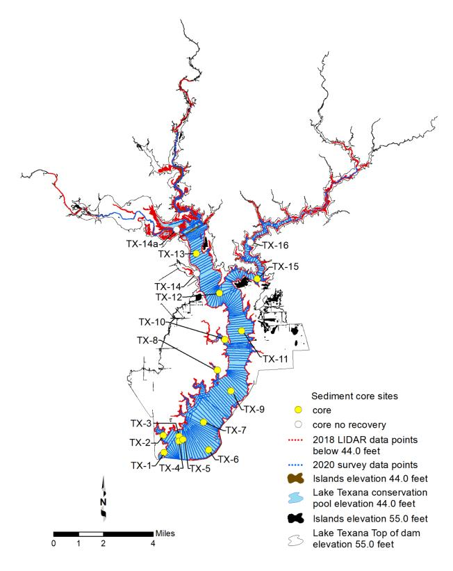
Figure 2. 2020 TWDB sounding data (*blue dots*), sediment coring locations (*yellow circles*), and 2018 LIDAR data for bathymetric model (*red dots*).
