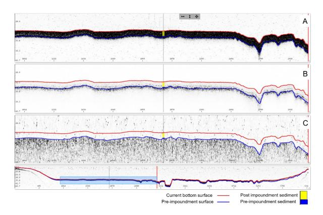
Figure 8. Sediment core sample TX-5 compared with acoustic signal returns. A) 208 kHz frequency, B) 50 kHz frequency, and C) 12 kHz frequency.
