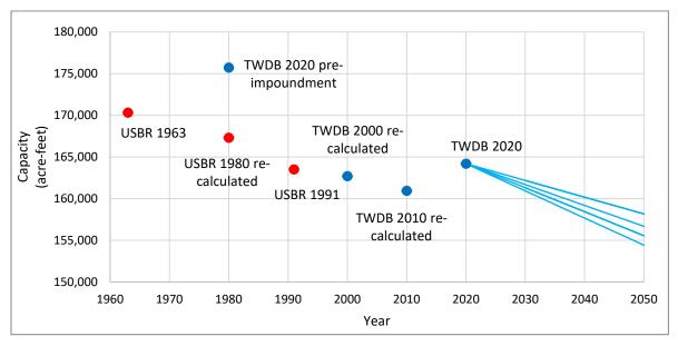
Figure 12. Plot of current and previous capacity estimates (acre-feet) with projected future capacity trends. Capacity estimates for each TWDB survey plotted as blue dots and other surveys as red dots. Future capacity projections from Table 5 shown as light blue lines. The top light blue line represents capacity loss at 200.71 acre-feet per year, while the bottom light blue line represents capacity loss at 325.65 acre-feet per year.
