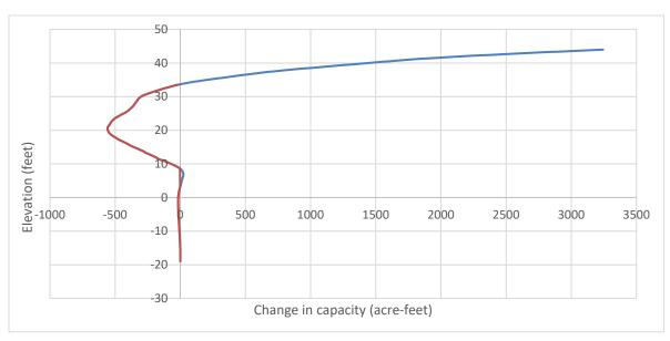
Figure 11. Change in capacity of Lake Texana between TWDB 2020 and 2010 surveys. The red segments show elevations where capacity decreased since 2010. The blue segments show elevations where capacity increased since 2010. Capacity loss due to sedimentation is occurring below elevation 33.6 feet. Capacity gain above elevation 33.6 feet is largely a result of increased data coverage in the 2020 survey and LIDAR data coverage.
