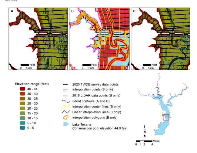
Figure 3. Anisotropic spatial interpolation as applied to Lake Texana sounding data; A) bathymetric contours without interpolated points, B) sounding points (*black*) and interpolated points (*red*), C) bathymetric contours with interpolated points.
