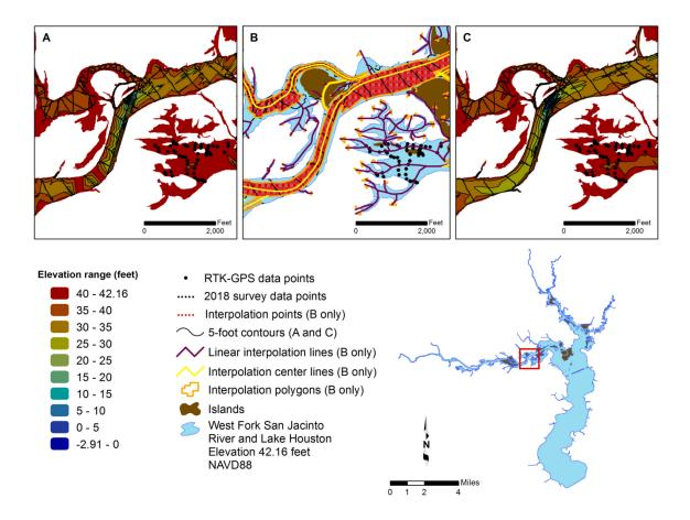
Figure 3. Anisotropic spatial interpolation and linear interpolation of the West Fork San Jacinto River sounding data; A) bathymetric contours without interpolated points, B) sounding points (*black*) and interpolated points (*red*), C) bathymetric contours with interpolated points.
