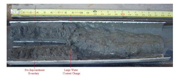
Figure D2 – Sediment Core R-3 from Richland-Chambers Reservoir, showing the preimpoundment boundary 3.5 inches above the base of the core (left). The preimpoundment boundary is marked by the change in sediment moisture content below and above the area 3.5 inches up from the core base. Above 8.5 inches from the core base, the sediment moisture content is extremely high.
