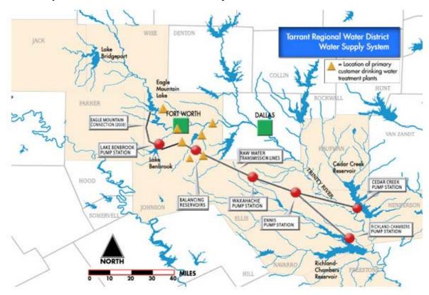
**Figure 2**. Tarrant Regional Water District Water Supply System and service area. Source: Tarrant Regional Water District, Pipeline, 25 April 2008, http://www.trwd.com/prod/AboutUs\_Pipeline.asp, 2007.
