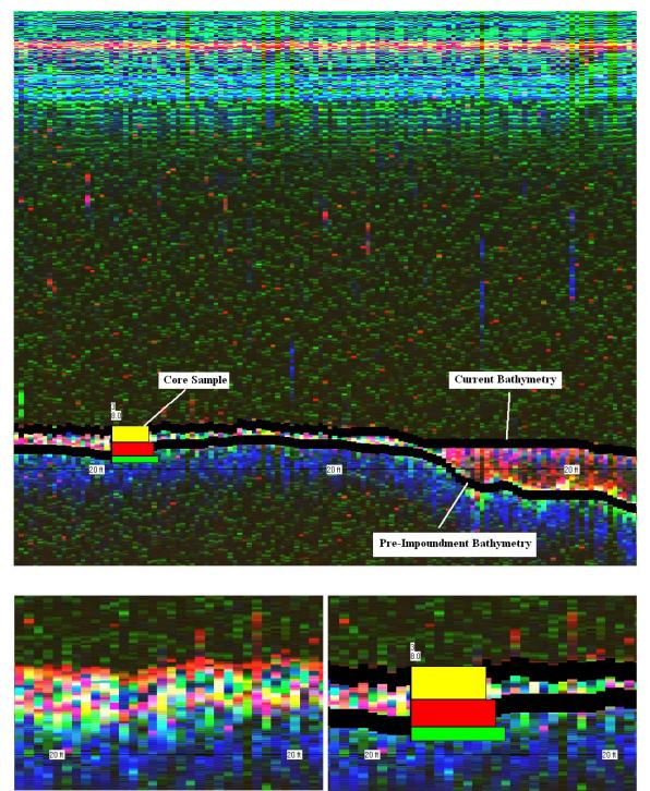
*Figure D3 – DepthPic and core sample use in identifying the pre-impoundment bathymetry.*
