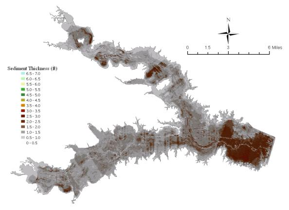
*Figure D4 - Sediment thicknesses in Richland-Chambers Reservoir derived from multifrequency sounding data.*
