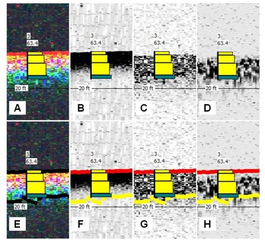
Figure 8. Comparison of sediment core P-3 with acoustic signal returns A,E) combined acoustic signal returns, B,F) 200 kHz frequency, C,G) 50 kHz frequency, D,H) 24 kHz frequency
