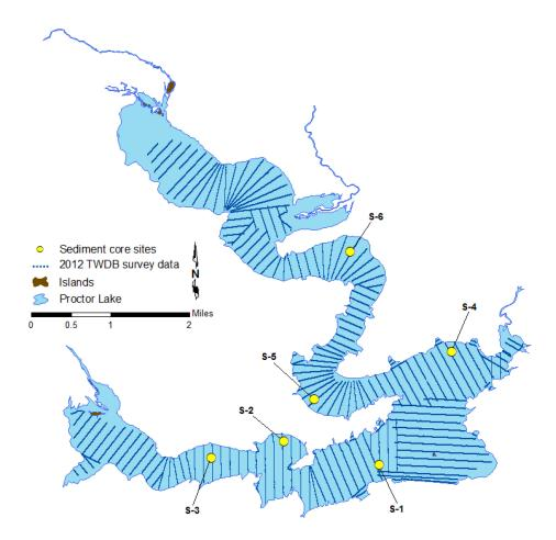
Figure 2. Data collection during 2012 TWDB Proctor Lake survey
