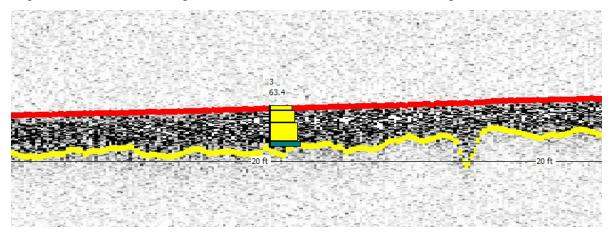
Figure 9. Cross-section of data collected during 2012 survey, displayed in DepthPic<sup>®</sup> (50 kHz frequency), correlated with sediment core sample P-3 and showing the current surface in red and pre-impoundment surface in yellow
