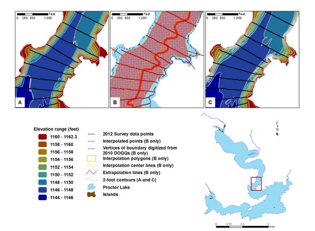
Figure 3. Anisotropic spatial interpolation and linear extrapolation of Proctor Lake sounding data -A) bathymetric contours without interpolated points, B) sounding points (black) and interpolated points (red), C) bathymetric contours with the interpolated points
