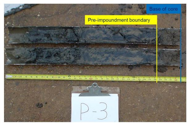
Figure 7. Sediment core P-3 from Proctor Lake
