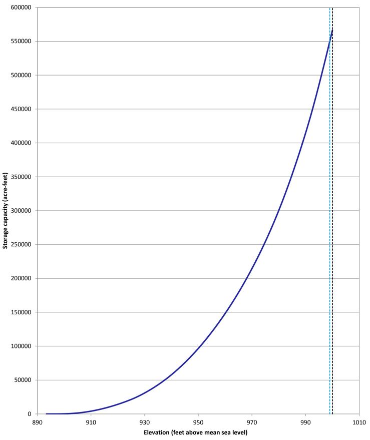
Total capacity 1994 ----- Normal operating level 999.0 feet ----- Top of gates/Emergency spillway elevation 1,000.0 feet
