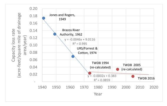
Figure 12. Plot of average annual capacity loss rates (acre-feet per square mile of drainage per year) for Possum Kingdom Lake. Capacity loss rates 1974 and earlier shown as blue dots, and capacity loss rates since 1974 shown as red dots. Blue and red trend lines illustrate a shift in rates of capacity loss before and after 1974.
