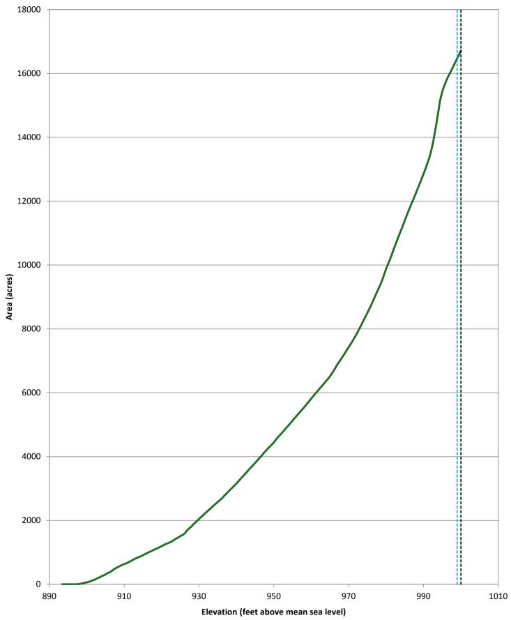
Total area 2005 ----- Normal operating level 999.0 feet ----- Top of gates/Emergency spillway elevation 1,000.0 feet
