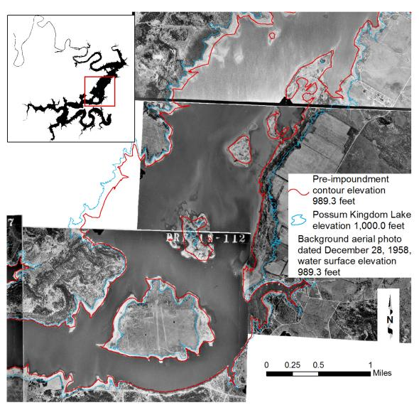
Figure 16. The TWDB surveyed pre-impoundment contour at elevation 989.3 feet (*red line*) overlain on an aerial photograph taken on December 28, 1958, while the daily average water surface elevation measured 989.3 feet. The current 1,000-foot contour is shown in blue.
