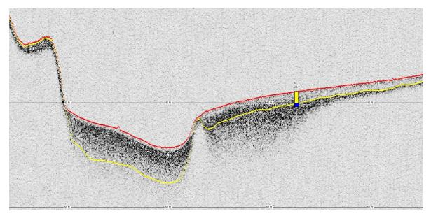
Figure 9. Cross-section of data collected during the 2016 survey, displayed in DepthPic<sup>®</sup> (50 KHz acoustic signal returns), correlated with sediment core sample PK-6 and showing the current surface as the top red line, and pre-impoundment surface as the bottom yellow line.
