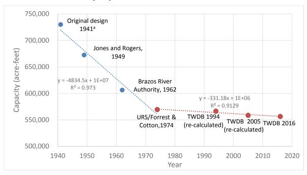
Figure 11. Plot of total capacity estimates at elevation 1,000.0 feet for Possum Kingdom Lake.
