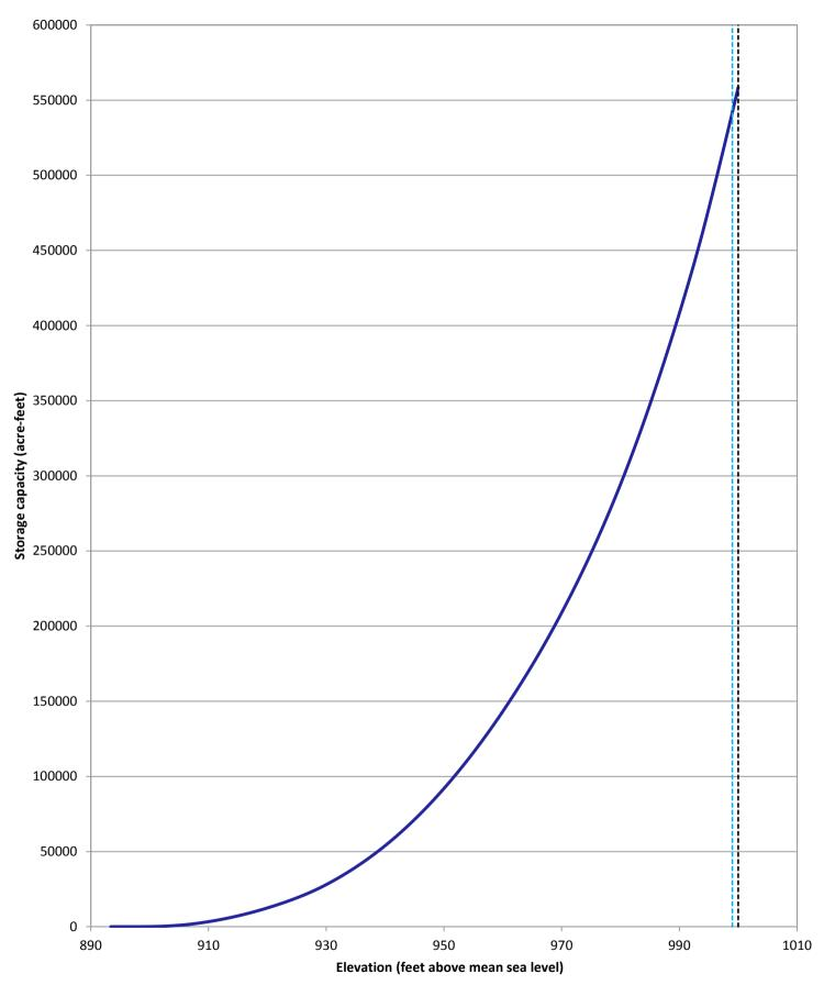
Total capacity 2005 ----- Normal operating level 999.0 feet ----- Top of gates/Emergency spillway elevation 1,000.0 feet
