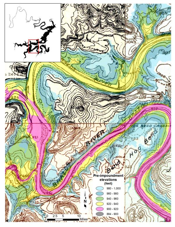
Figure 14. The TWDB surveyed pre-impoundment surface at 20-foot increments overlain on the USGS 1924 contour maps with a contour interval of 20 feet (solid lines, with some 10-foot contours shown as dashed lines).
