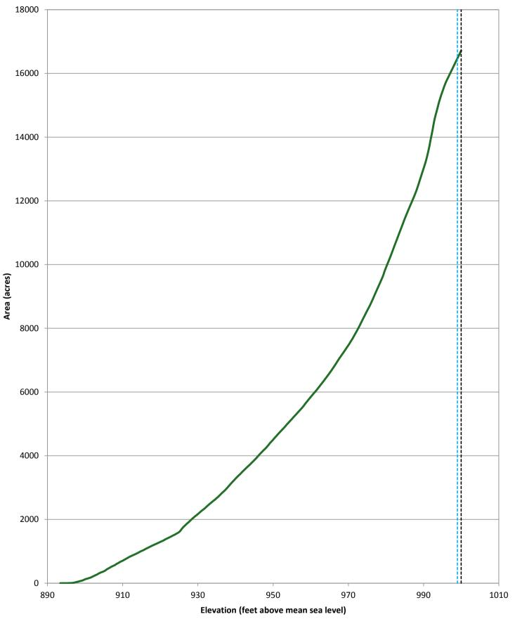
Total area 1994 ----- Normal operating level 999.0 feet ----- Top of gates/Emergency spillway elevation 1,000.0 feet
