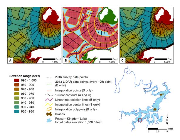
Figure 3. Anisotropic spatial interpolation and linear interpolation of Possum Kingdom Lake sounding data; A) bathymetric contours without interpolated points, B) sounding points (black) and interpolated points (red), C) bathymetric contours with interpolated points.
