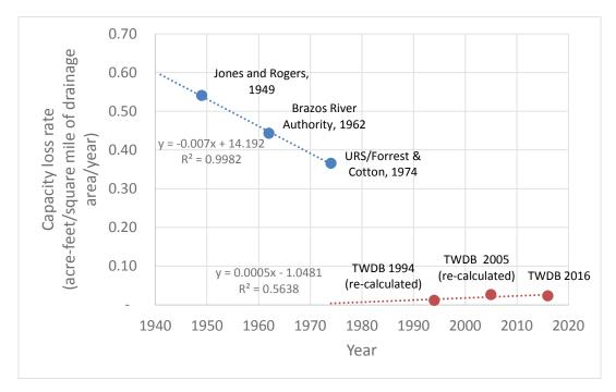
Figure 13. Plot of capacity loss rates (acre-feet per square mile of drainage per year) before and after 1974 for Possum Kingdom Lake. Capacity loss rates dated 1974 and earlier shown as blue dots, and capacity loss rates after 1974 shown as red dots. Blue and red trend lines illustrate a shift in rates of capacity loss before and after 1974.
