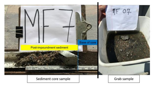
Figure 7. Sediment sample MF-7. In the sediment core on the left, the 8.5 inches of sediment was interpreted to be post-impoundment sediment (identified by the yellow box). Pre-impoundment sediment layers were not identified. Similar sediment was retrieved by the grab sample as seen on the right.
