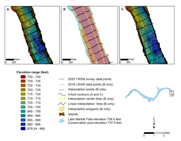
Figure 3. Anisotropic spatial interpolation as applied to Lake Marble Falls sounding data; A) bathymetric contours without interpolated points, B) sounding points (*black*) and interpolated points (*red*), C) bathymetric contours with interpolated points.
