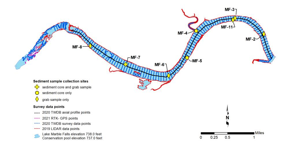
Figure 2. 2020 TWDB Lake Marble Falls survey data (*blue dots*), RTK-GPS data (*pink dots*), sediment sampling locations (*yellow shapes*), and 2019 LIDAR data (*red dots*)
