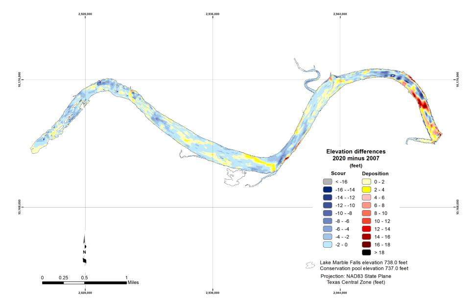
Figure 11. Bathymetric differences between 2020 and 2007 bottom surfaces
