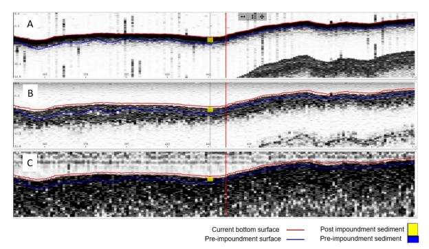
Figure 8. Sediment core sample MF-7 compared with acoustic signal returns. A) 208 kHz frequency, B) 50 kHz frequency, and C) 12 kHz frequency.
