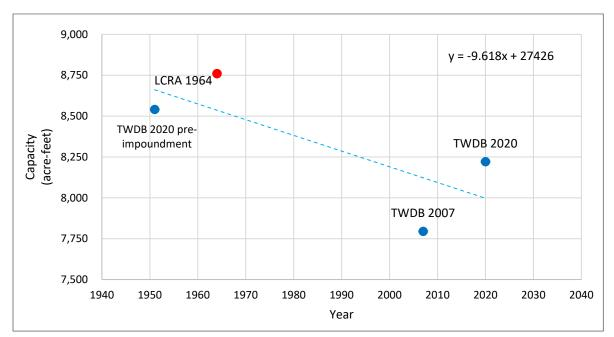
Figure 10. Plot of current and previous capacity estimates (acre-feet) at elevation 738.00 feet for Lake Marble Falls. Capacity estimates for each TWDB survey plotted as blue dots and other surveys as red dots. The blue trend line illustrates the total average loss of capacity through 2020.
