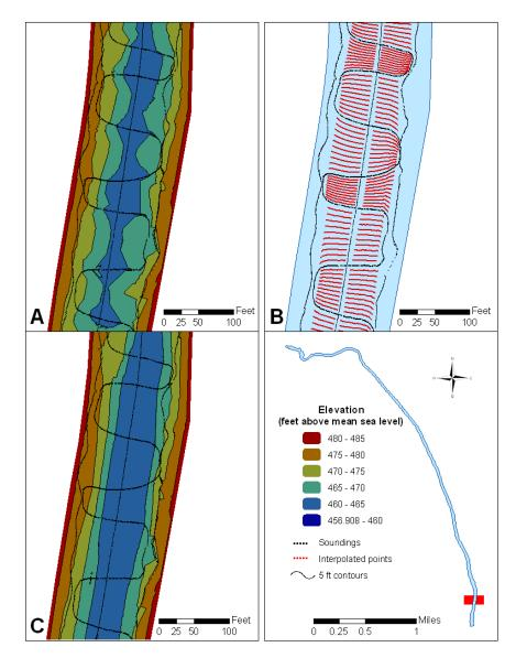
Figure 10.Application of the self-similar interpolation technique to the Leon River sounding<br/>data – A) bathymetric contours without interpolated points, B) sounding points<br/>(black) and interpolated points (red) with reservoir boundary shown at elevation<br/>481.97 feet, C) bathymetric contours with the interpolated points.
