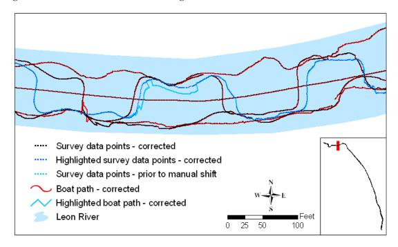
Figure 4. Illustration of how survey data were corrected using an estimated boat path and manually moving other sections of data.
