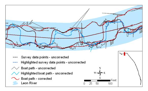
Figure 3. Illustration of how DGPS signal loss affects the data.
