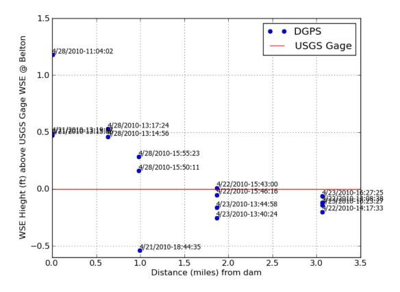
Figure 7. Water surface elevations relative to the gage water surface elevation.
