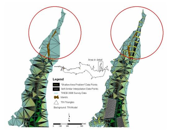
**Figure 7**. The image on the left illustrates how triangles form during the TIN generation process without the Self-Similar and "Shallow Area Problem" data points. The red circle highlights those triangles where all three vertices are on the boundary, creating flat triangles. The image on the right illustrates how the TIN triangles are formed after the Self-Similar and "Shallow Area Problem" data points are added. Notice the flat triangles no longer exist.
