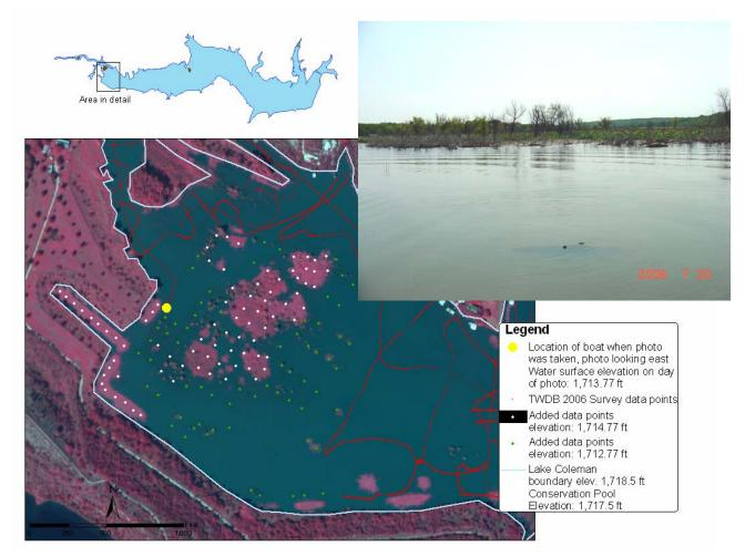
**Figure 8**. Illustrates the methodology used to determine depths/ elevations for an area of the reservoir that was too shallow to navigate by boat. A combination of photographs, such as the one shown here, and field observations were used to estimate the elevations of these additional data points.
