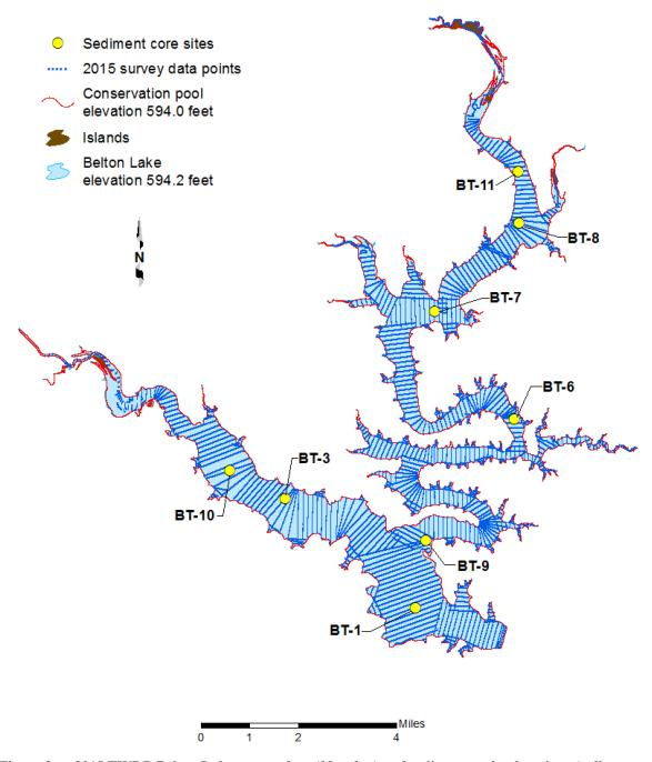
Figure 2. 2015 TWDB Belton Lake survey data (*blue dots*) and sediment coring locations (*yellow circles*).
