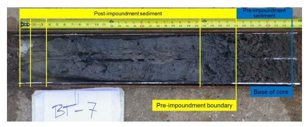
Figure 7. Sediment core BT-7 from Belton Lake. Post-impoundment sediment layers occur in the top 28 inches of this sediment core (identified by yellow boxes). Pre-impoundment sediment layers were identified and are defined by the blue box.
