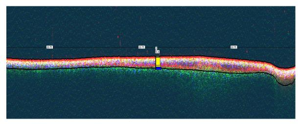
Figure 9. Cross-section of data collected during the 2015 survey, displayed in DepthPic© (combined acoustic signal returns), correlated with sediment core sample BT-7 and showing the current surface as the top black line, and pre-impoundment surface as the bottom black line.
