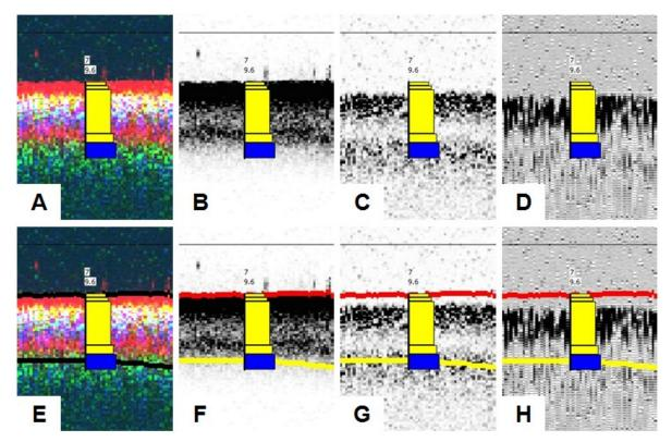
Figure 8. Comparison of sediment core BT-7 with acoustic signal returns A, E) combined acoustic signal returns, B, F) 208 kHz frequency, C, G) 50 kHz frequency, and D, H) 24 kHz frequency.
