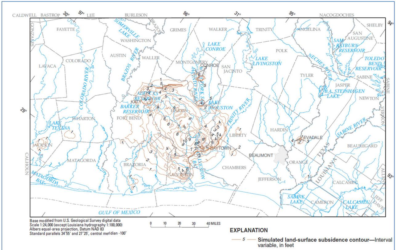
**Figure 6-16. Simulated 2010 land-surface subsidence in the northern portion of the Gulf Coast Aquifer System groundwater availability model area (from Kasmarek and others, 2005).**
