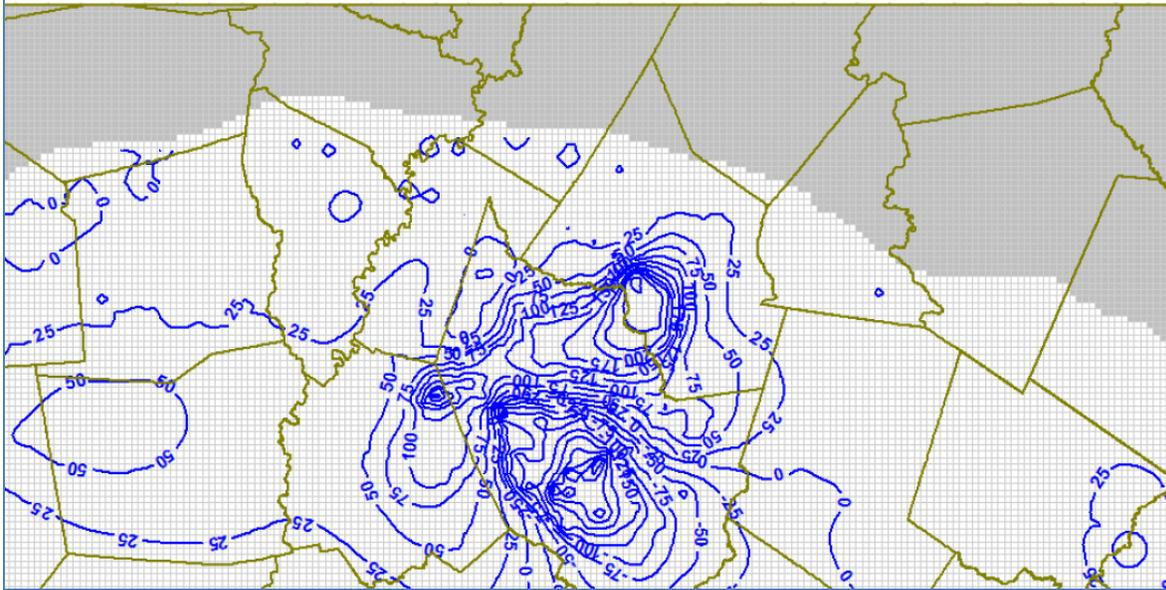
**Figure 6-3. Cumulative drawdown (through 2009) in the Evangeline Aquifer (from Groundwater Management Area 14, 2016; Appendix J)**
