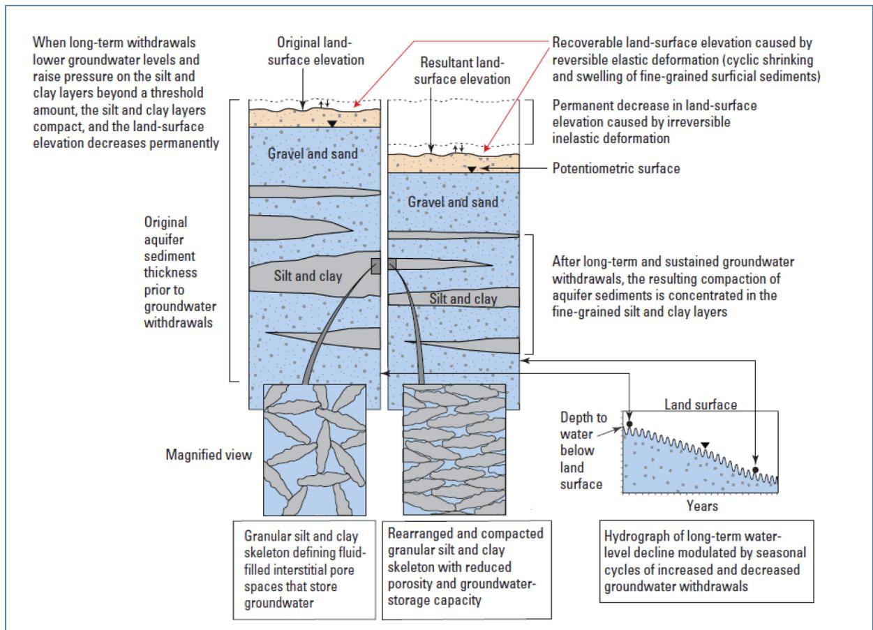
**Figure 6-14. Mechanism of subsidence (from Kasmarek and others, 2015).**
