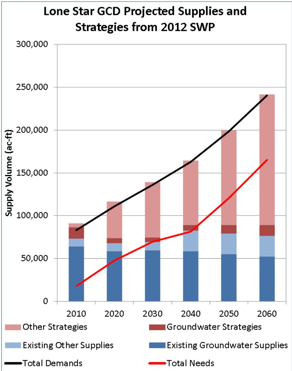
**Figure 6-5. Graph of projected supplies and strategies from the 2012 State Water Plan (from Groundwater Management Area 14, 2016; Appendix I)**
