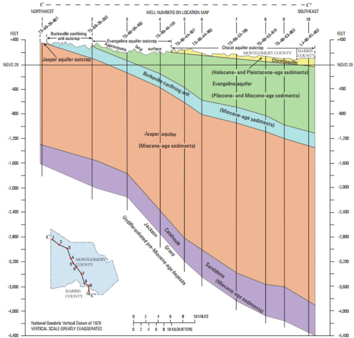
**Figure 3-3. Cross-Section of Gulf Coast Aquifer System in Montgomery County (from Kasmarek and others, 2016).**
