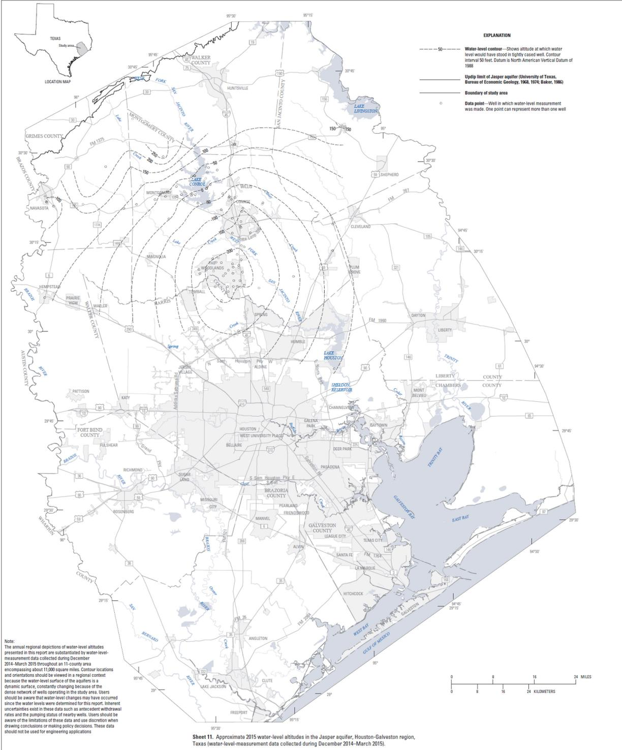
**Figure 6-8. Potentiometric surface map for the Jasper Aquifer (from Kasmarek and others, 2015).**
