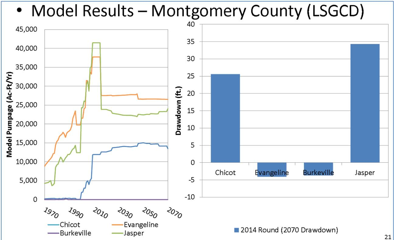
Figure 6-12. Modeled pumping rates for Montgomery County from 1970 through 2070 in the Chicot, Evangeline, and Jasper aquifers (from Mullican and Associates, 2015).
