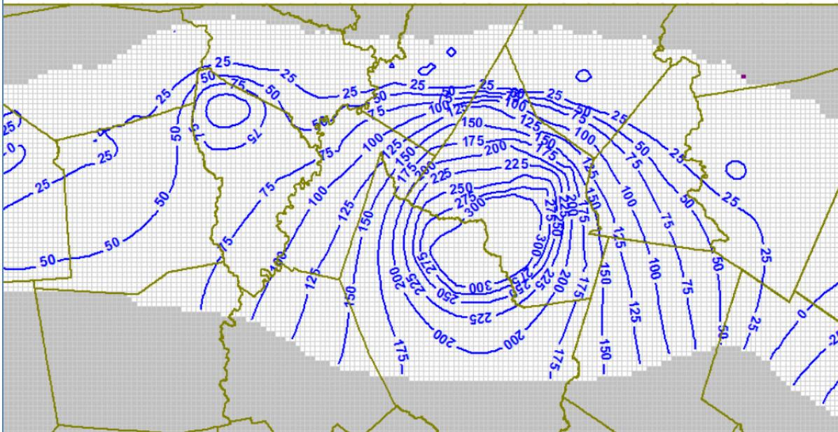
**Figure 6-4. Cumulative drawdown (through 2009) in the Jasper Aquifer (from Groundwater Management Area 14, 2016; Appendix J)**
