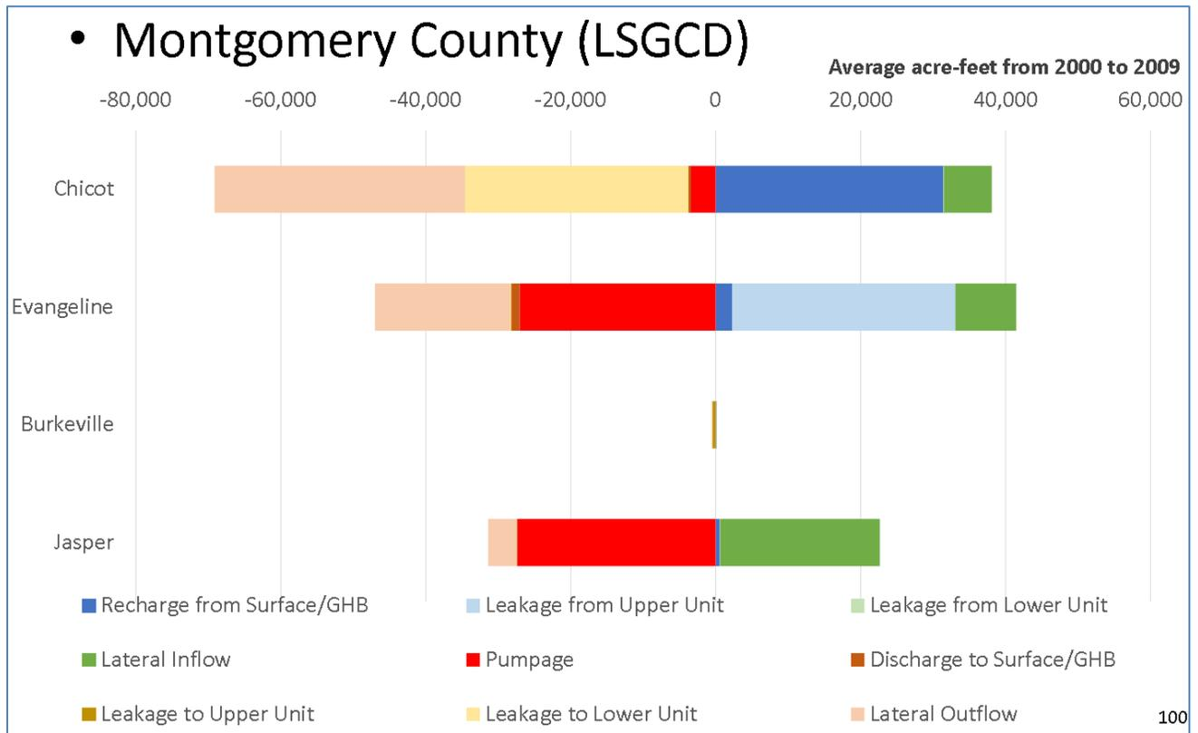
**Figure 6-11. Modeled water budget for Montgomery County (from Groundwater Management Area 14, 2016; Appendix J).**
