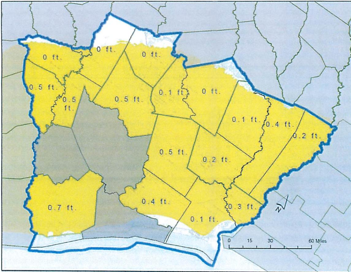
Figure 5-24 – County average subsidence results from Northern Gulf Coast GAM Run 2 using SUB package for predictive period of 2010-2070<sup>71</sup>
