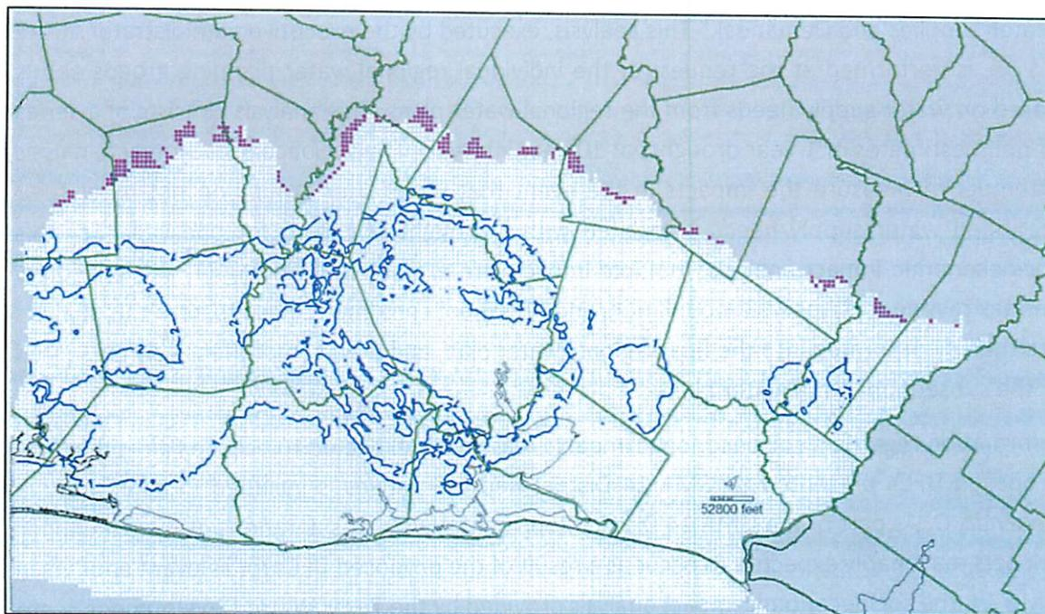
Figure 5-25 – Contours of subsidence from Northern Gulf Coast GAM Run 2 using SUB package for predictive period of 2010-2070.
