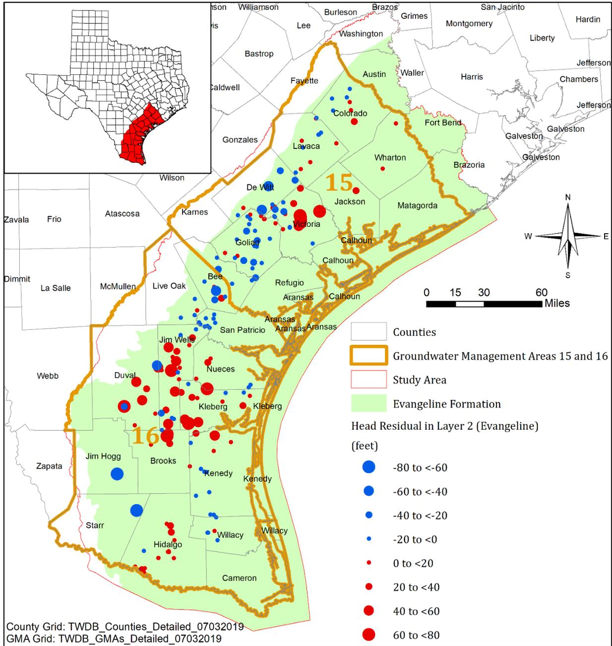
**Figure 3.2.7** Distribution of average head residuals (simulated minus measured) in the Evangeline Aquifer (Layer 2). Negative (positive) values indicate that the simulated head is greater (lesser) than the measured head.
