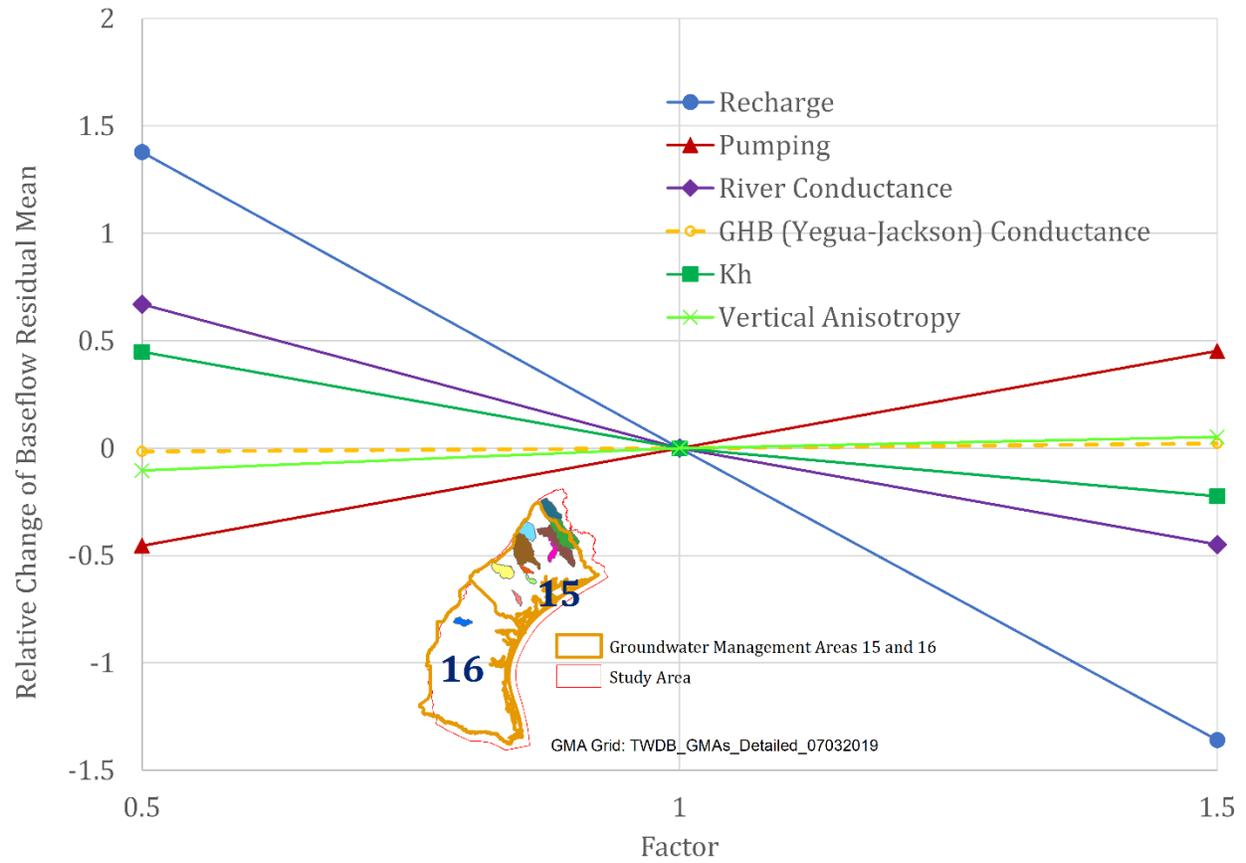
**Figure 4.1.2** Sensitivity of stream baseflow to model input parameters. The inset map shows the locations of river basins.
