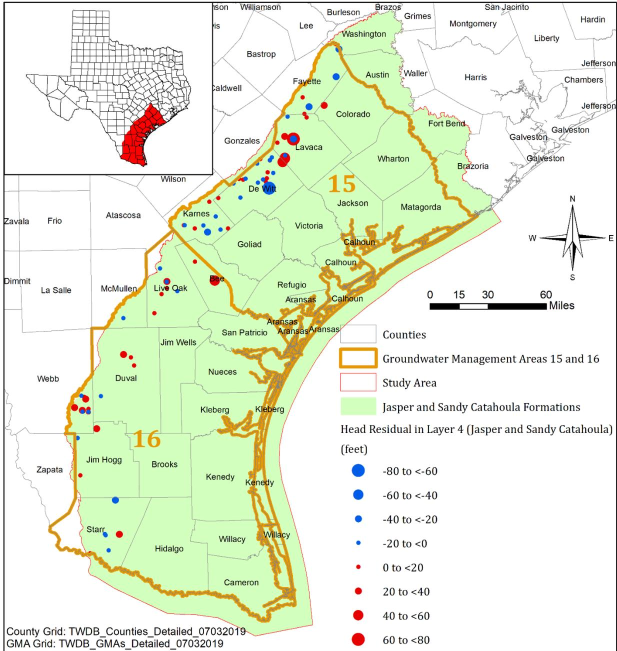
**Figure 3.2.9** Distribution of average head residuals (simulated minus measured) in the Jasper Aquifer and sandy Catahoula Formation (Layer 4). Negative (positive) values indicate that the simulated head is greater (lesser) than the measured head.
