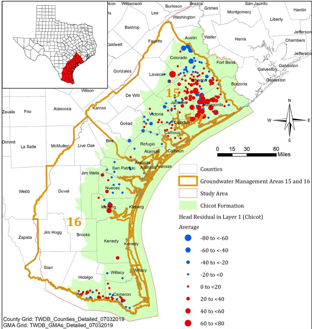
**Figure 3.2.6** Distribution of average head residuals (simulated minus measured) in the Chicot Aquifer (Layer 1). Negative (positive) values indicate that the simulated head is greater (lesser) than the measured head.
