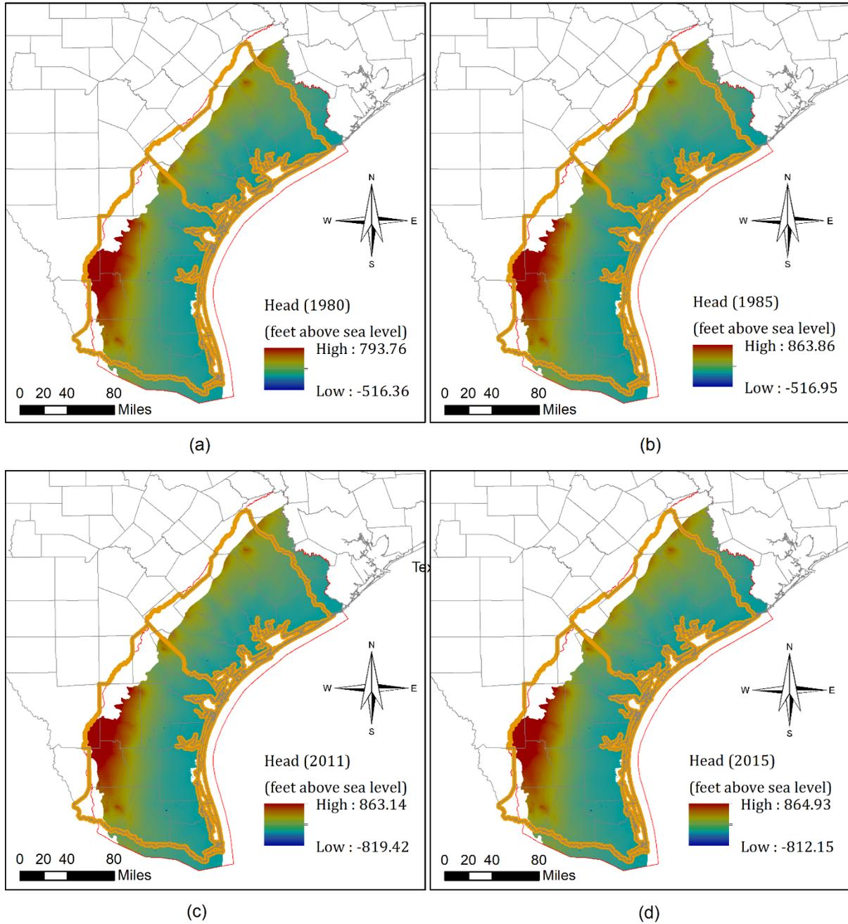
Figure 3.2.11 Simulated water-level elevations (hydraulic head) in the Evangeline Aquifer (Layer 2) for selected years: (a) 1980, (b) 1985, (c) 2011, and (d) 2015.
