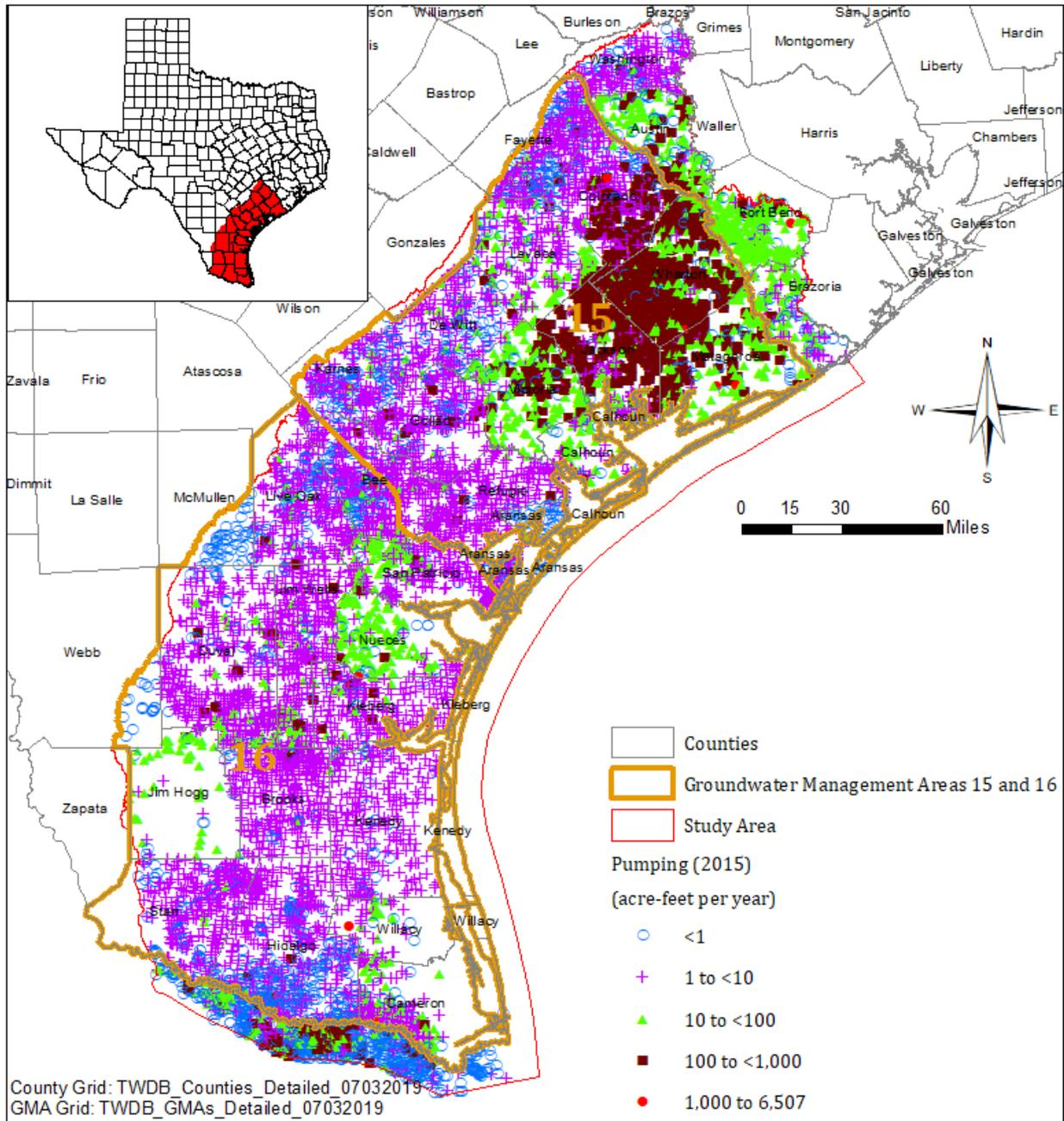
Figure 2.13.5 Simulated pumping in 2015 (a wet year).
