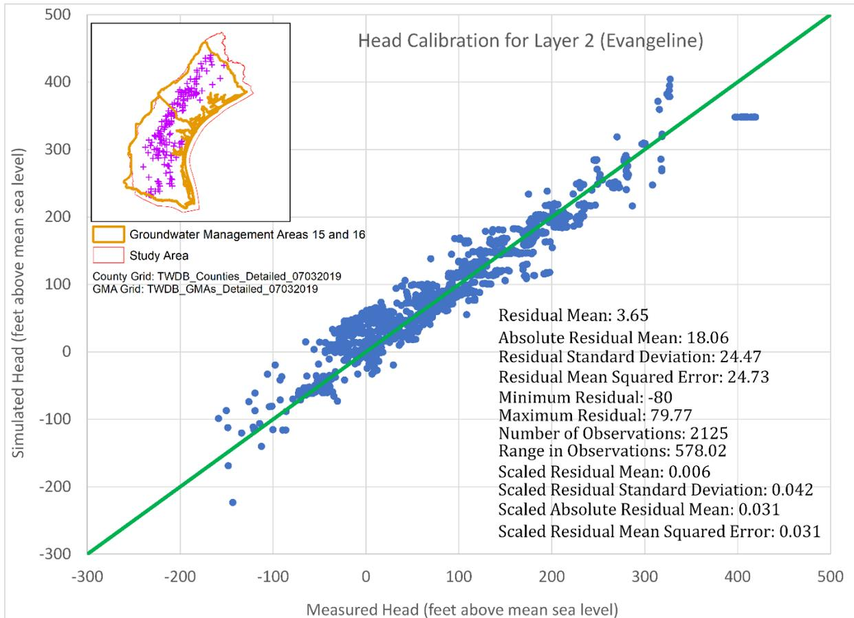
**Figure 3.2.3 Simulated versus observed hydraulic head and statistic summary in the Evangeline Aquifer (Layer 2).**
