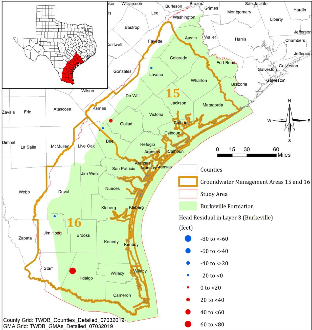
**Figure 3.2.8** Distribution of average head residuals (simulated minus measured) in the Burkeville Unit (Layer 3). Negative (positive) values indicate that the simulated head is greater (lesser) than the measured head.
