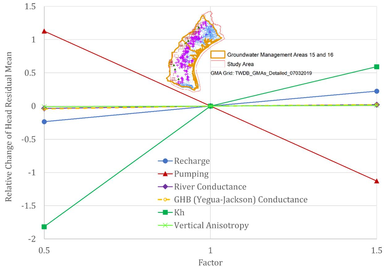
**Figure 4.1.1 Sensitivity of hydraulic head to model input parameters. The inset map shows the locations of water level targets.**
