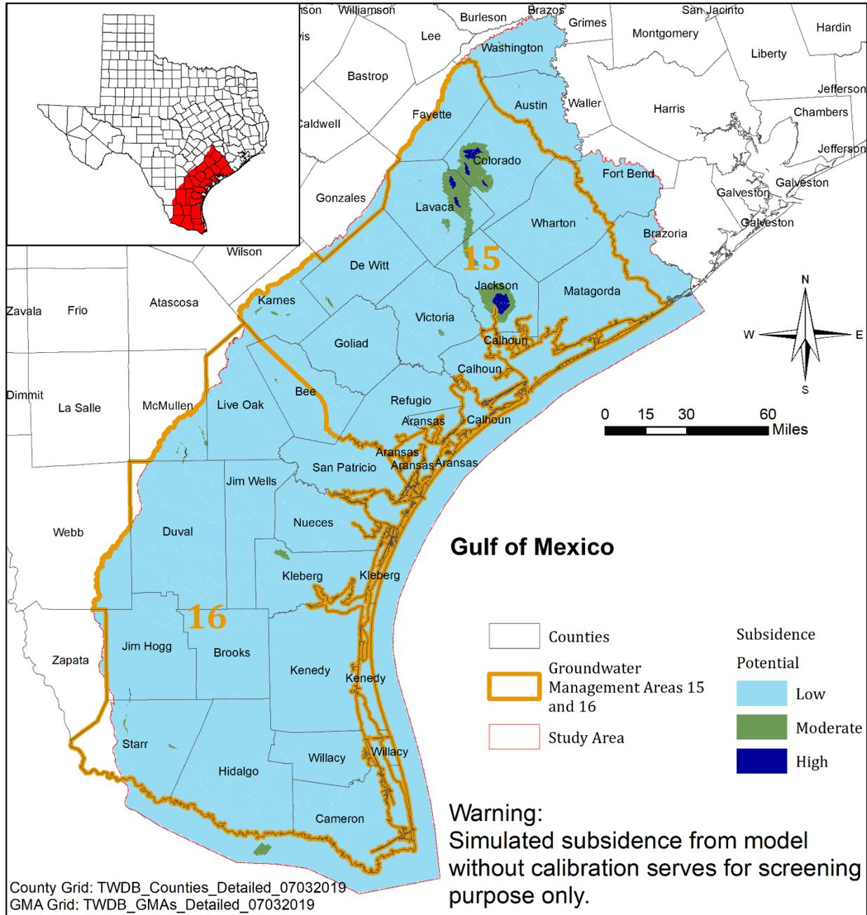
**Figure 3.5.1 Simulated subsidence of the Gulf Coast Aquifer System between 1981 and 2015.**
