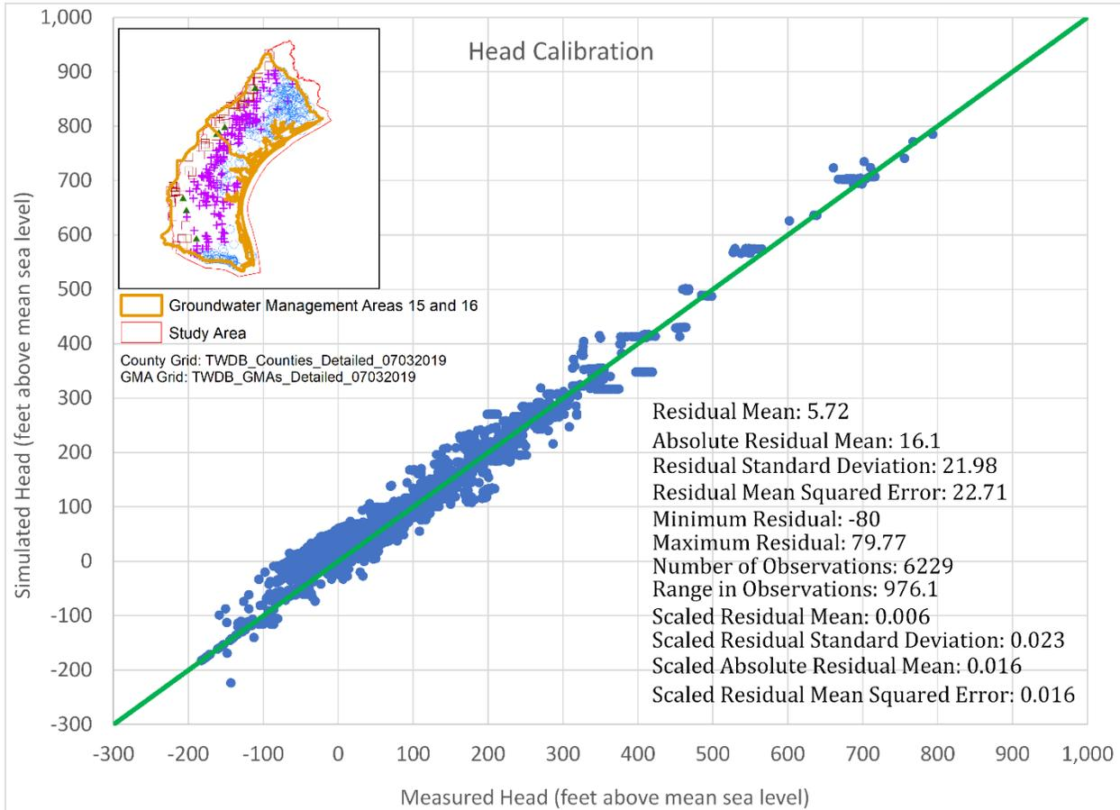
**Figure 3.2.1 Simulated versus observed hydraulic head and statistic summary in Chicot Aquifer (layer 1), Evangeline Aquifer (Layer 2), Burkeville Unit (Layer 3), and Jasper Aquifer (Layer 4).**
