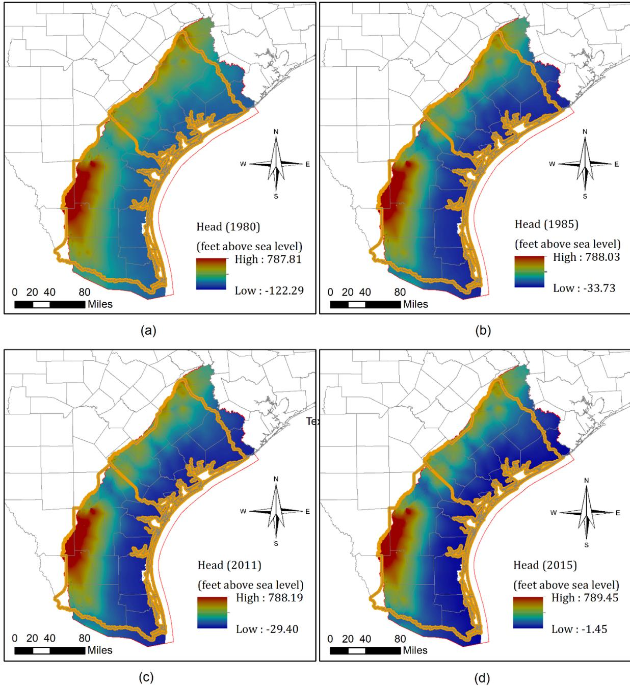
**Figure 3.2.13 Simulated water-level elevations (hydraulic head) in the Jasper Aquifer and sandy Catahoula Formation (Layer 4) for selected years: (a) 1980, (b) 1985, (c) 2011, and (d) 2015.**
