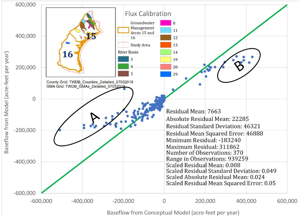
**Figure 3.3.1 Simulated versus calculated stream baseflow and statistic summary at selected river basins.**
