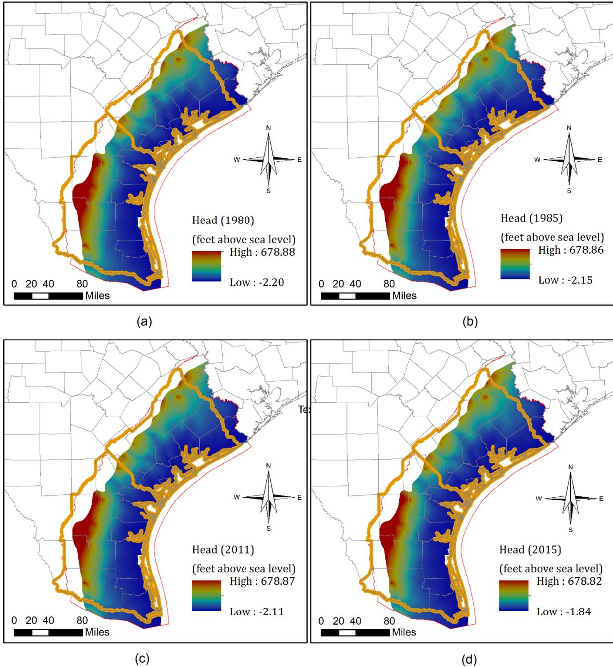
**Figure 3.2.12 Simulated water-level elevations (hydraulic head) in the Burkeville Unit (Layer 3) for selected years: (a) 1980, (b) 1985, (c) 2011, and (d) 2015.**
