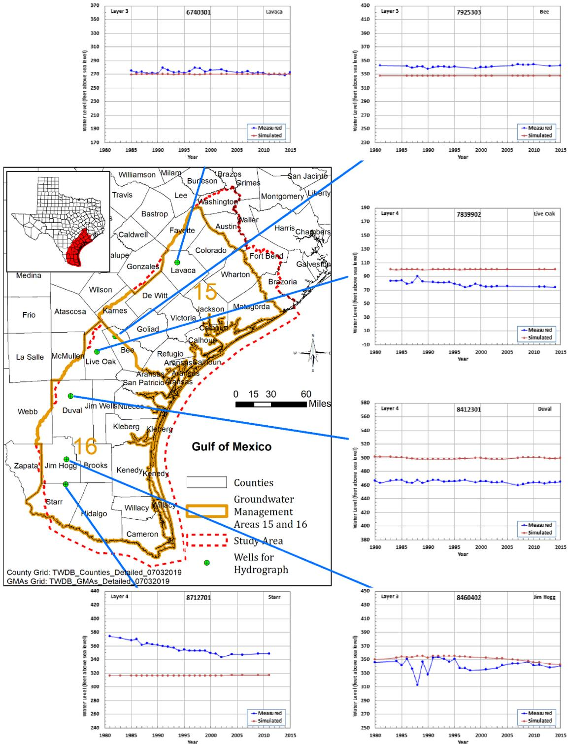
**Figure 3.2.19** Water level hydrographs at selected wells in the Burkeville Unit (Layer 3) and Jasper Aquifer (Layer 4) in Bee, Jim Hogg, Lavaca, Duval, Live Oak, and Starr counties.
