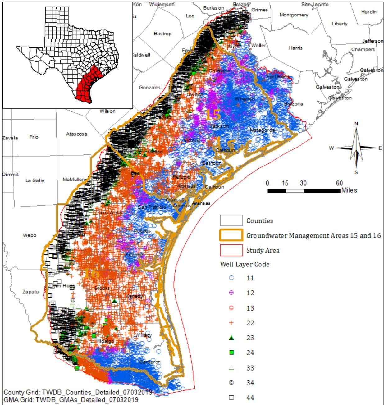
**Figure 2.13.1 Simulated pumping wells. Some wells were only active in certain years. Well layer code represents screened model layer(s). The first digit is the screened top layer and second the screened bottom layer.**
