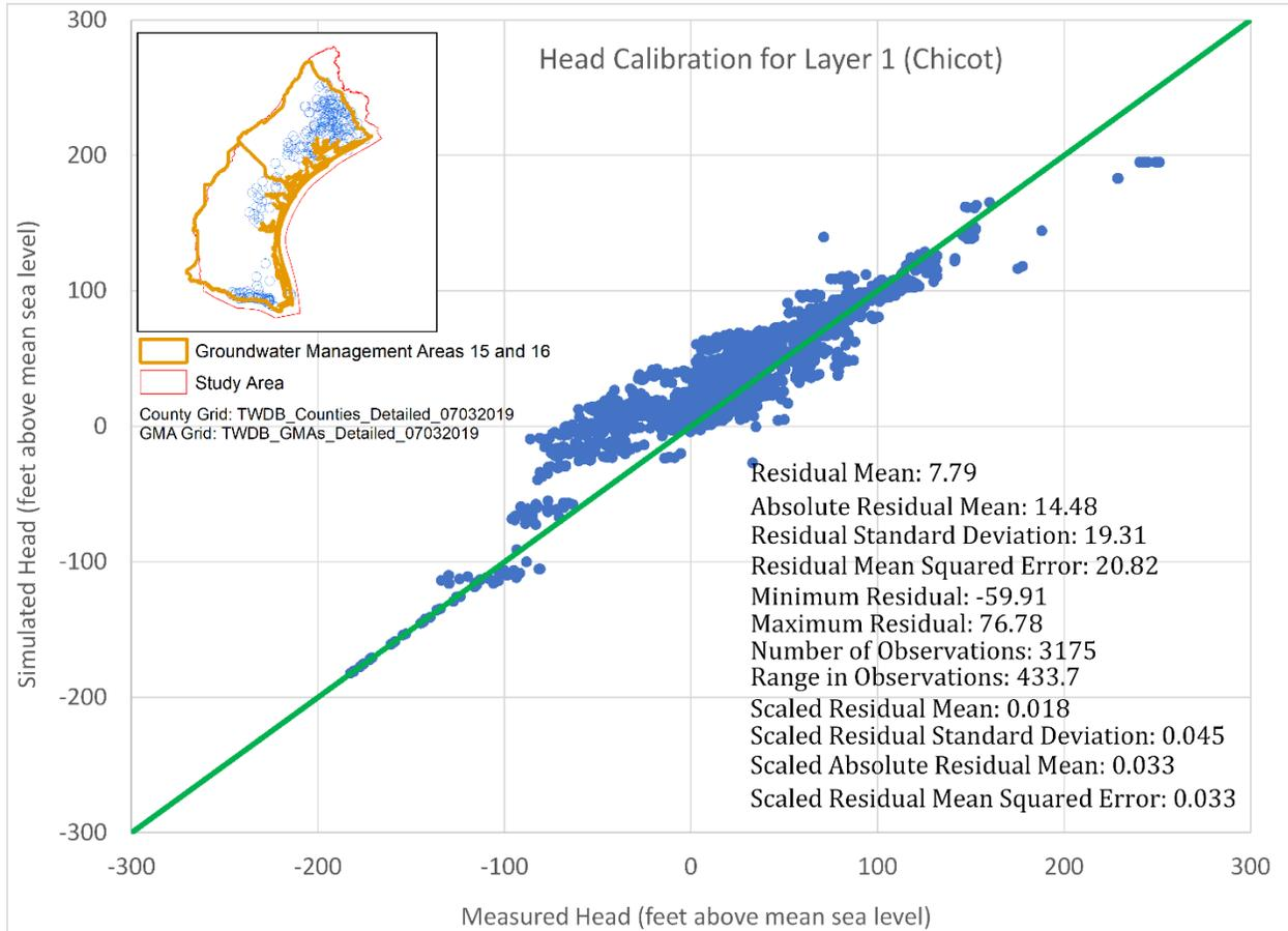
Figure 3.2.2 Simulated versus observed hydraulic head and statistic summary in the Chicot Aquifer (Layer 1).
