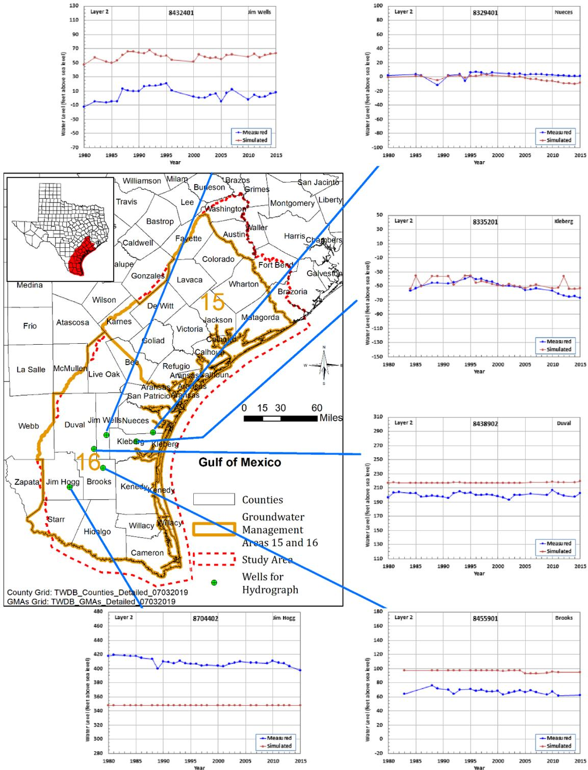
Figure 3.2.17 Water level hydrographs at selected wells in the Evangeline Aquifer (Layer 2) in Brooks, Duval, Jim Hogg, Jim Wells, Kleberg, and Nueces counties.
