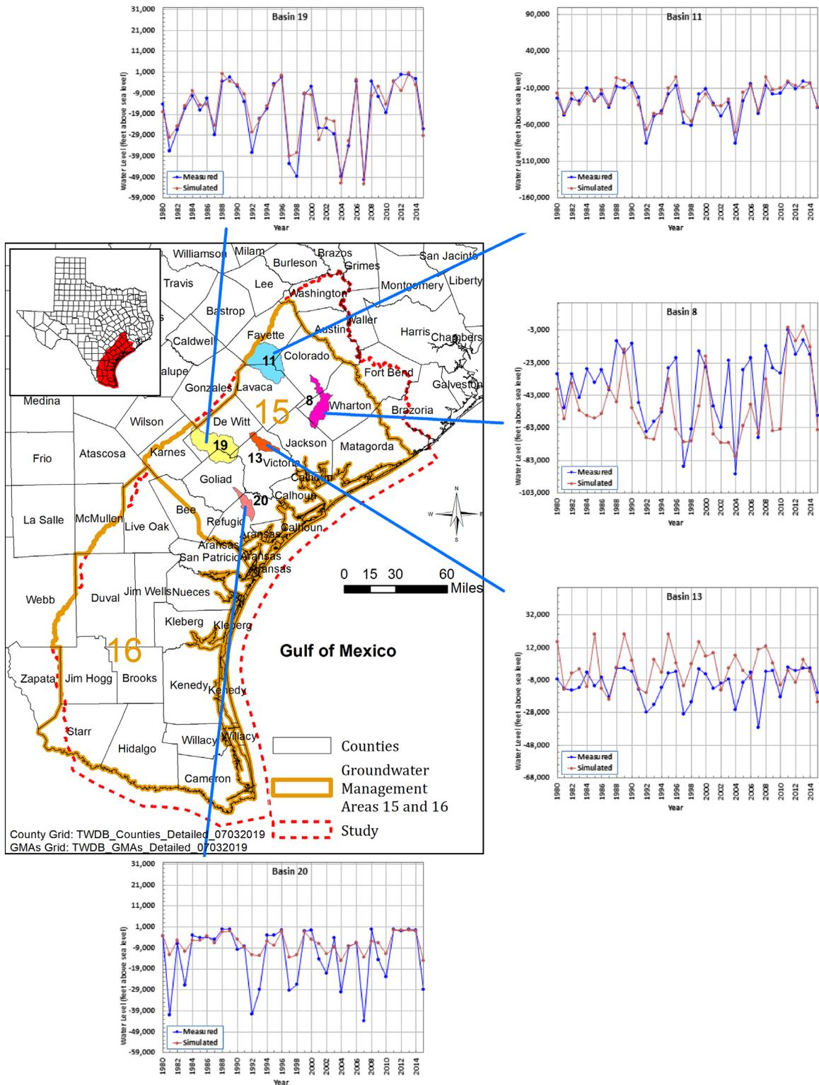
**Figure 3.3.3 Simulated versus calculated stream baseflow at river basins 8, 11, 13, 19, and 20.**
