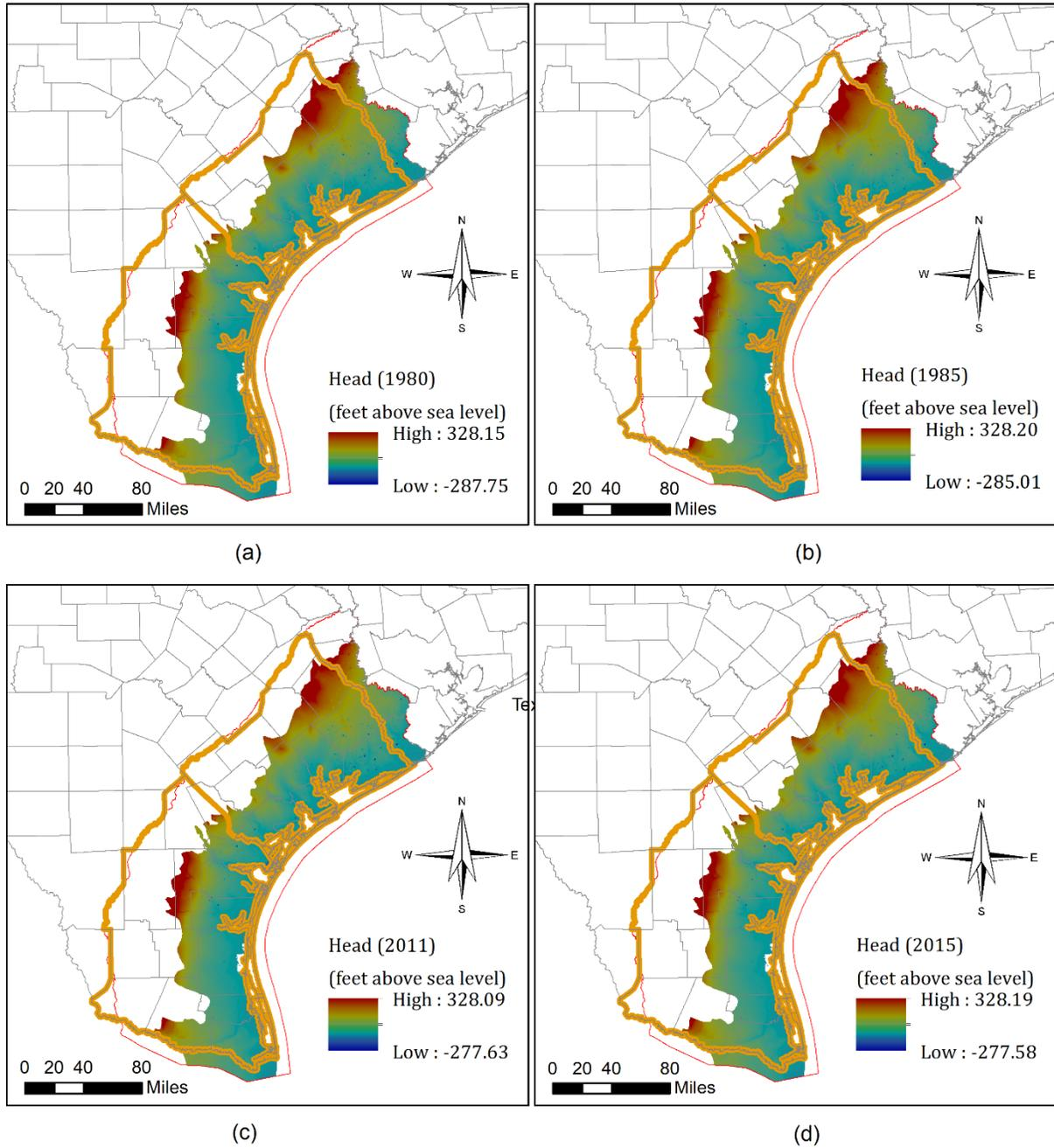
Figure 3.2.10 Simulated water-level elevations (hydraulic head) in the Chicot Aquifer (Layer 1) for selected years: (a) 1980, (b) 1985, (c) 2011, and (d) 2015.
