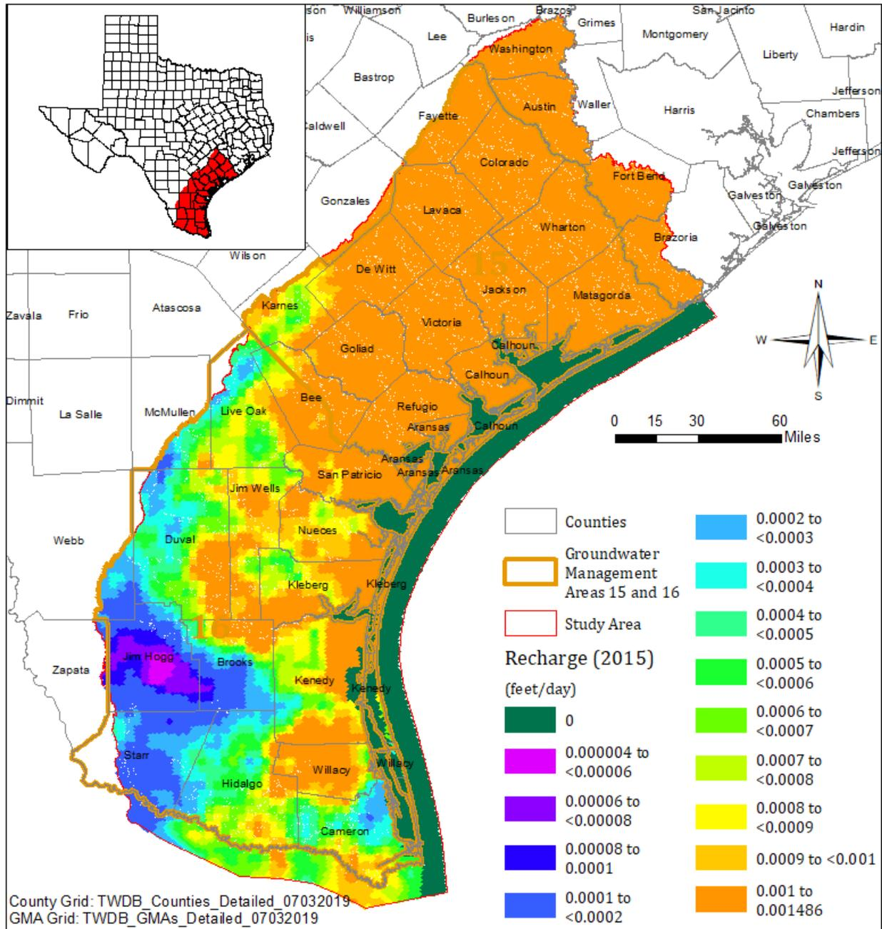
Figure 2.11.4 Calibrated groundwater recharge for 2015 (a wet year).
