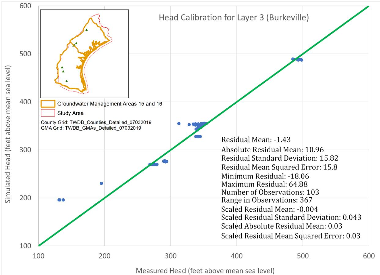
**Figure 3.2.4 Simulated versus observed hydraulic head and statistic summary in the Burkeville Unit (Layer 3).**
