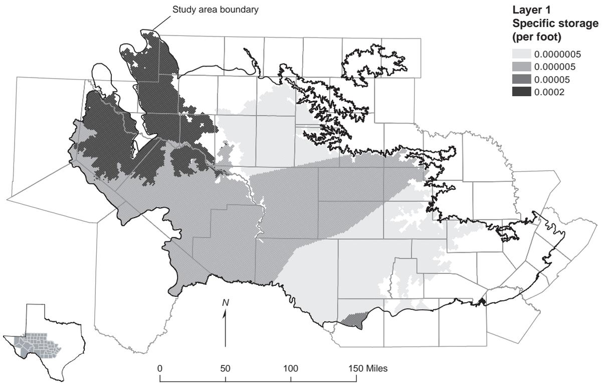
Figure 10-5. Specific storage for layer 1 used within model.
