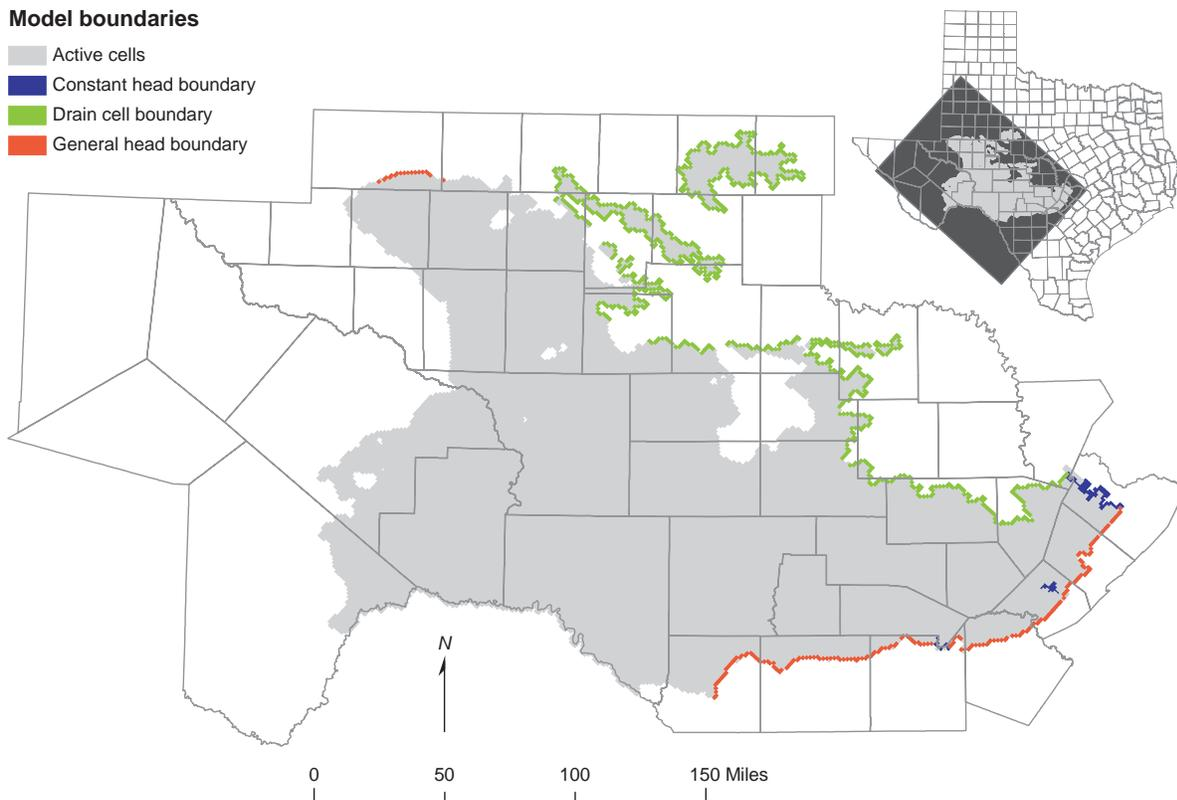
Figure 7-3. Boundary conditions for layer 2 used within model.
