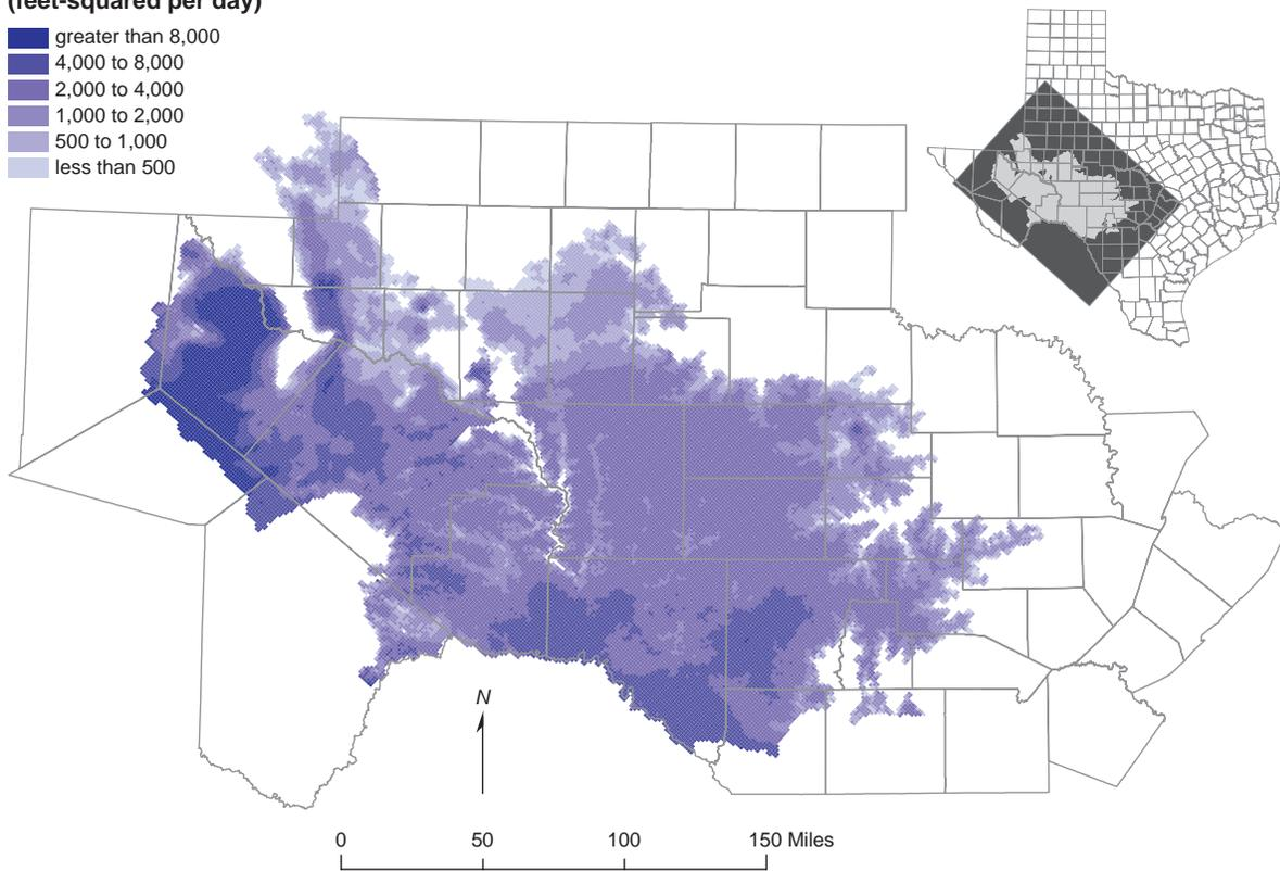
Figure 7-6. Transmissivity for layer 1 used within model.
