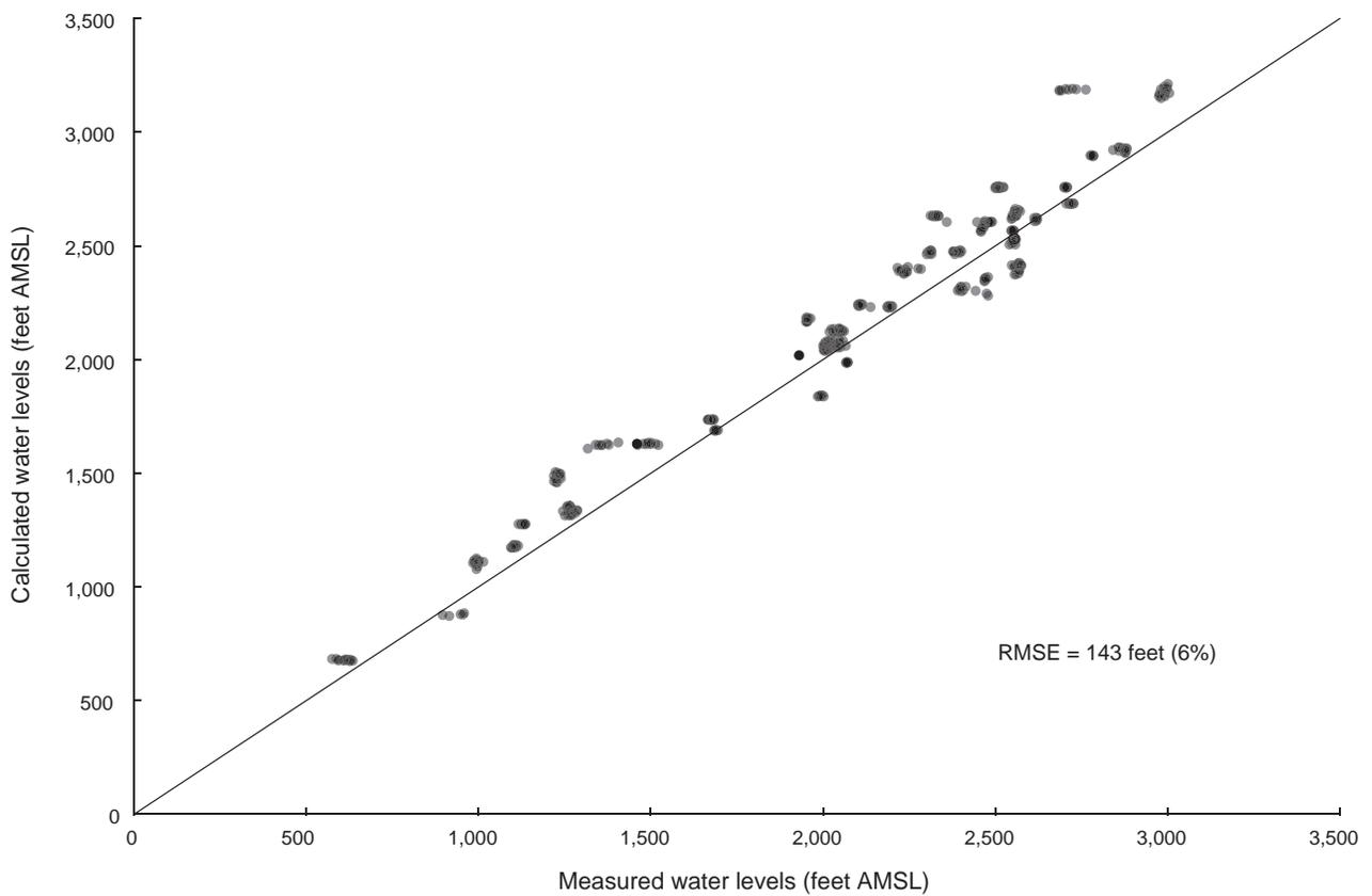
Figure 10-11. Cross plot comparison of simulated and measured water levels for both layers 1 and 2 of the (1980–2000) transient model.
