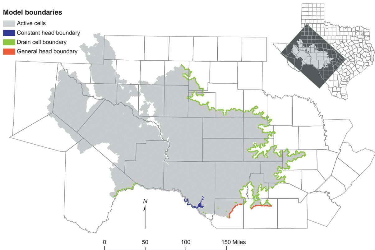
Figure 7-2. Boundary conditions for layer 1 used within model.
