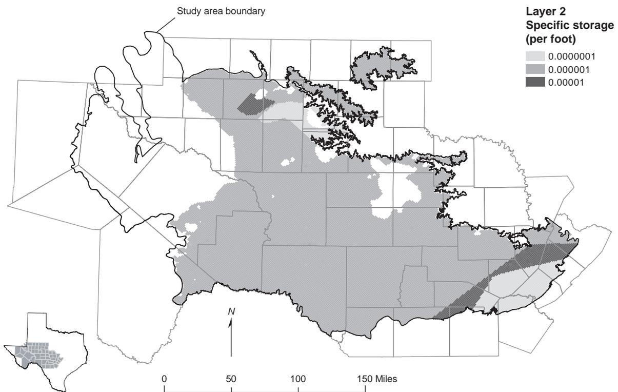
Figure 10-6. Specific storage for layer 2 used within model.
