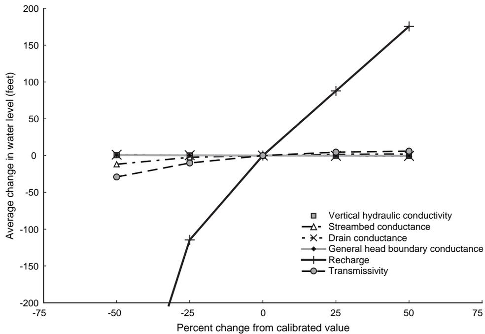
Figure 9-11. Sensitivity of numerically predicted water levels for 1980.
