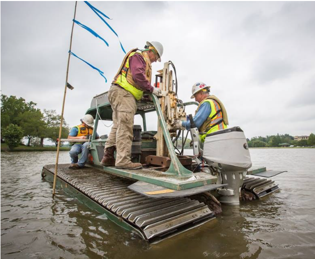
Figure 7-9. Examples of Geoprobe Rigs (provided courtesy of Vortex Drilling, Inc in San Antonio, Texas and Pro-Tech in Baton Rouge, Louisiana).
