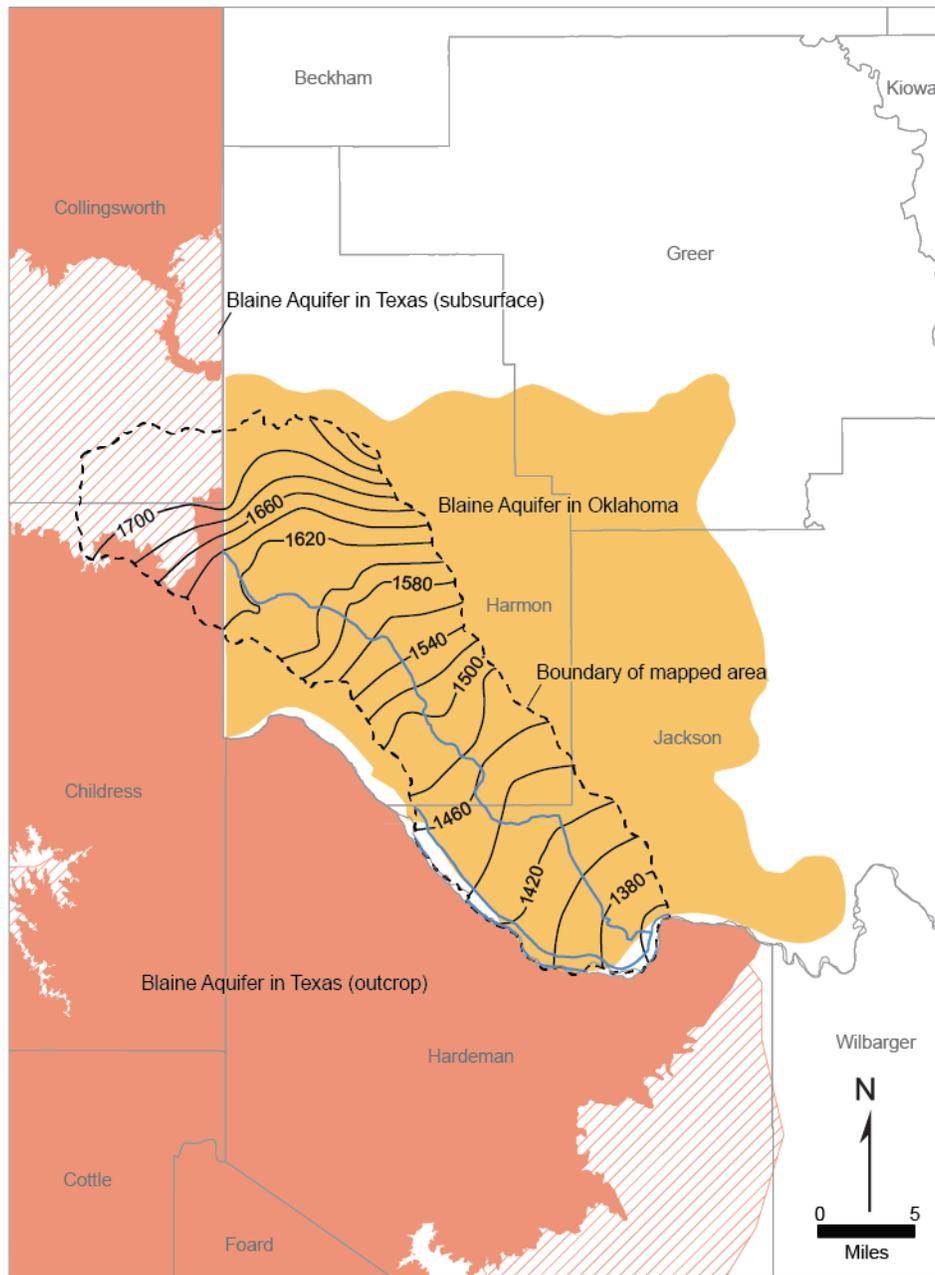
**Figure A2-3 Potentiometric surface of part of the Blaine Aquifer from wells measured in February 1994 (modified from Osborn and Others, 1997). Hydraulic heads elevations are shown in feet above mean sea level**
