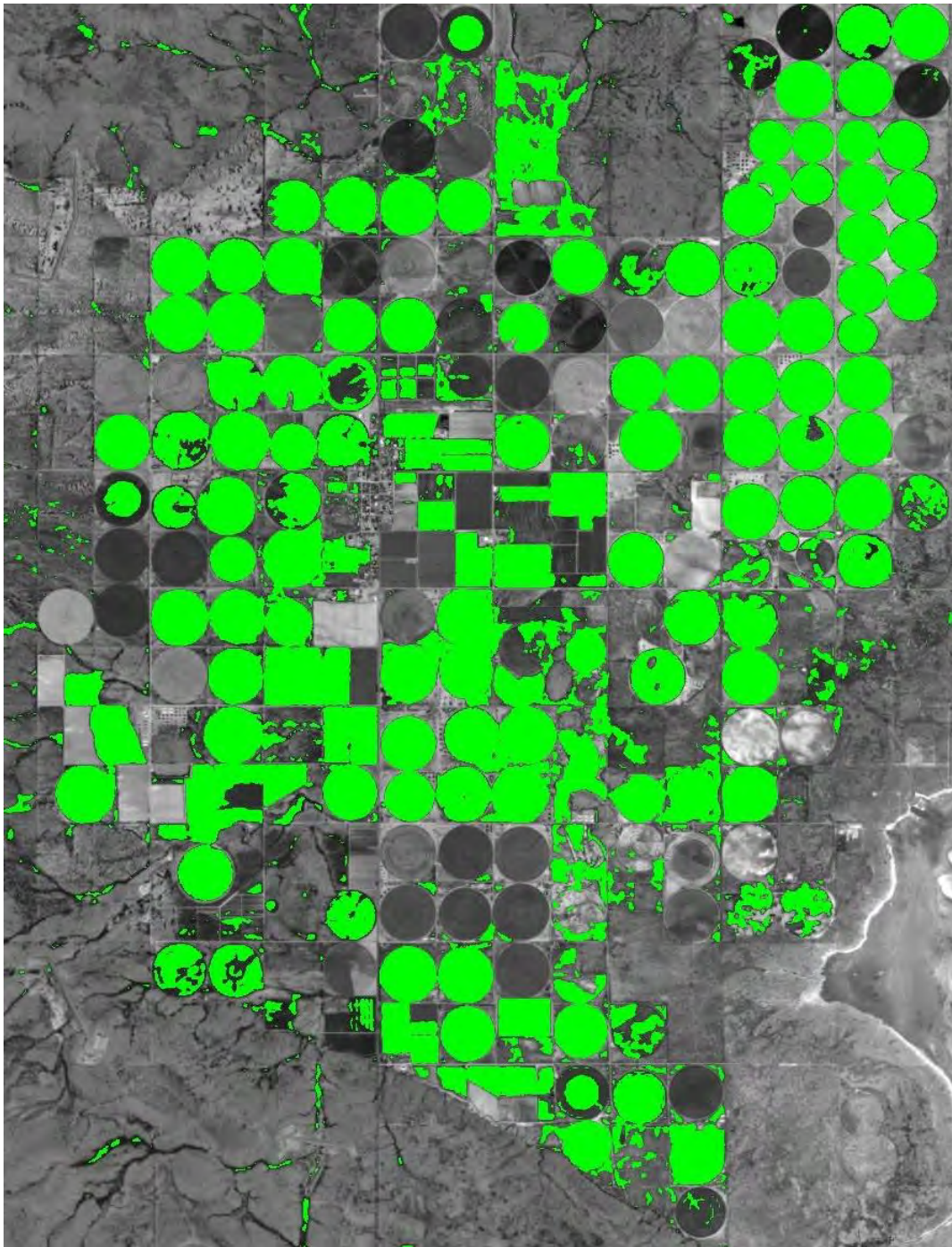
Figure 2-1: Cultivated Acreage in Dell City, Texas, Area in August 2021 from a Landsat 8 Image (Actively growing area shown in green, circular areas are center pivot irrigation systems with approximate diameters of ½ mile)
