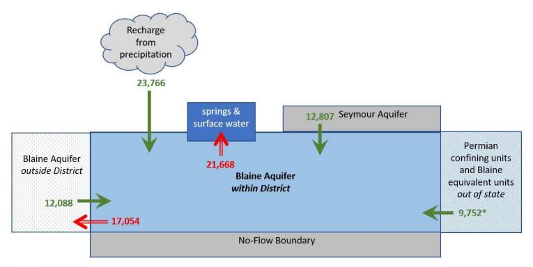
\* Flow from Permian confining units and Blaine equivalent units out of state includes net flow of 13,663 acre-feet per year to Blaine Aquifer from Permian confining units and 3,911 acre-feet per year from Blaine Aquifer to equivalent units in Oklahoma
