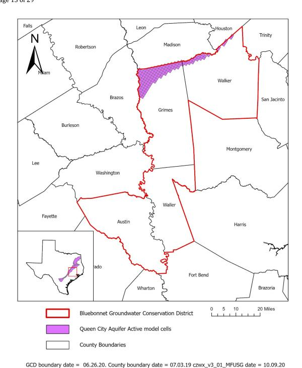
Figure 3: Area of the groundwater availability model for the central portion of the Carrizo-Wilcox, Queen City, and Sparta aquifers from which the information in Table 2 was extracted (the Queen City Aquifer extent within the district boundary).
