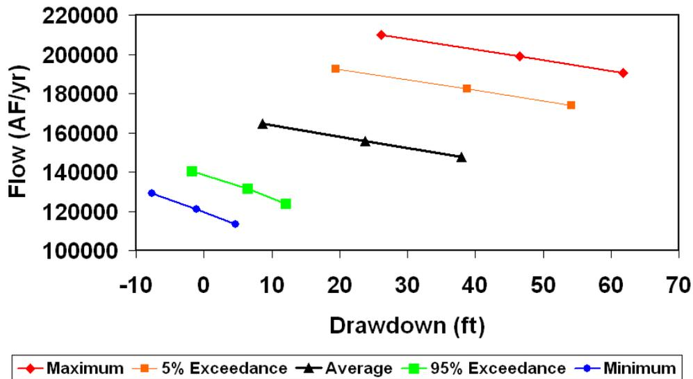
Figure 11. Overall Trinity Aquifer Drawdown in GMA 9 vs. Spring and Base Flow in GMA 9.
