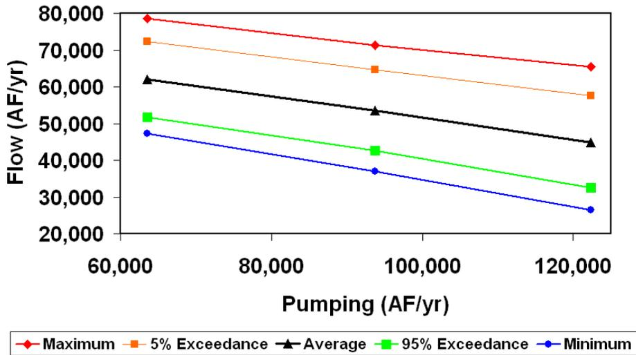
Figure 7. Pumping vs. Outflow across the Balcones Fault Zone for Constant Pumping Scenarios for GMA 9
