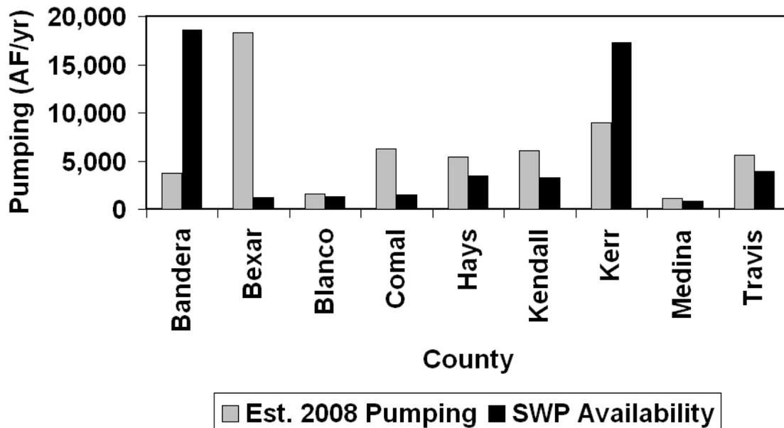
Figure 4. Comparison of 2008 Estimated Pumping and 2007 State Water Plan (SWP) Groundwater Availability in 2060 for the Trinity Aquifer.
