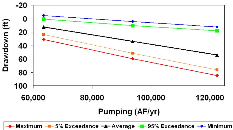
Figure 10. Pumping vs. Drawdown in the Lower Trinity Aquifer for Constant Pumping Scenarios for GMA 9
