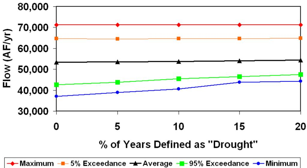
Figure 15. Impact of Definition of Drought and Associated 33% pumping reduction on Outflow across the Balcones Fault Zone in GMA 9.
