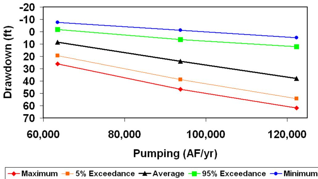
Figure 5. Pumping vs. Overall Trinity Aquifer Drawdown for Constant Pumping Scenarios for GMA 9
