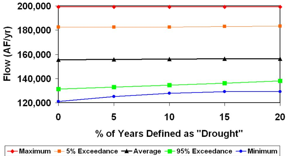
Figure 14. Impact of Definition of Drought and Associated 33% pumping reduction on Spring and Base Flow in GMA 9.
