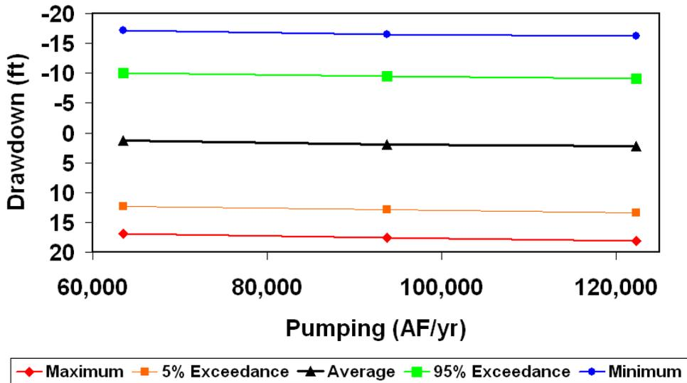
Figure 8. Pumping vs. Drawdown in the Upper Trinity Aquifer for Constant Pumping Scenarios for GMA 9
