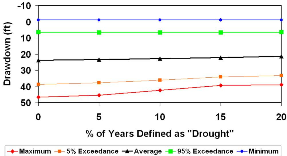
Figure 13. Impact of Definition of Drought and Associated 33% pumping reduction on overall Trinity Aquifer Drawdown in GMA 9.
