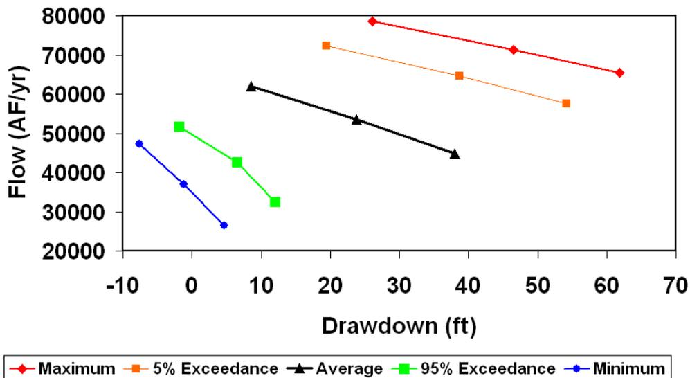
Figure 12. Overall Trinity Aquifer Drawdown in GMA 9 vs. Outflow across the Balcones Fault Zone in GMA 9.
