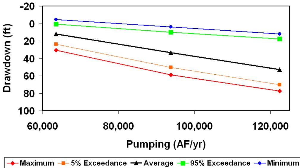
Figure 9. Pumping vs. Drawdown in the Middle Trinity Aquifer for Constant Pumping Scenarios for GMA 9
