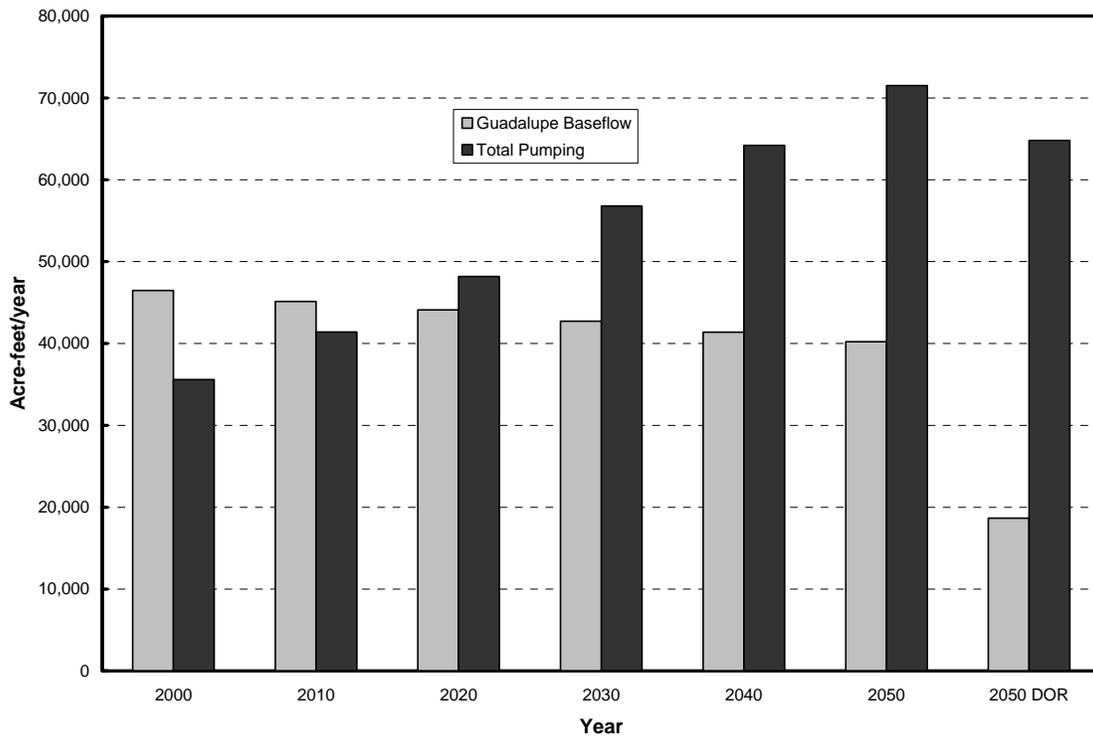
Figure 1. Simulated baseflow to the Guadalupe River and projected total pumping from the Trinity (Hill Country) aquifer for the years 2000, 2010, 2020, 2030, 2040, and 2050 for simulations with and without a drought-of-record. DOR indicates a simulation including a 2044 through 2050 drought-of-record.
