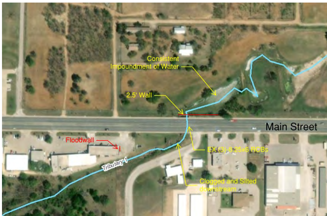
Figure 7-1. CIP 01 Weaver Creek and Main Street Culvert Upsizing, Channel and Grading Improvements
