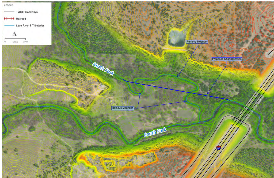
Figure 7-19. FME 07 Proposed Efficiency Improvements to the North Fork
