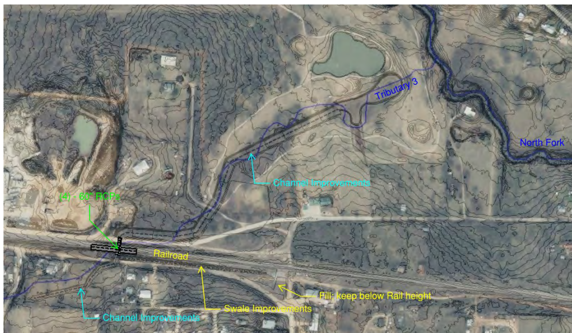
Figure 7-8. CIP 02 Proposed Tributary 3 Culvert and Grading Improvements
