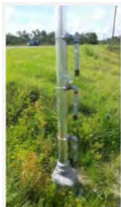
Figure 7-22. Example of a flood sensor.
