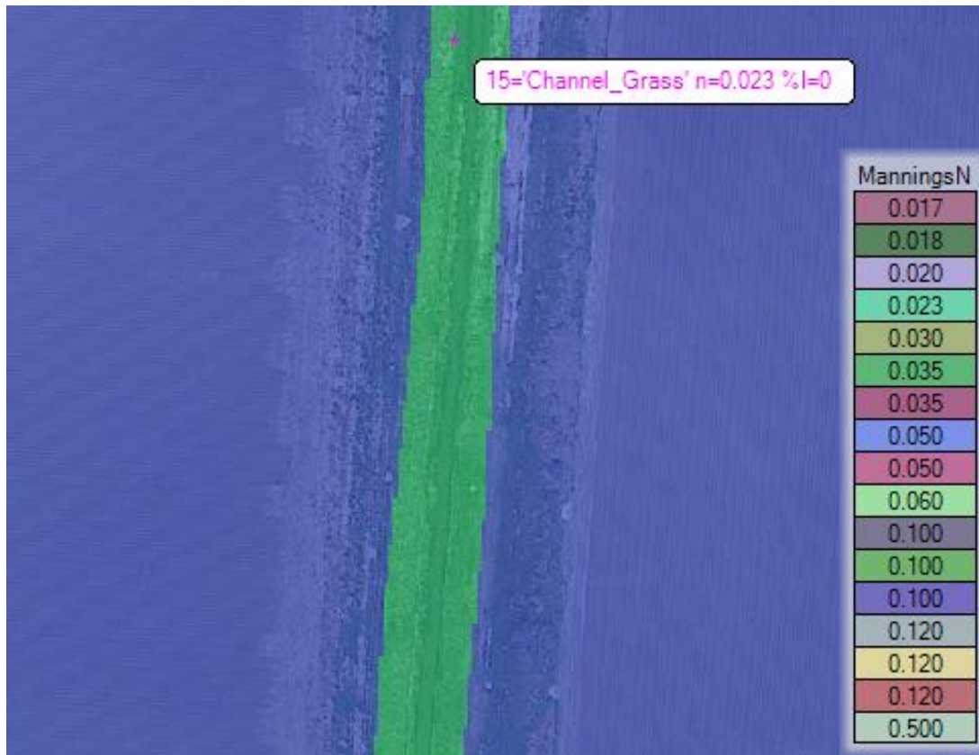
Figure 5.12 Channel Manning's 'n' Classification
