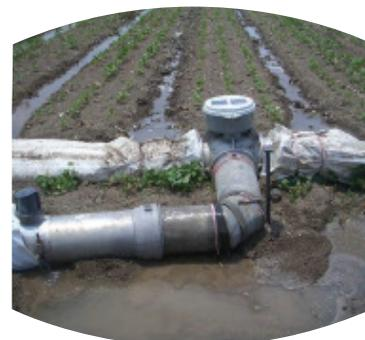
SURGE IRRIGATION IS AN EFFICIENT TECHNOLOGY FOR ACHIEVING OPTIMUM FURROW WATER-VELOCITY.
