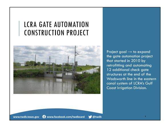
The LCRA Gate Automation project is an example of an active construction project that was granted funding through our program. The goal of this project was to expand the gate automation project that started in 2010 by retrofitting and automating 12 additional check gate structures at the end of the Wadsworth line in the eastern canal system of LCRA's Gulf Coast Irrigation division. This project was awarded grant funds in 2020 and its anticipated completion date is 2028.
