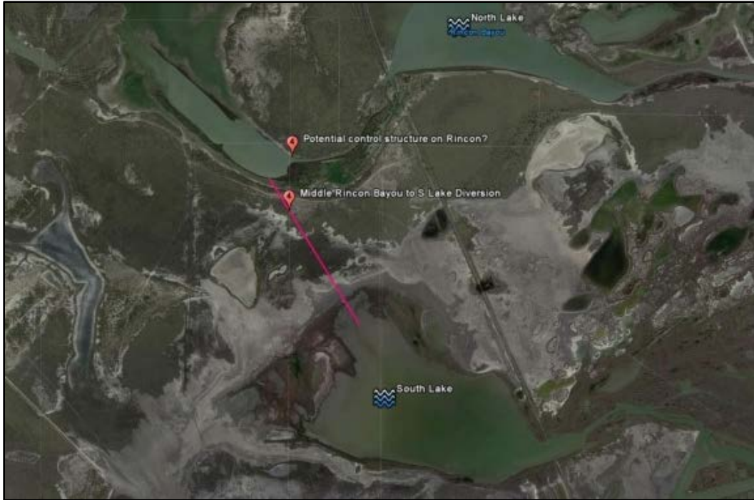
Figure 20. Proposed Diversion from Middle Rincon Bayou to South Lake. From Figure 3.1.1-4: Project #4 – Middle Rincon Bayou Diversion to South Lake Area (Dodson et al., 2016).
