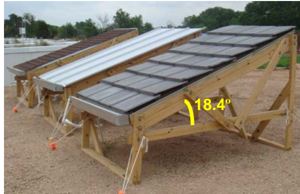
Figure 4-1. Pilot-scale roofs. (From left to right: asphalt fiberglass shingle, Galvalume®, concrete tile)
