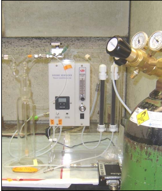
Figure 4-1. Ozone generation and application apparatus.
